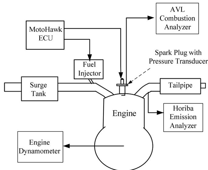
**Fig. 1.** Schematic diagram of engine test.
