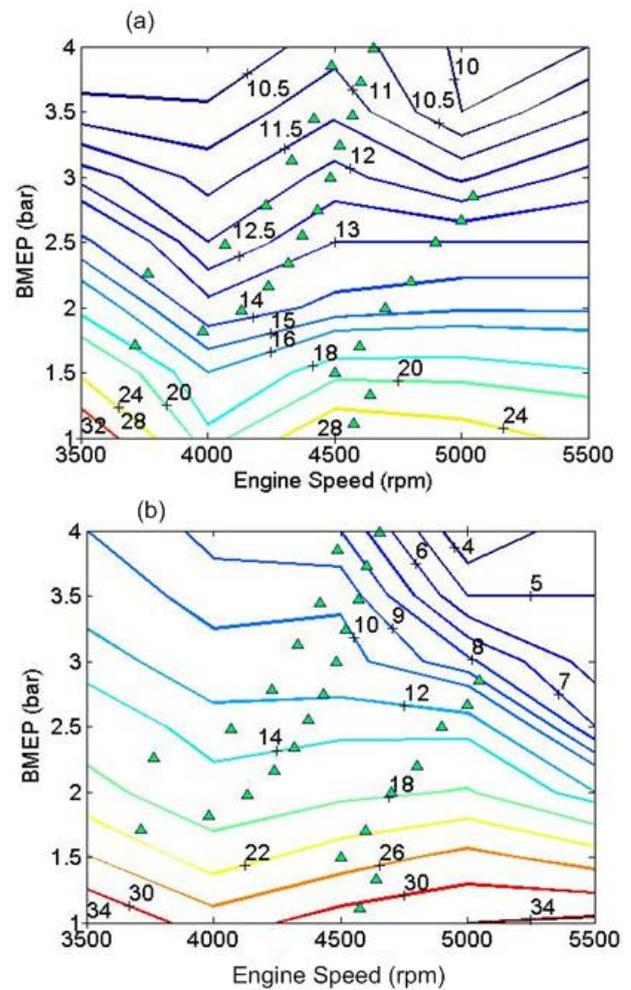
**Fig. 9.** Brake specific hydrocarbon (g/kW.h) maps and ECE-40 operating points (▲) in low-load region: (a) original gasoline engine, (b) SDI engine.
