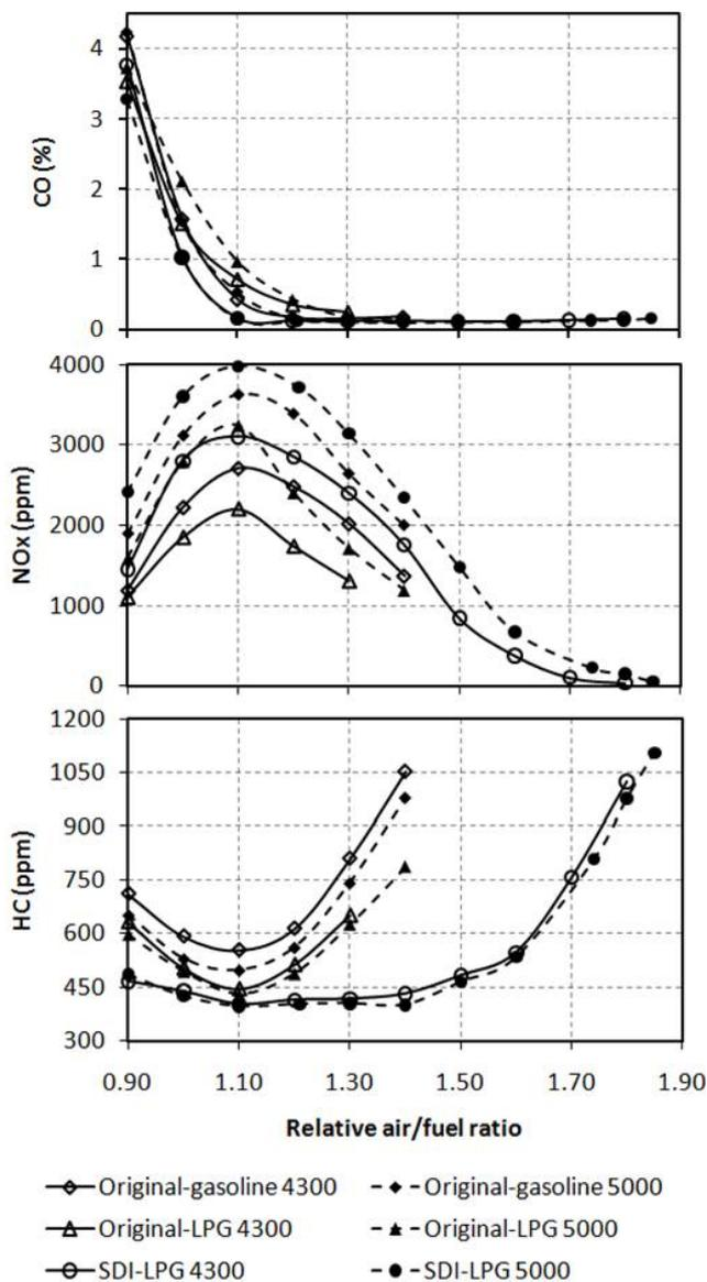
Fig. 5. Effect of relative air/fuel ratio on CO, NO<sub>x</sub> and HC at 4300 and 5000 rpm.
