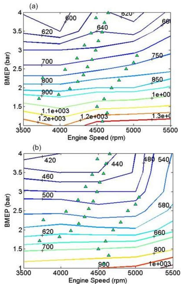
**Fig. 7.** Brake specific carbon dioxide (g/kW.h) maps and ECE-40 operating points ( $\blacktriangle$ ) in low-load region: (a) original gasoline engine, (b) SDI engine.
