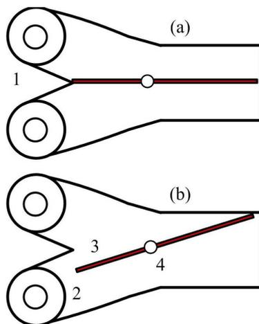
**Fig. 2.** Schematic of intake port: (a) Homogeneous mode, (b) Stratified mode.
