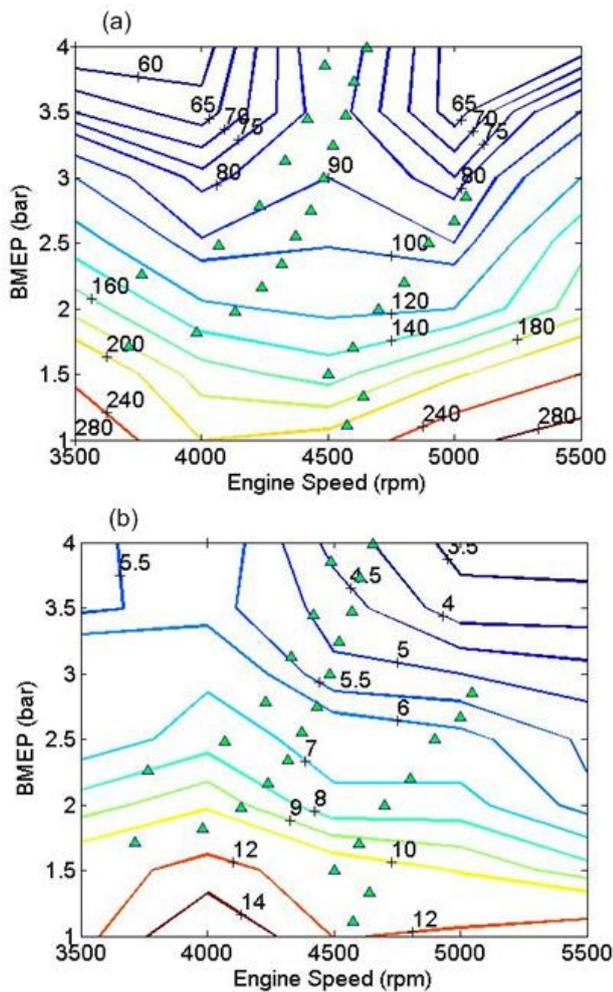
**Fig. 8.** Brake specific carbon monoxide (g/kW.h) maps and ECE-40 operating points (▲) in low-load region: (a) original gasoline engine, (b) SDI engine.
