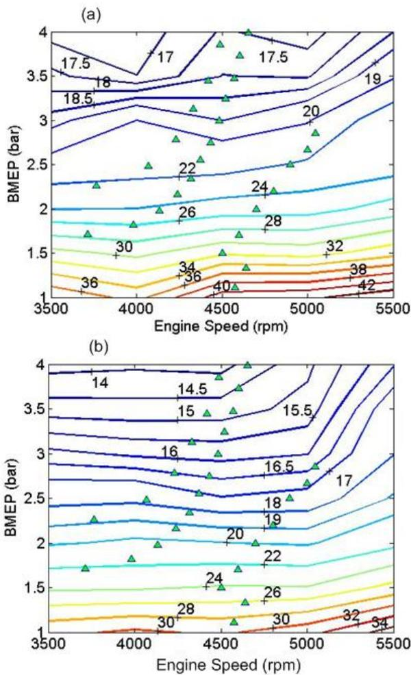
**Fig. 6.** Brake specific energy consumption (MJ/kW.h) maps and ECE-40 operating points ( $\blacktriangle$ ) in low-load region: (a) original gasoline engine, (b) SDI engine.
