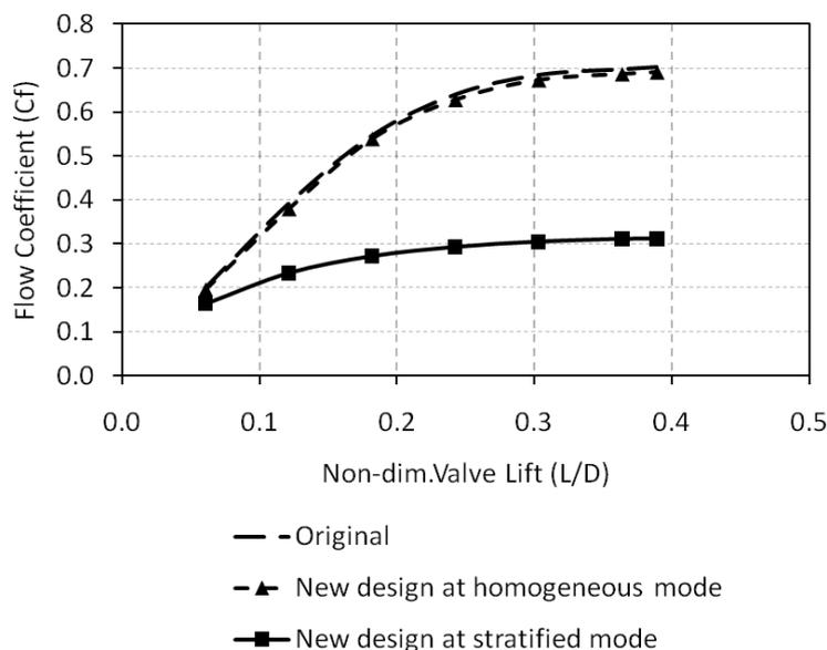
**Fig. 3.** Comparison of flow coefficient of original and new design intake port.
