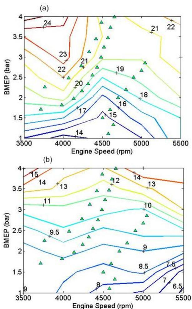
**Fig. 10.** Brake specific oxides nitrogen (g/kW.h) maps and ECE-40 operating points (▲) in low-load region: (a) original gasoline engine, (b) SDI engine.
