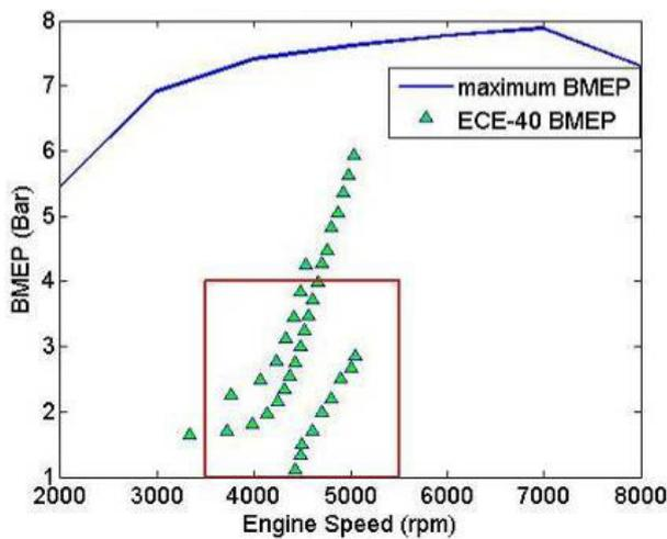
Fig. 4. 125 cc Engine map of ECE-40 cycle.
