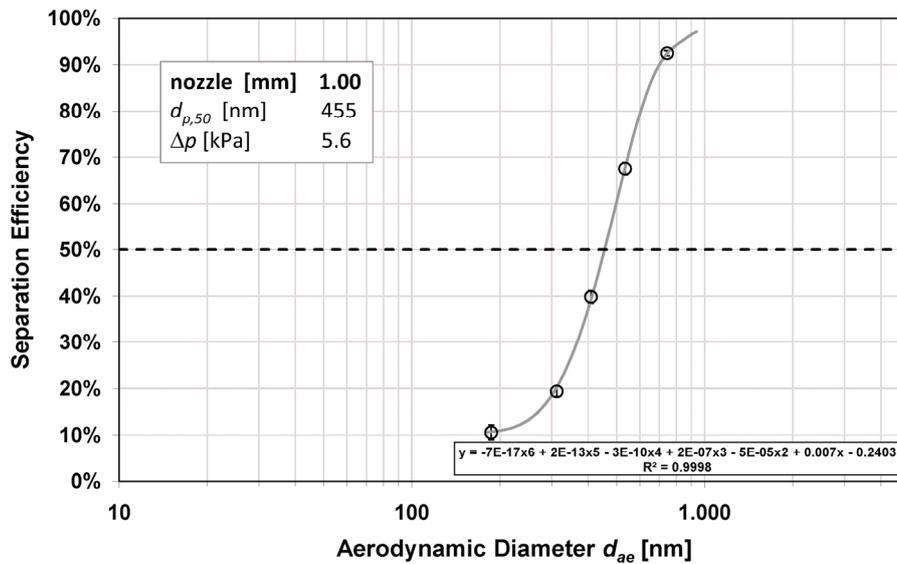
**Fig. 6.** Separation curve of the combination of cyclone with virtual impactor with NIST traceable polystyrene latex particles with 1.5 L/min aerosol flow, 1.0 L/min minor flow and 1.0 mm inlet nozzle.
