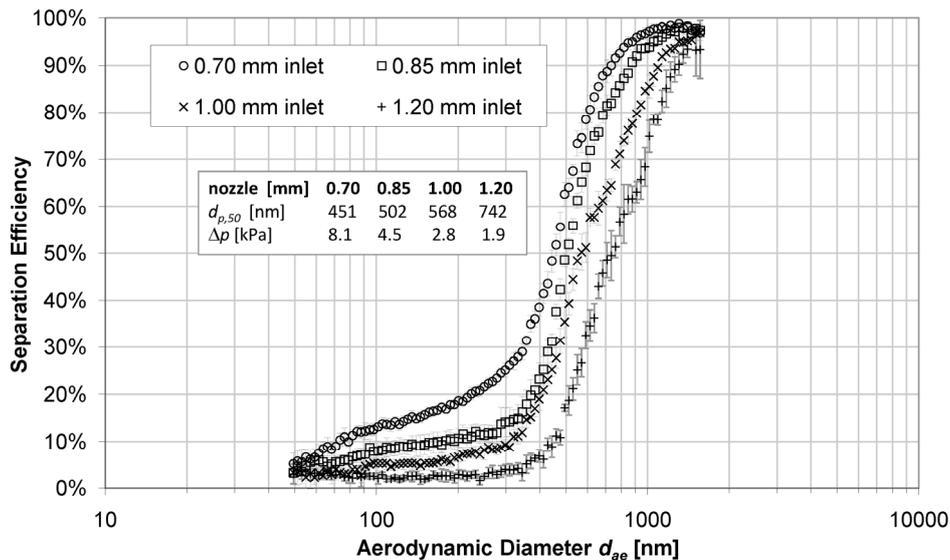
**Fig. 5.** Separation efficiency of preseparator in cyclone mode, i.e. with 1.5 L/min aerosol flow and plugged minor flow outlet; four different inlet nozzle diameters: 0.7 mm, 0.85 mm, 1.0 mm, and 1.2 mm
