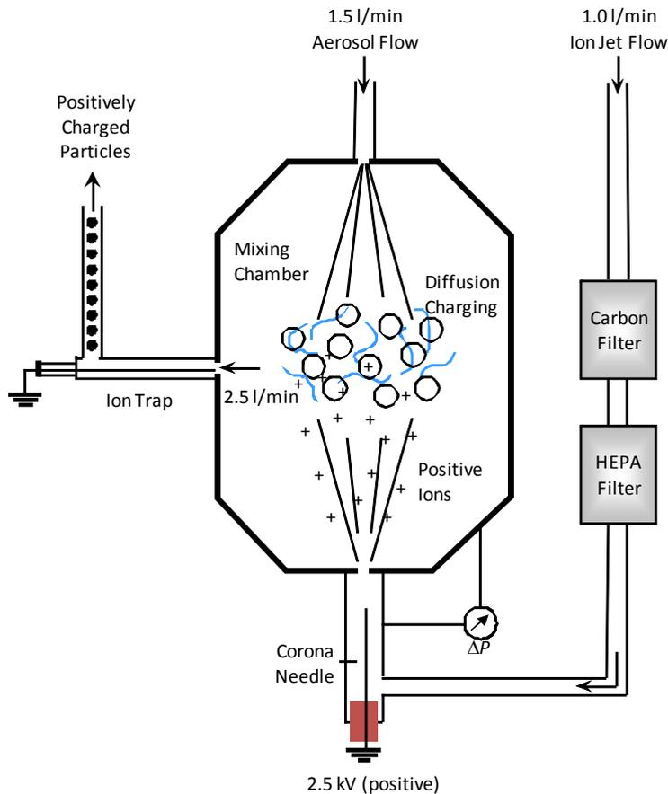
Fig. 2. Schematic of investigated unipolar diffusion charger (Medved et al., 2000).
