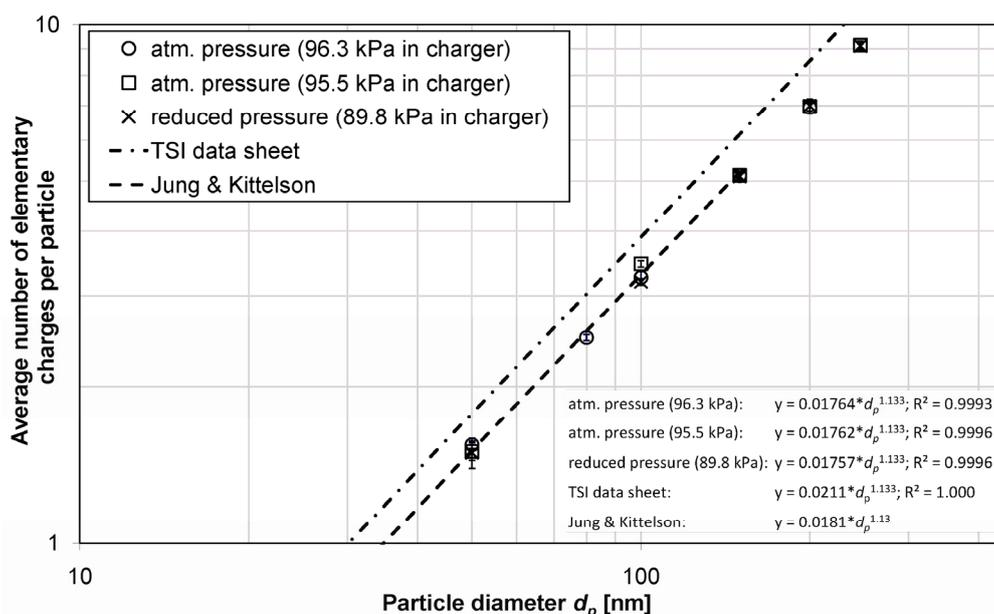
**Fig. 8.** Average number of elementary charges per particle as a function of particle diameter from the present study at atmospheric and reduced pressure, TSI data sheet (2004) and a publication by Jung and Kittelson (2005).
