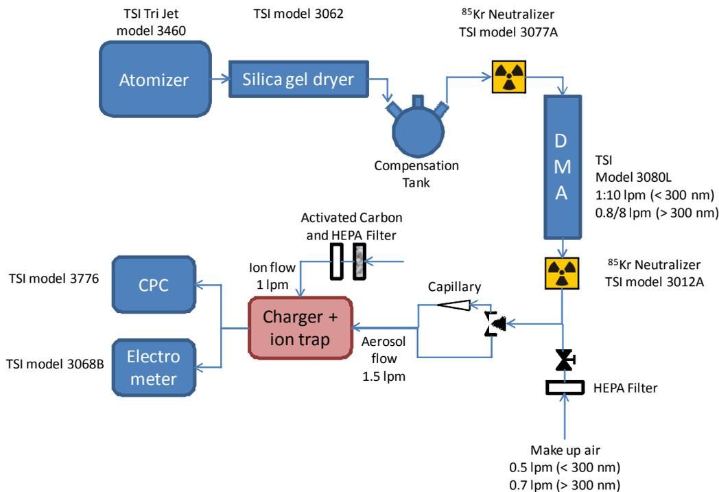
**Fig. 7.** Experimental set up for the measurement of pressure dependent charging efficiency.
