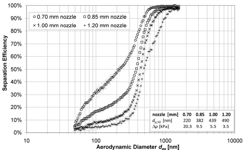
**Fig. 4.** Separation efficiency of preseparator with 1.5 L/min aerosol flow and 1.0 L/min minor flow, i.e. 2.5 L/min total flow with four different inlet nozzle diameters (0.7 mm, 0.85 mm, 1.0 mm, and 1.2 mm).
