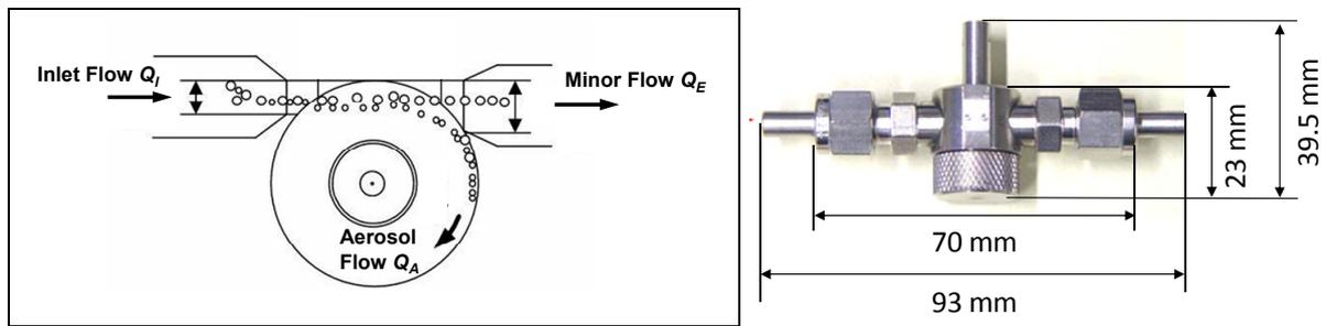
Fig. 1. Schematic and photograph of the preseparator.
