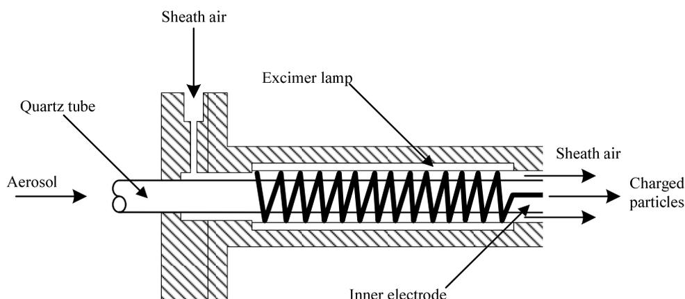
**Fig. 22.** Schematic diagram of the fast photoelectric charger by Graskow (2001).
