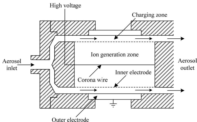
**Fig. 4.** Schematic diagram of the unipolar corona-wire diffusion charger developed by Biskos *et al.* (2005a).
