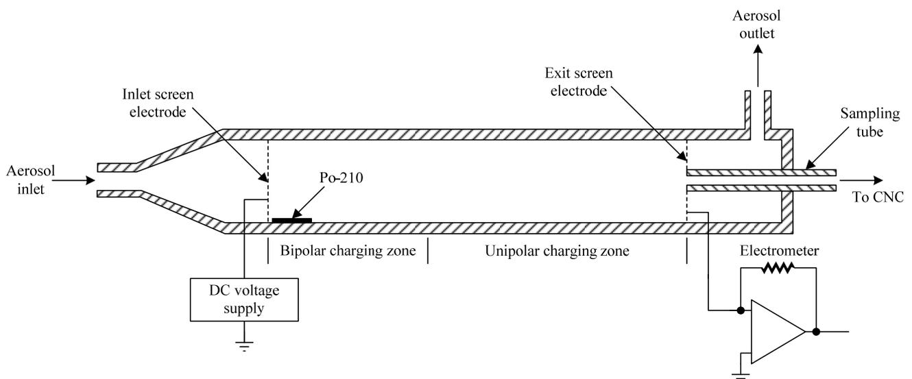
**Fig. 15.** Schematic diagram of the unipolar charger originally developed by Adachi *et al.* (1992).
