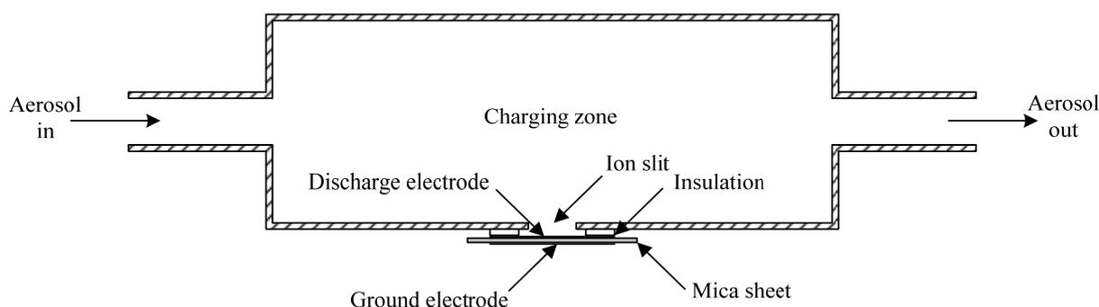
**Fig. 11.** Schematic diagram of the surface-discharge microplasma aerosol charger (SMAC) (Kwon *et al.*, 2007).
