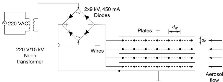
**Fig. 2.** Diagram of the direct current high-voltage circuit.
