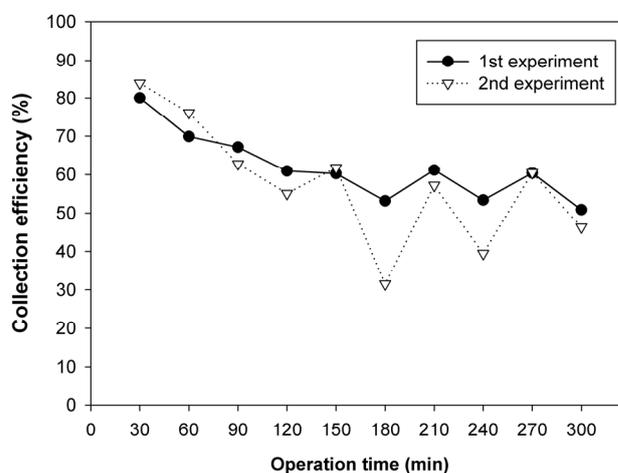
Fig. 9. Collection efficiency of the ESP equipped with a cleaning system.
