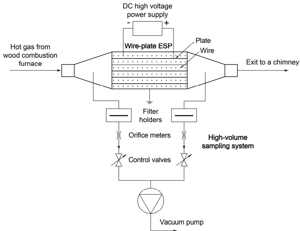
**Fig. 4.** Diagram of the gas sampling equipment.
