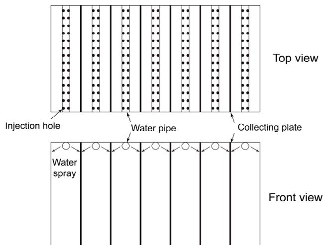
Fig. 8. Diagram of cleaning system of the ESP.
