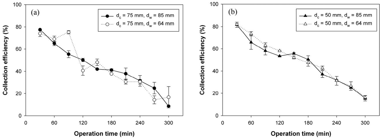
**Fig. 5.** Collection efficiency of the ESP for constant gap between collection plate electrodes ( $d_c$ ) and variable distance between wire electrodes ( $d_w$ ) (a)  $d_c = 75$  mm,  $d_w = 85$ , and 64 mm. (b)  $d_c = 50$  mm,  $d_w = 85$  and 64 mm.
