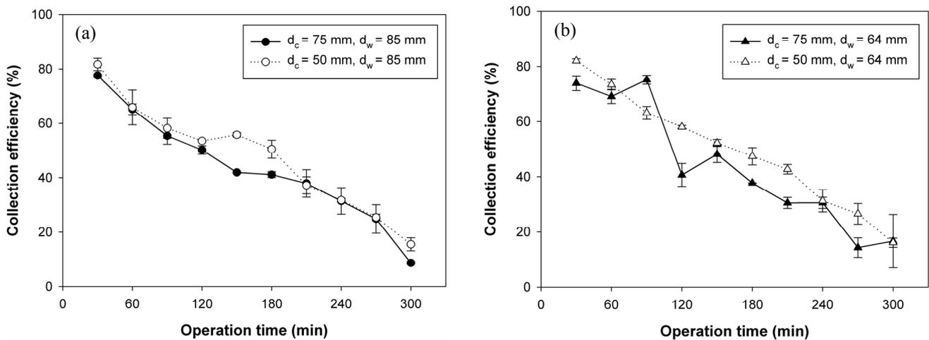
**Fig. 6.** Collection efficiency of the ESP for constant distance between wire electrodes ( $d_w$ ) and variable gap between collection plate electrodes ( $d_c$ ) (a)  $d_w = 85$  mm,  $d_c = 50$  and 75 mm. (b)  $d_w = 64$  mm,  $d_c = 50$ , and 75 mm.
