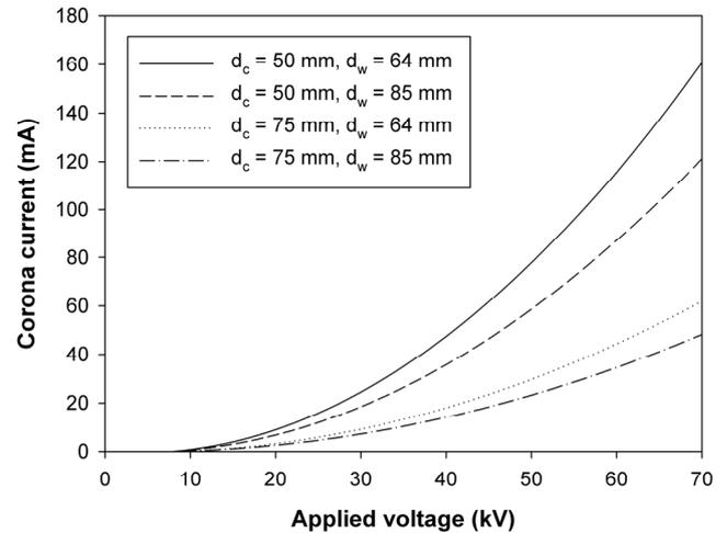
**Fig. 3.** Current-voltage prediction of the designed electrostatic precipitator.**Table 3.** Prediction of the numbers of charges and corona onset values from the designed ESP.
