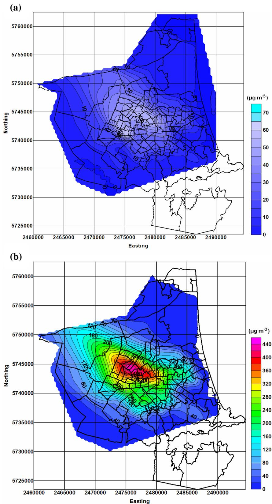
**Fig. 4.** Spatial near-surface (8-10 metres) distribution of  $\text{PM}_{10}$  concentrations ( $\mu\text{g m}^{-3}$ ) at midnight 5 May 2005: (a) for the winter 2010 proposed 70% reduction of total emissions; (b) for the initial winter 1999 “Total” group emissions.
