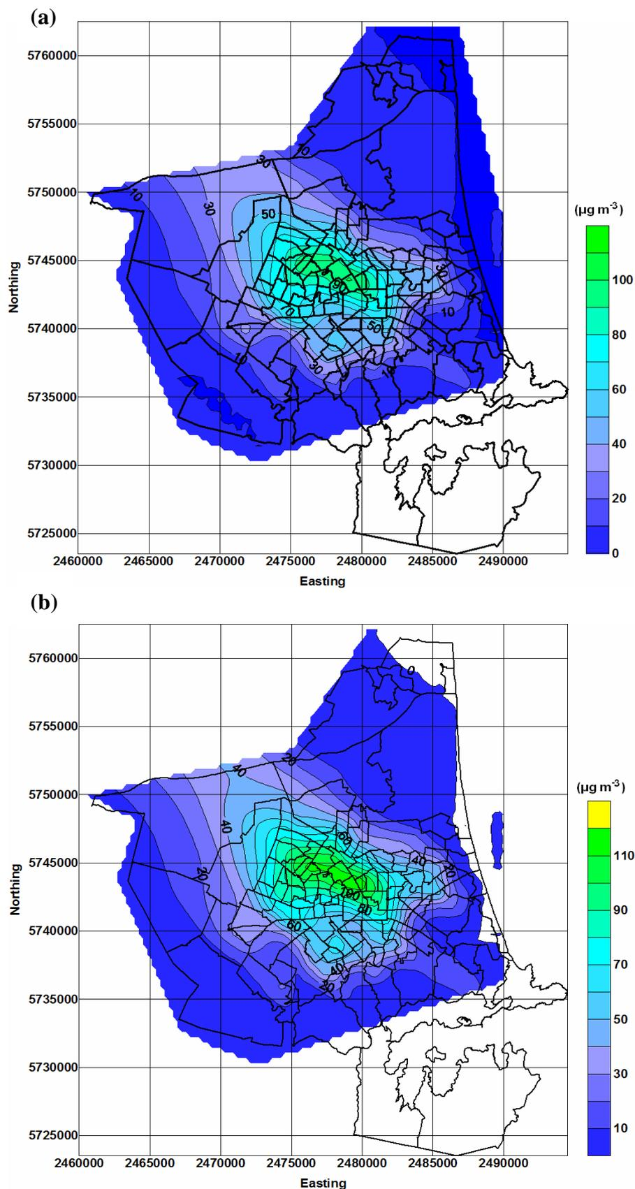
**Fig. 3.** Spatial distribution of "Total" PM<sub>10</sub> ( $\mu\text{g m}^{-3}$ ) at 11 pm 4 May 2005 using the optimal chemical scenario: (a) ("Domestic + Transport")/2 – linear; (b) ("Domestic + Transport")/2 – non-linear.
