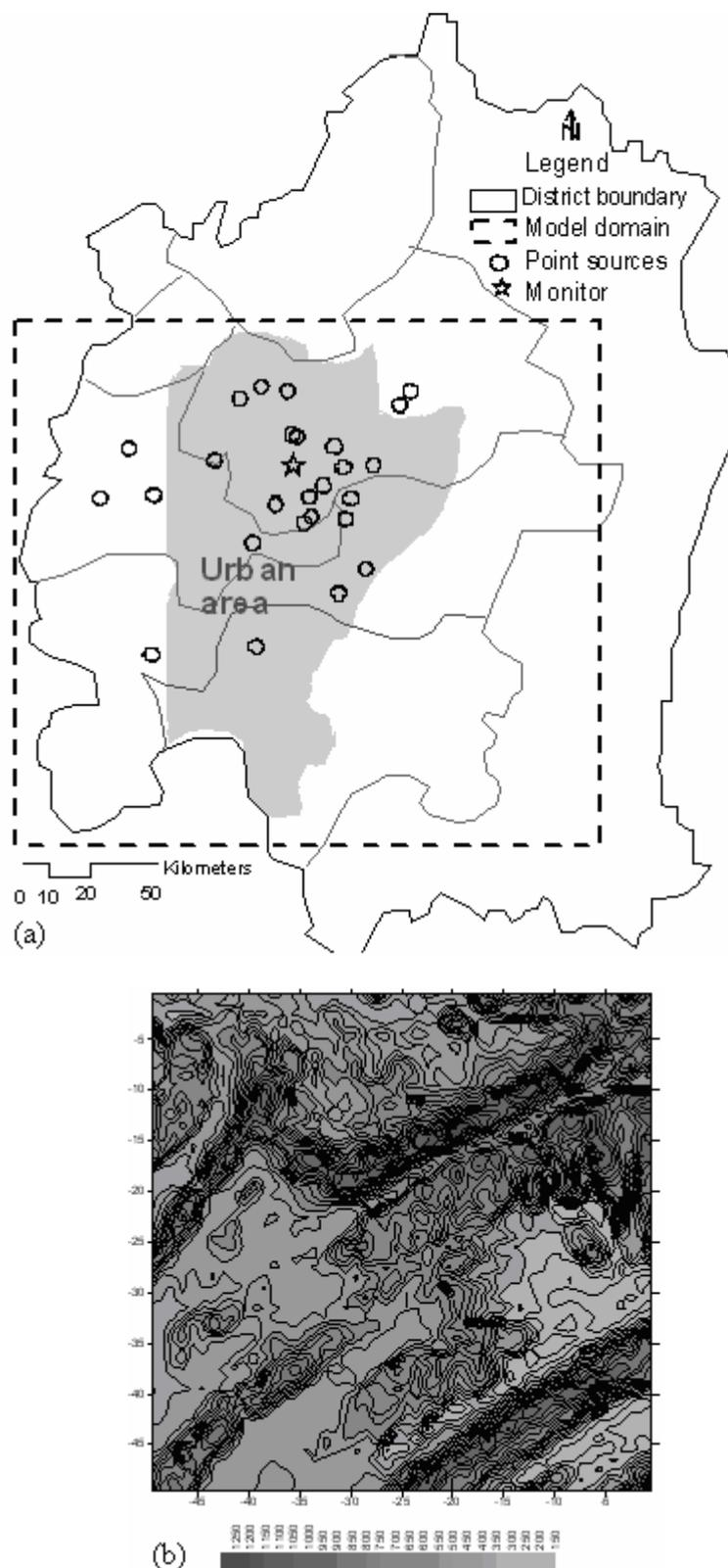
**Fig. 1.** (a) Domain coverage and locations of elevated point sources; (b) terrain characteristics (m) in Chongqing. Area in gray color is the urban area of Chongqing. Also shown is the location of the monitor site (open star).
