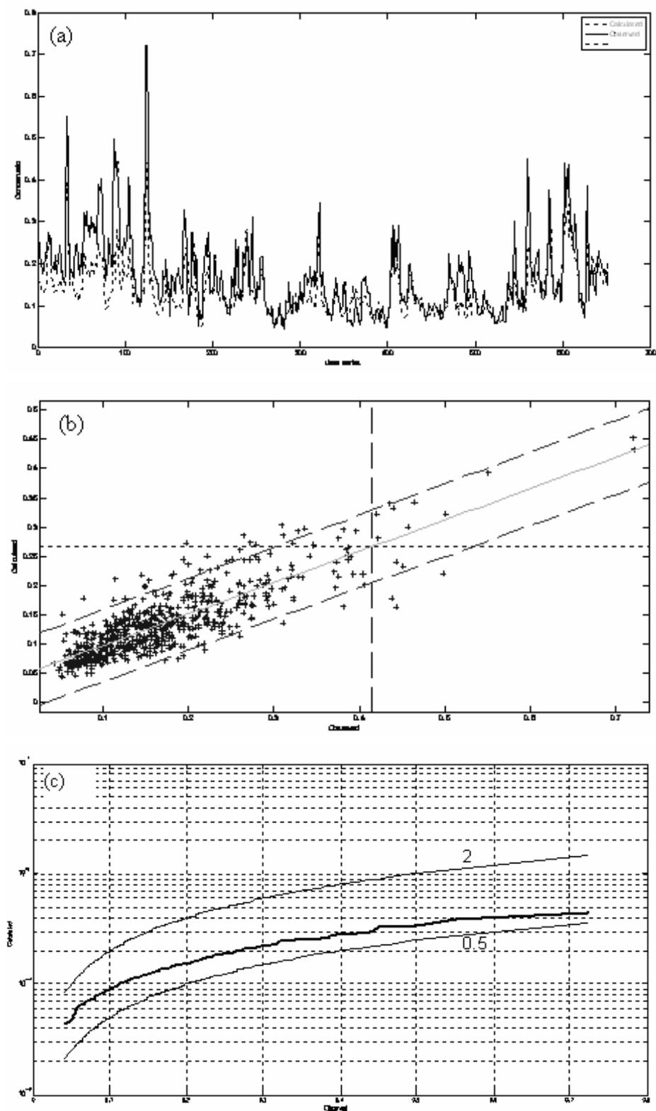
**Fig. 5.** (a) Time series of CALPUFF predicted (dot line) and observed  $\text{SO}_2$  concentrations (solid line) at the monitor from 1 to 31, January, 2004 ( $\text{mg}/\text{m}^3$ ); (b) Scatter plots of modeled versus observed concentrations ( $\text{mg}/\text{m}^3$ ); (c) Quantile-quantile plots of modeled versus observed concentrations ( $\text{mg}/\text{m}^3$ ).
