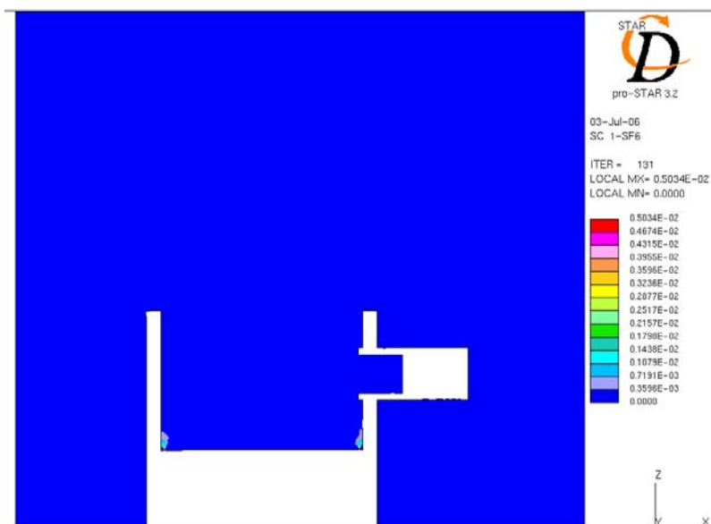
Fig. 7. Concentration field around the chamber and at the breathing zone for SF 6 release flow rate of 10 L/min, venting flow rate of 3130 L/min (Case 1).
