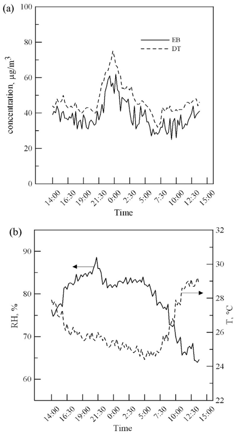
**Fig. 2.** (a) PM<sub>2.5</sub> reading vs. time (b) Relative humidity and temperature vs. time (EB without heating).
