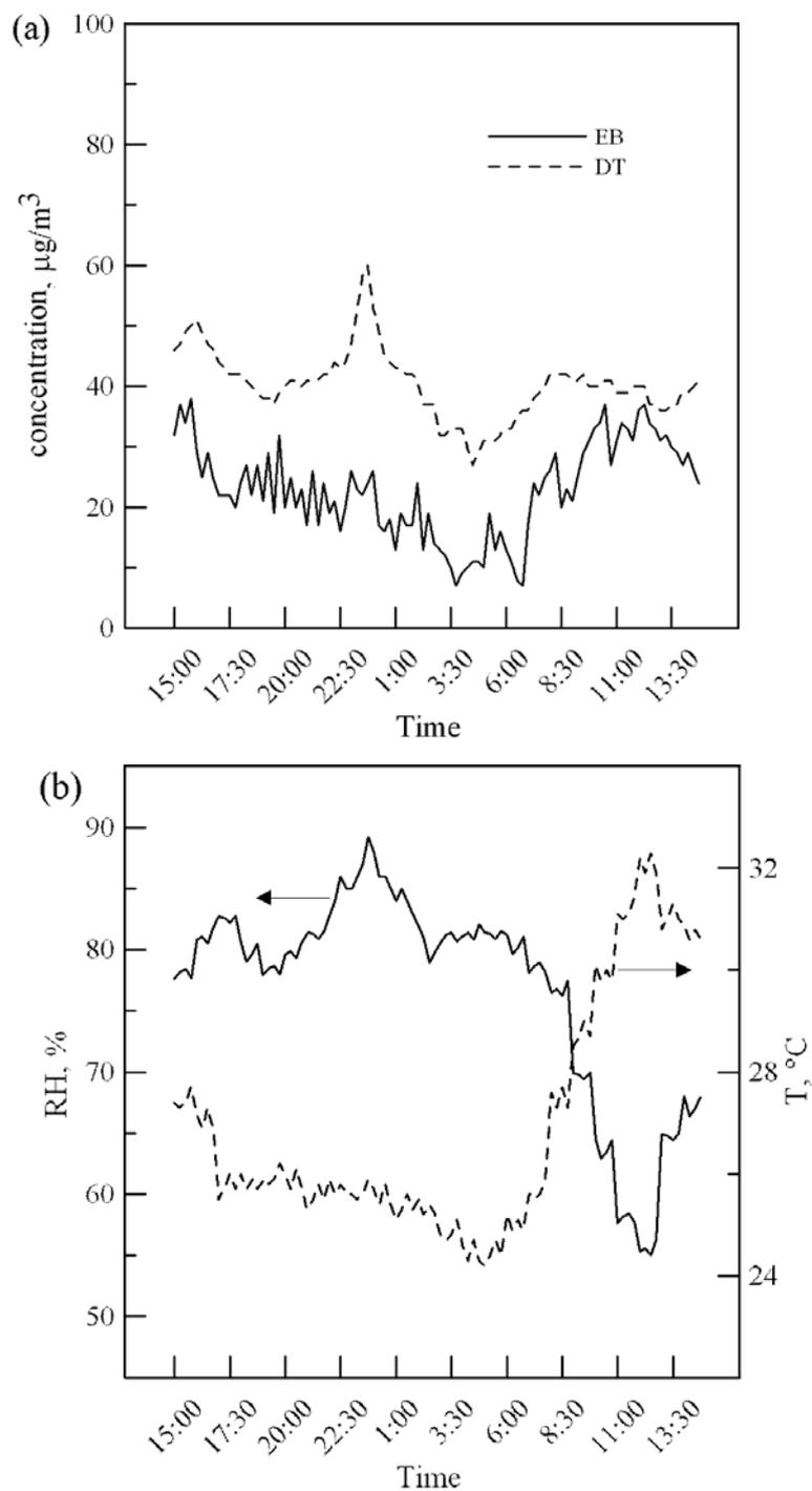
**Fig. 5.** (a) PM<sub>2.5</sub> reading vs. time (b) Relative humidity and temperature vs. time (EB with heating).
