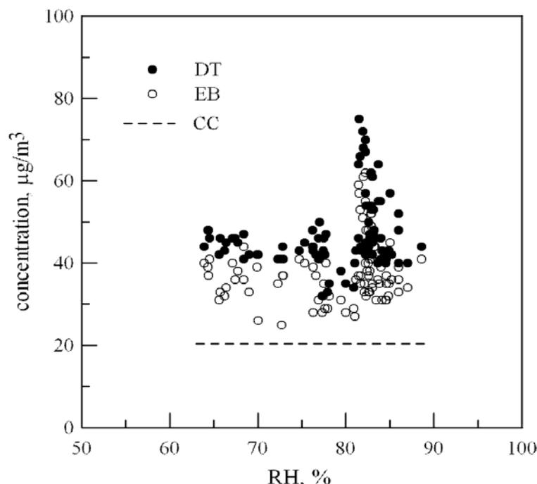
**Fig. 3.** PM<sub>2.5</sub> reading of DT, CC and EB without heating at various relative humidities.
