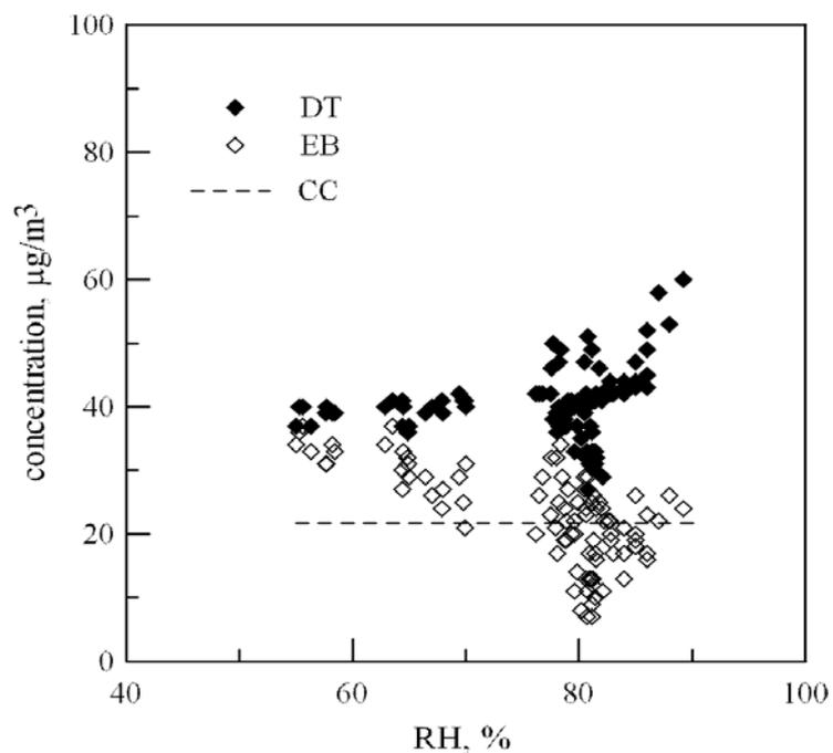
**Fig. 6.** PM<sub>2.5</sub> reading of DT, CC and EB with heating at various relative humidities.
