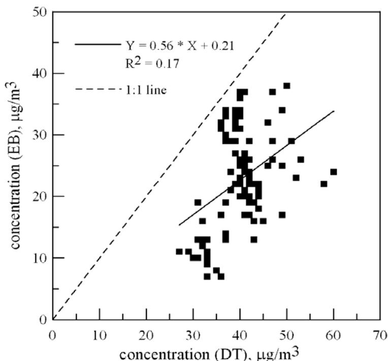
**Fig. 4.** Comparison of PM<sub>2.5</sub> readings between DT and EB with heating.
