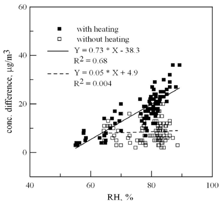
**Fig. 7.** Influence of relative humidity on PM<sub>2.5</sub> difference between DT and EB.
