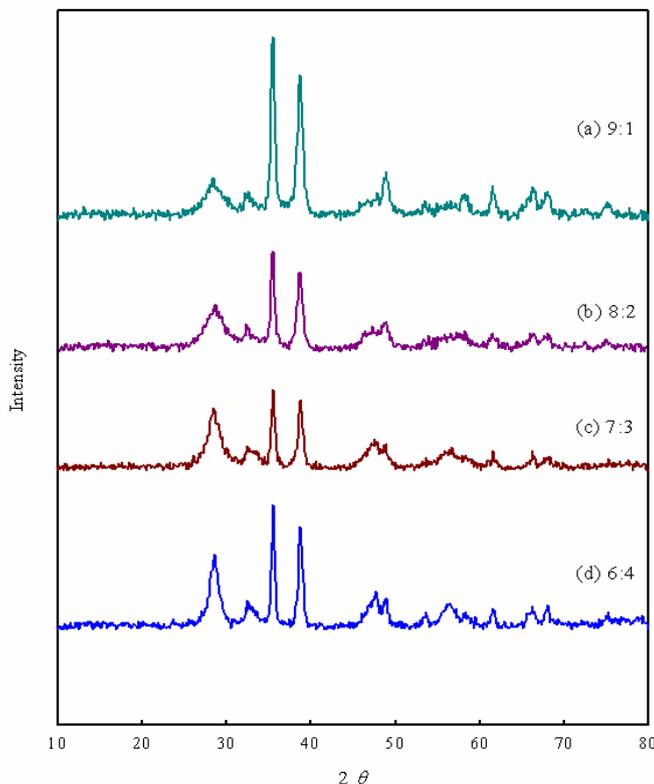
**Fig. 2.** XRD pattern of the various metal content on the CuO-CeO<sub>2</sub> bimetallic oxide catalyst for the conversion of NH<sub>3</sub>.
