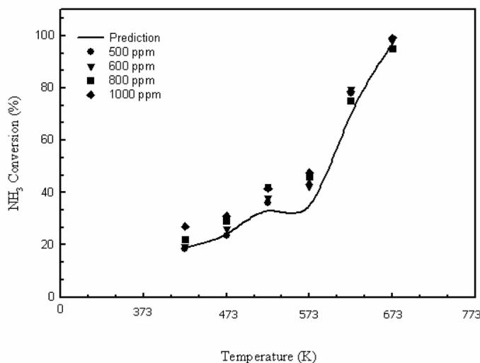
**Fig. 11.** Comparison of experimental data (symbols) and computed values (solid lines) from conversions of the rate equation at different temperatures and different concentrations of  $\text{NH}_3$  by integral type model. Test conditions: 500-1,000 ppm  $\text{NH}_3$  in He, Temp.=423-673 K,  $\text{O}_2=4\%$ , R.H.=12%, GHSV=92,000 ml/h-g.
