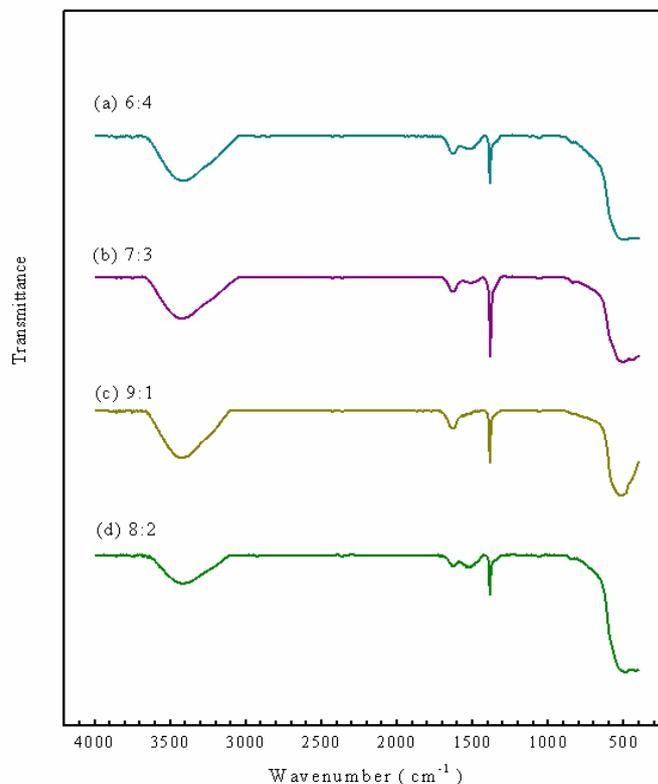
**Fig. 3.** FTIR pattern of the various metal content on the CuO-CeO<sub>2</sub> bimetallic oxide catalyst for the conversion of NH<sub>3</sub>.
