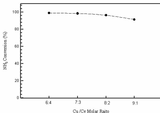
**Fig. 5.** Effect of the metal content on the CuO-CeO<sub>2</sub> bimetallic oxide catalyst for the conversion of NH<sub>3</sub>. Test conditions: 1,000 ppm NH<sub>3</sub> in He, O<sub>2</sub>=4%, temperature= 673 K, R.H.=12%, GHSV=92,000 ml/h-g.
