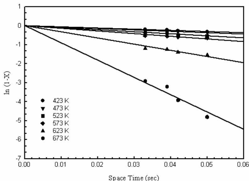
**Fig. 9.** Effect of the space time with the fractional conversion ( $X$ ) on the CuO-CeO<sub>2</sub> (6:4) bimetallic oxide catalyst for the conversion of NH<sub>3</sub>. Test conditions: 1,000 ppm NH<sub>3</sub> in He, O<sub>2</sub>=4%, R.H.=12%, GHSV=92,000 ml/h-g.
