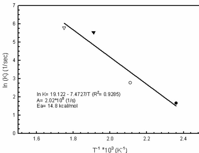
**Fig. 10.** Arrhenius plots of rate constants on the CuO-CeO<sub>2</sub> (6:4) bimetallic oxide catalyst for the conversion of NH<sub>3</sub>.
