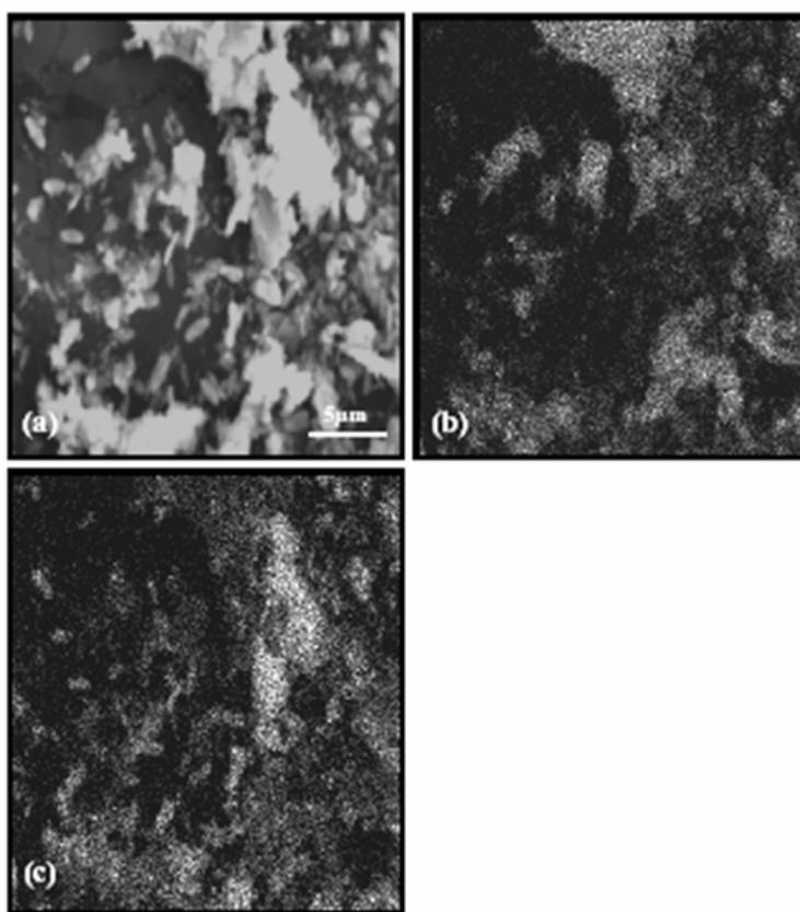
**Fig. 7.** SEM with dot mapping photographs result of various contents on the fresh  $\text{CuO-CeO}_2$  (6:4) bimetallic oxide catalyst after activity test. (a) Original magnification:  $\times 3,000$ , (b) Cu and (c) Ce. Test conditions : 1,000 ppm  $\text{NH}_3$  in He,  $\text{O}_2=4\%$ , R.H.=12%, GHSV=92,000 ml/h-g.
