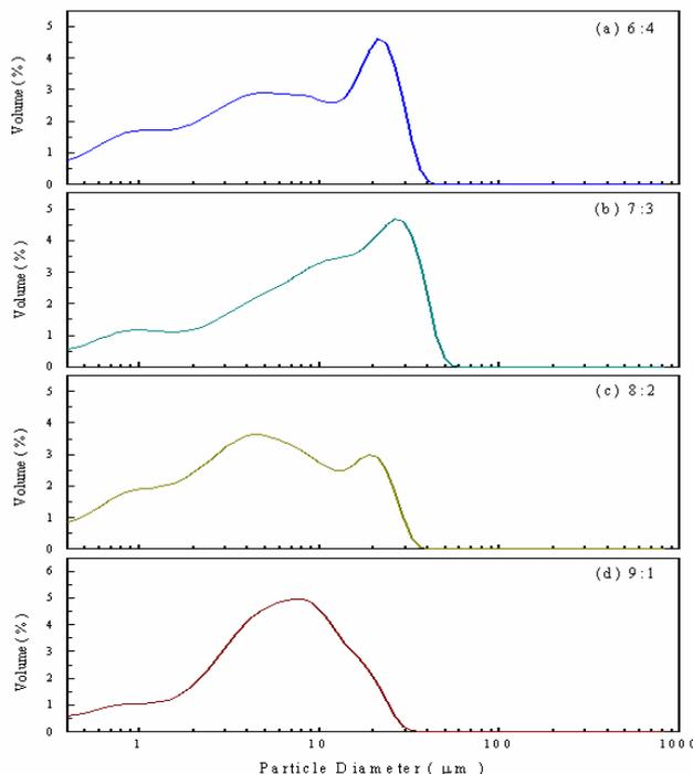
**Fig. 4.** Changes in particle sizes distribution of the various metal content on the CuO-CeO<sub>2</sub> bimetallic oxide catalyst for the conversion of NH<sub>3</sub>.
