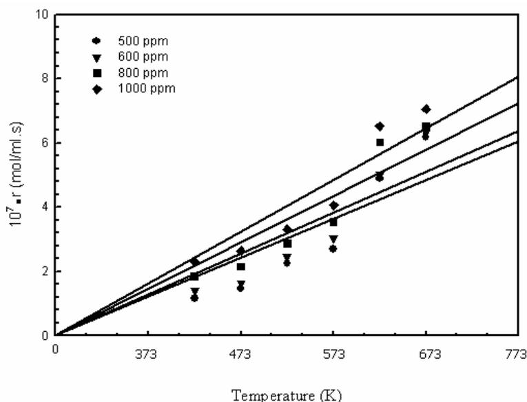
**Fig. 8.** Effect of various ammonia concentrations and different temperatures with reaction rates on the  $\text{CuO-CeO}_2$  (6:4) bimetallic oxide catalyst for the conversion of  $\text{NH}_3$ . Test conditions: 500-1,000 ppm  $\text{NH}_3$  in He,  $\text{O}_2=4\%$ , R.H.=12%, GHSV=92,000 ml/h-g.
