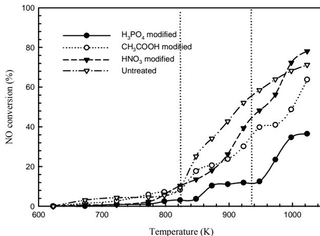
**Figure 6.** Effect of treatment with different a fixed concentration (2M) of various inorganic acids on the 8 wt.% Cu/ $\gamma$ -Al<sub>2</sub>O<sub>3</sub> catalyst for the conversion of NO with CH<sub>4</sub>. Test conditions : 1000 ppm NO in He, 1000 ppm CH<sub>4</sub> in He, O<sub>2</sub> = 2%, GHSV = 108000 ml/h-g.
