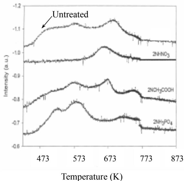
**Figure 8.** TPD of triethylamine profiles of 8 wt.% Cu/ $\gamma$ -Al<sub>2</sub>O<sub>3</sub> catalysts that are untreated or treated with various inorganic acids.
