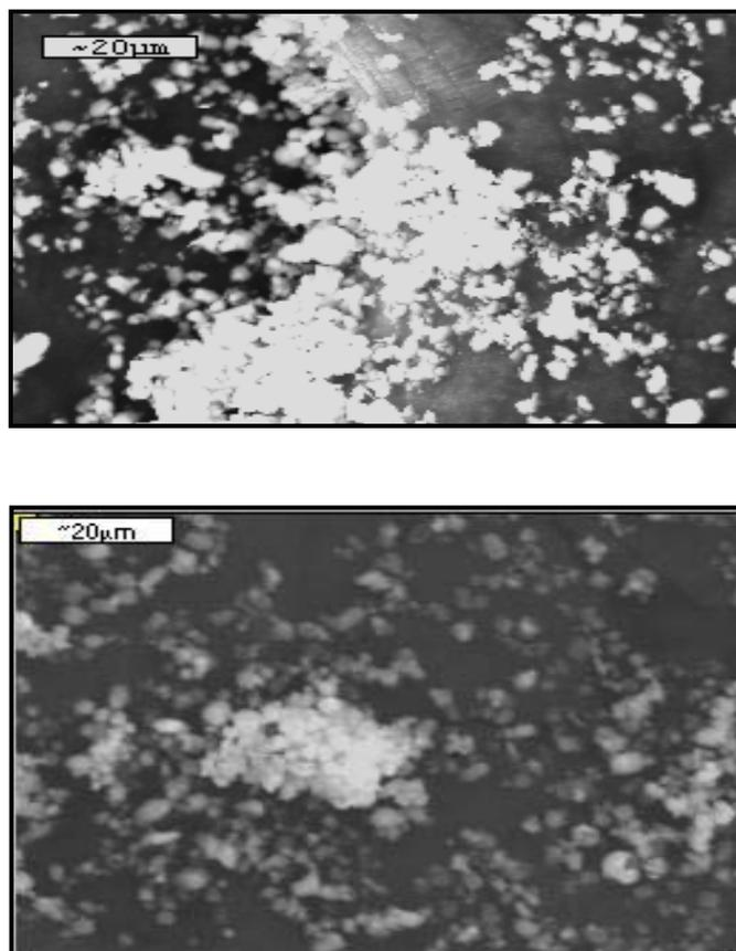
**Figure 10.** SEM photograph of the outward appearance of dispersed metal white point of 8 wt.%  $\text{Cu}/\gamma\text{-Al}_2\text{O}_3$  catalyst that is (a) untreated and (b) that is treated with 6 M nitric acid.
