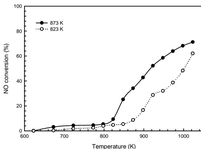
**Figure 3.** Effect of calcinations temperature on the 8 wt.% Cu/ $\gamma$ -Al<sub>2</sub>O<sub>3</sub> catalyst for the conversion of NO with CH<sub>4</sub>. Test conditions : 1000 ppm NO in He, 1000 ppm CH<sub>4</sub> in He, O<sub>2</sub> = 2%, GHSV = 108000 ml/h-g.
