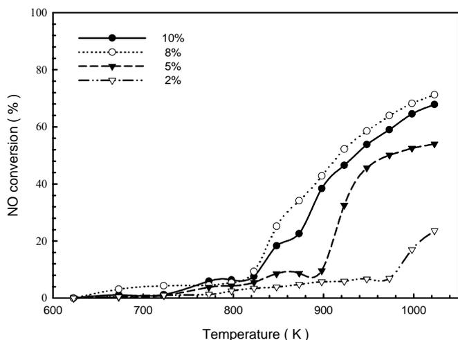
**Figure 2.** Effect of copper loading on the Cu/ $\gamma$ -Al<sub>2</sub>O<sub>3</sub> catalyst for the conversion of NO with CH<sub>4</sub>. Test conditions : 1000 ppm NO in He, 1000 ppm CH<sub>4</sub> in He, O<sub>2</sub> = 2%, GHSV = 108000 ml/h-g.
