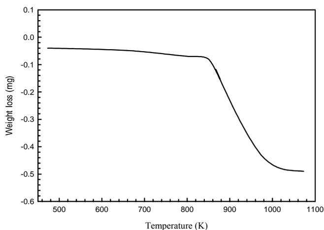
**Figure 4.** Thermal gravimetric analysis (TGA) diagram of 8 wt.% Cu/ $\gamma$ -Al<sub>2</sub>O<sub>3</sub> catalyst for the conversion of NO with CH<sub>4</sub>. Test conditions : Sample weight = 25 mg, heating rate = 283 K/min in nitrogen flow.
