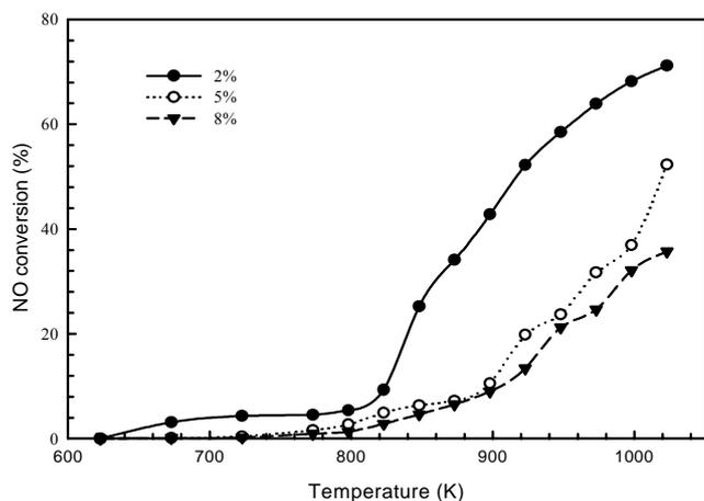
**Figure 5.** Effect of oxygen concentrations on the 8 wt.% Cu/ $\gamma$ -Al<sub>2</sub>O<sub>3</sub> catalyst for the conversion of NO with CH<sub>4</sub>. Test conditions : 1000 ppm NO in He, 1000 ppm CH<sub>4</sub> in He, O<sub>2</sub> = 2%-8%, GHSV = 108000 ml/h-g.
