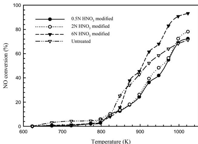
**Figure 7.** Effect of treatment with various concentrations of nitric acid on the 8 wt.% Cu/ $\gamma$ -Al<sub>2</sub>O<sub>3</sub> catalyst for the conversion of NO with CH<sub>4</sub>. Test conditions : 1000 ppm NO in He, 1000 ppm CH<sub>4</sub> in He, O<sub>2</sub> = 2%, GHSV = 108000 ml/h-g.
