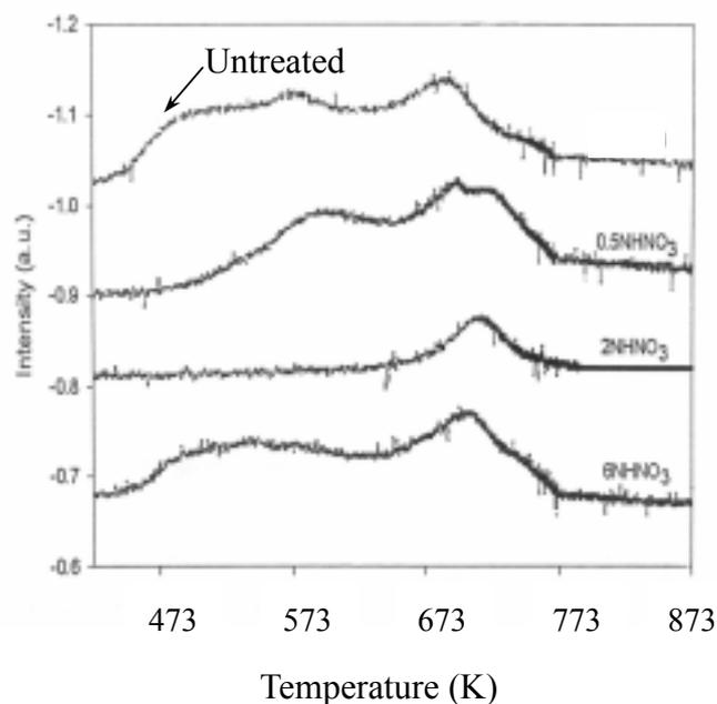
**Figure 9.** TPD of triethylamine profiles of 8 wt.% Cu/ $\gamma$ -Al<sub>2</sub>O<sub>3</sub> catalysts that are untreated or treated with various concentration of nitric acid.
