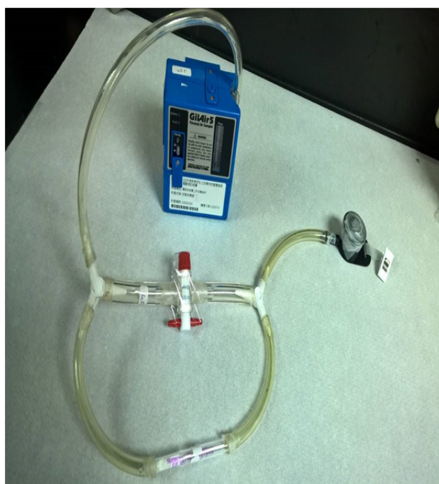
Fig. 1. The sampling train of gaseous and particulate phase PAHs.
