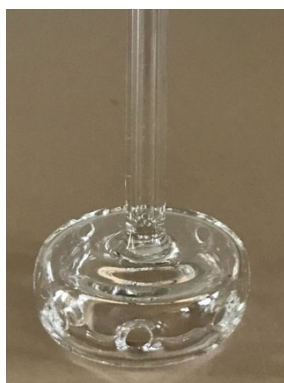
Figure 1S: filter-holder used during the kinetic/solubility measurements.
