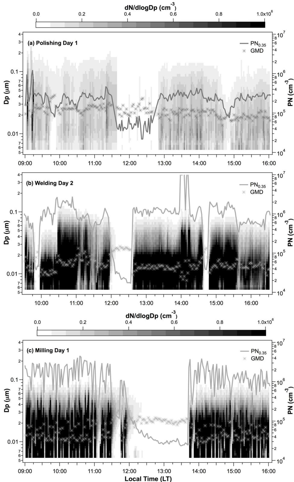
**Fig. 6.** Examples of the measured ambient particle number size distributions, total particle number concentrations ( $PN_{0.35}$ ) and geometric mean diameters (GMD) during metal (a) polishing, (b) welding and (c) milling.
