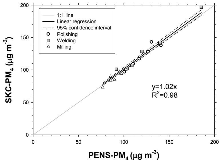
**Fig. 4.** Scatterplot and regression of respirable particle mass concentrations ( $PM_4$ ) measured by the paired PENS/SKC personal samplers at the three metalworking plants.
