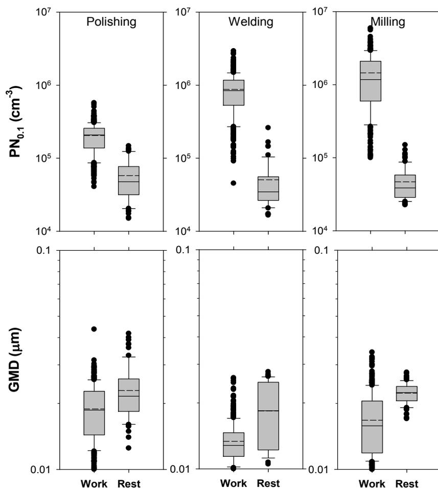
**Fig. 7.** Ambient nanoparticle number concentrations ( $PN_{0.1}$ ) during work and rest periods of metalworking operations, measured by the SMPS at a fixed point in close proximity (within 1.5 m) to the mannequin.
