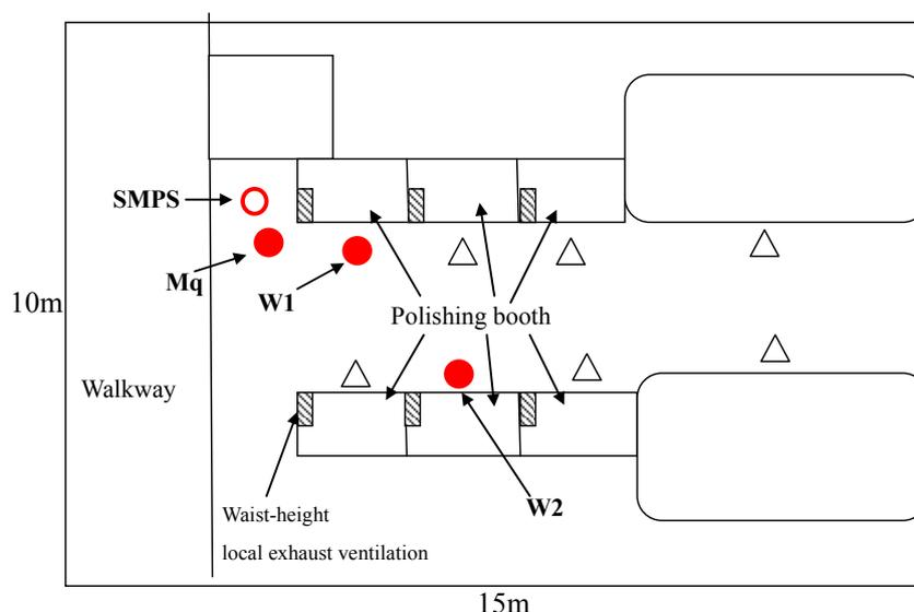
**Fig. 1.** Layout of the polishing operation plant. Solid circles represent workers (W) and mannequin (Mq) that wore the personal samplers, hallow circle shows the ambient air monitoring at fixed-location, and triangles represent other workers.
