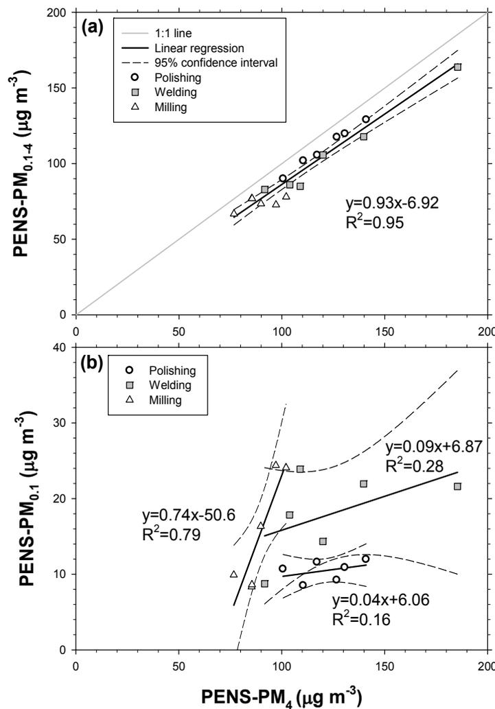
**Fig. 5.** Relationships between the respirable particles ( $PM_4$ ) and (a) 0.1–4  $\mu m$  particle ( $PM_{0.1-4}$ ), and (b) nanoparticle ( $PM_{0.1}$ ) mass concentrations measured by the PENS personal samplers at the three metalworking plants.
