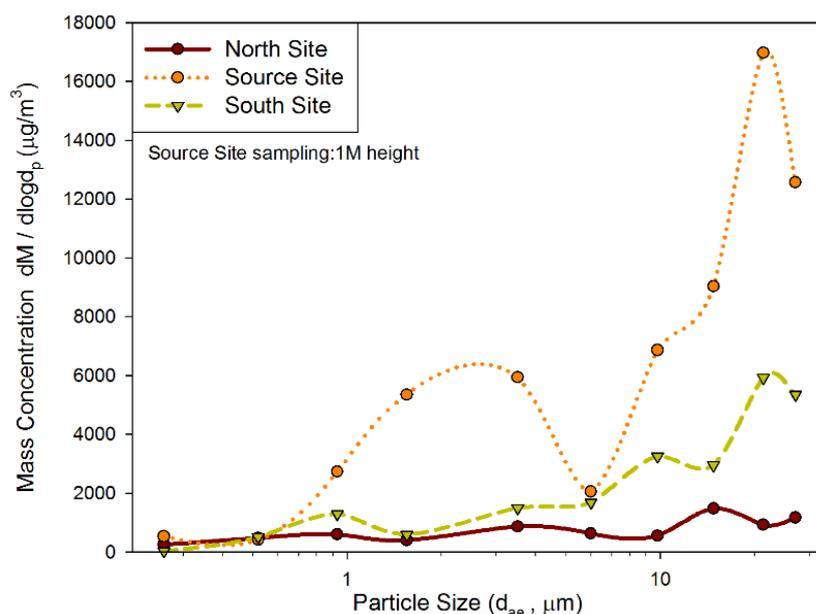
**Fig. 6.** The PM mass concentration and size distribution of horizontal sampling by using model 298 Marple samplers on January 15<sup>th</sup>, 2011.
