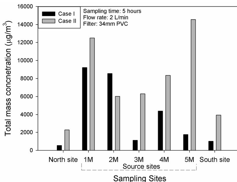
**Fig. 7.** The total PM mass concentration of two cases sampling by using model 298 Marple samplers.
