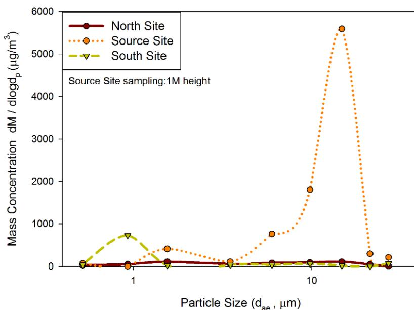
**Fig. 4.** The PM mass concentration and size distribution of horizontal sampling by using model 298 Marple samplers on November 26<sup>th</sup>, 2010.
