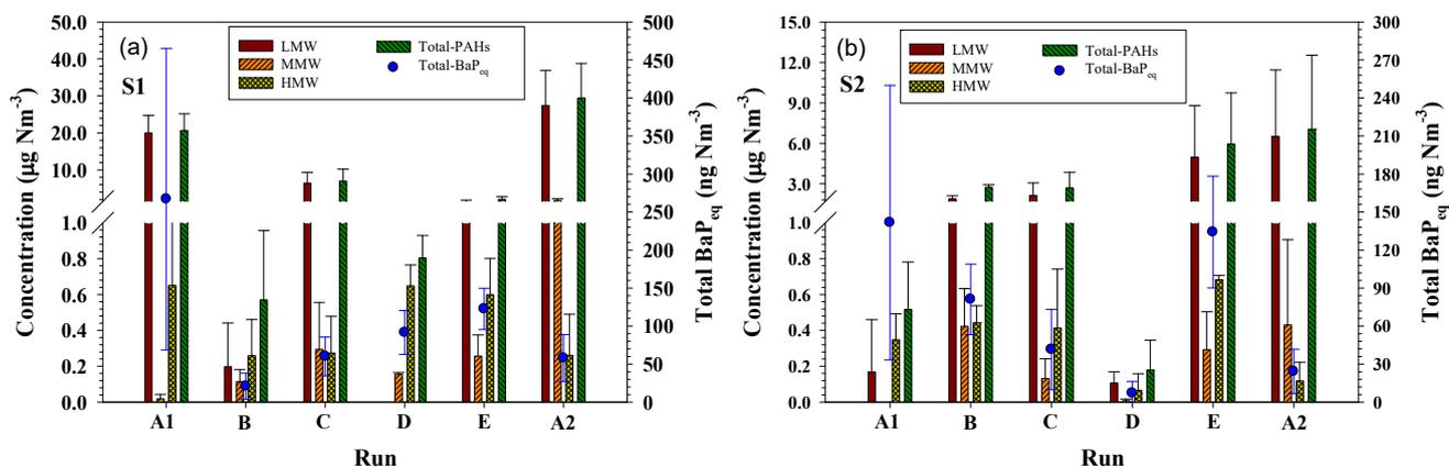
**Fig. 4.** Concentrations of LMW-, MMW-, HMW-, and Total-PAHs and Total-BaP<sub>eq</sub> of S1 (a) and S2 (b) at different runs (n = 3).
