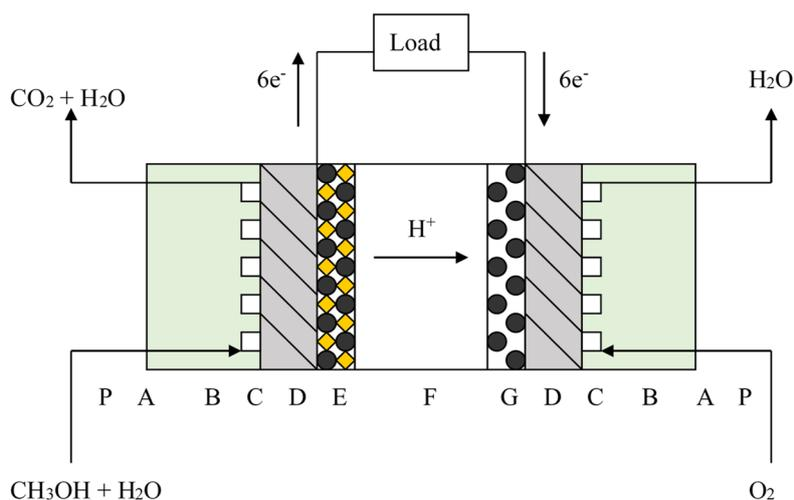
**Fig. 1.** The scheme of single DMFC with symmetrical components (A: current collector, B: graphite block, C: flow channel, D: gas diffusion layer, E: PtRu anode, F: Nafion membrane, G: Pt cathode, and P: end plate) (MEA: D + E + F + G + D).
