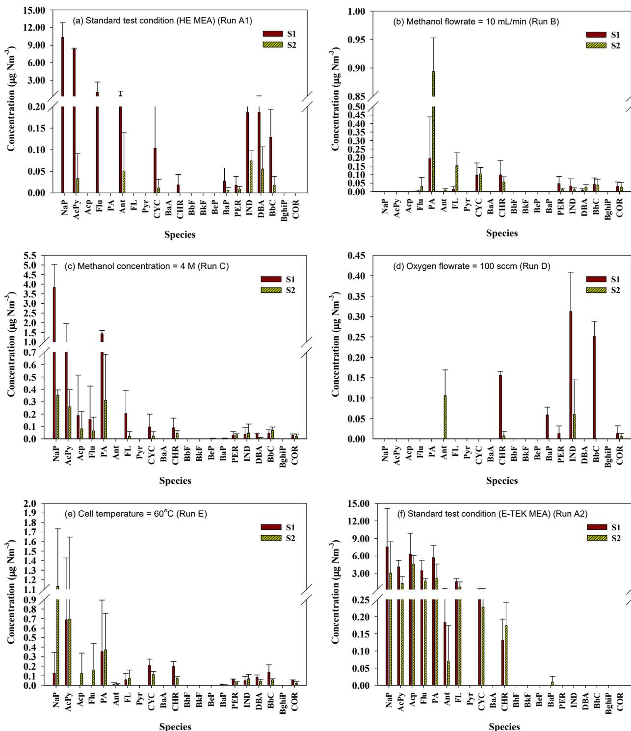
**Fig. 2.** PAHs concentrations of stage 1 (S1) and S2 of run A1 (methanol flowrate =  $2 \text{ mL min}^{-1}$ , methanol concentration = 2 M,  $\text{O}_2$  flowrate = 150 sccm, and cell temperature =  $80^\circ\text{C}$ ) (a) and the other runs operated at different operating parameters (b–f) ( $n = 3$ ).
