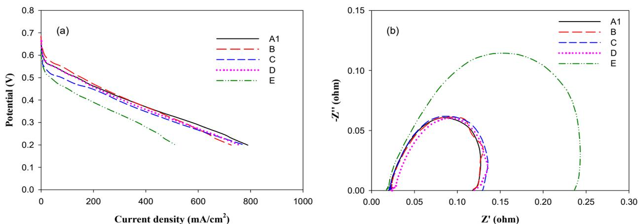
**Fig. 5.** (a) Cell potential versus current density ( $I$ – $V$ ) curves and (b) AC impedance Nyquist plots at  $0.5 \text{ V}$  ( $10 \text{ K}$ – $0.01 \text{ Hz}$ ) curves for the HE MEAs installed in DMFC operated at different runs (A1–E).
