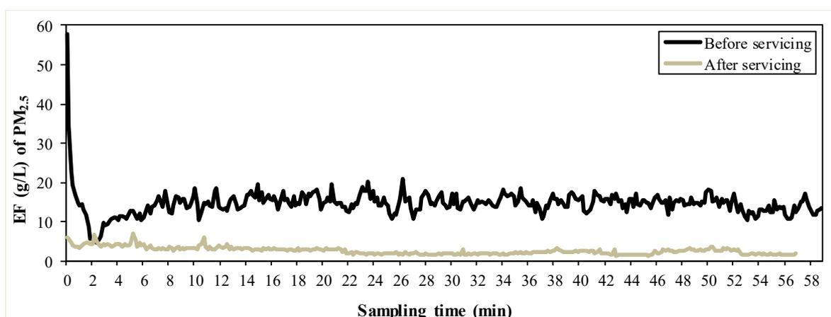
Fig. 5(b). Real-time EFs of PM<sub>2.5</sub> for pick-up before and after servicing.
