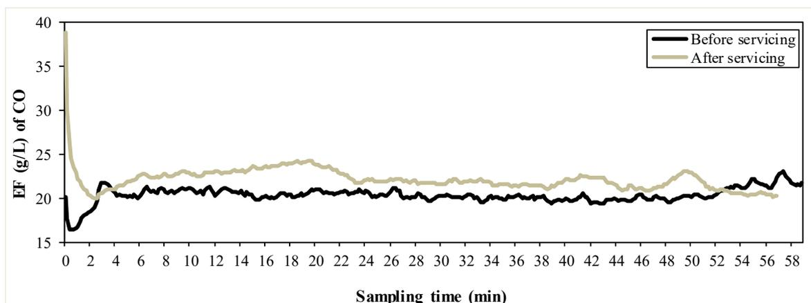
Fig. 5(a). Real-time EFs of CO for pick-up before and after servicing.
