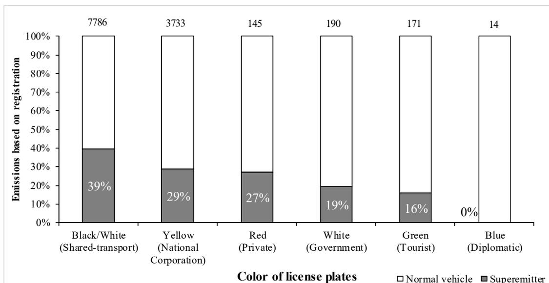
**Fig. 3(b).** Composition of superemitter vehicles based on registration. “Shared-transport” represents both the vehicles having black plates and white figures, and those with white plates and black figures. The numbers above each bar represent the total number of observed vehicles with particular color of license plates.
