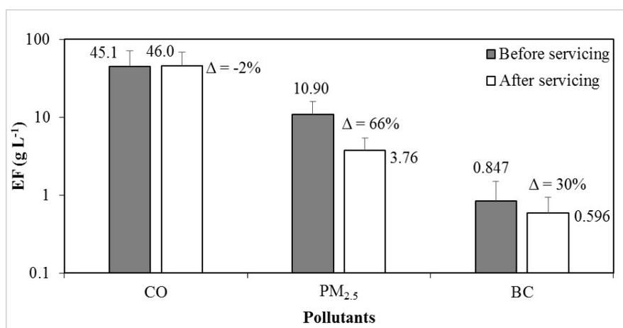
**Fig. 4.** Impact of servicing on EFs of CO, PM<sub>2.5</sub>, and BC. Servicing included changing the engine oil, and replacing oil, diesel and air filters.
