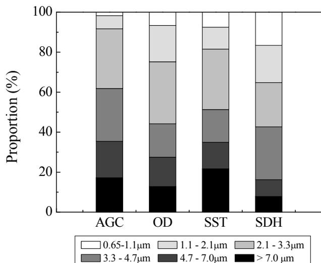
Fig. 4. Size distribution of airborne bacteria at different sewage treatment phases.
