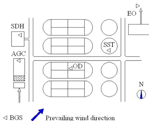
**Fig. 1.** Sketch of sampling sites at a municipal sewage treatment plant in Xi'an, China. AGC: aerated grit chamber; OD: oxidation ditch; SST: secondary settling tank; SDH: sludge dewatering house; EO: effluent outlet; BGS: background site;  $\Delta$ : sampling sites.
