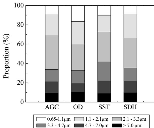
Fig. 5. Size distribution of airborne fungi at different sewage treatment phases.
