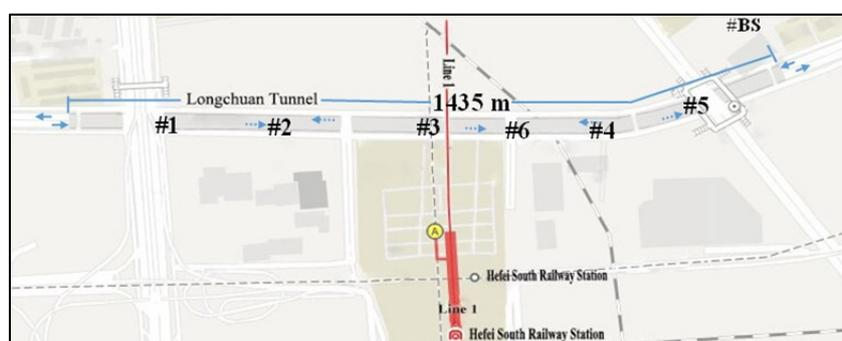
**Fig. 1.** Sampling sites and road layout of the tunnel experiment. The spatial distribution test was conducted at Sites #1, #2, #3, #4, and #5; the temporal distribution test was conducted at Sites #4 and #6; and the full experiment was conducted at Sites #2, #3, #4, and #6. BS indicates the background sampling site.
