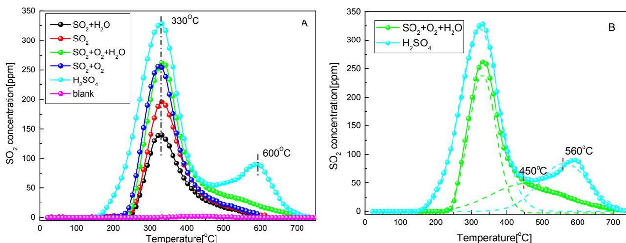
**Fig. 4.** TPD profiles of SO<sub>2</sub> from AC after adsorption tests. (a) Effect of pretreatment and (b) deconvolution results.
