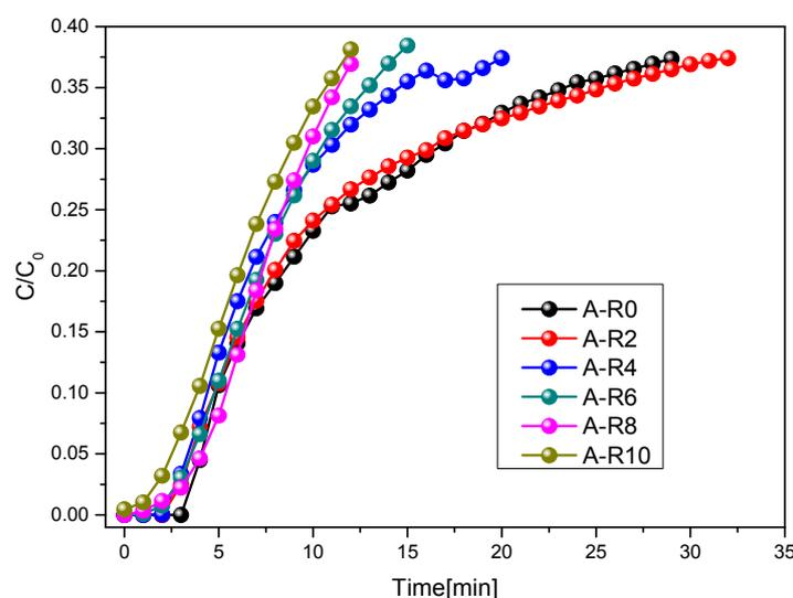
**Fig. 2.** Dynamic tests for SO<sub>2</sub> adsorption in samples with various cycles. Adsorption conditions: 1 vol.% SO<sub>2</sub>, 7 vol.% O<sub>2</sub>, 12 vol.% H<sub>2</sub>O, 120°C, 800 h<sup>-1</sup>. Desorption conditions: 400°C in N<sub>2</sub> for 1 h, 800 h<sup>-1</sup>.
