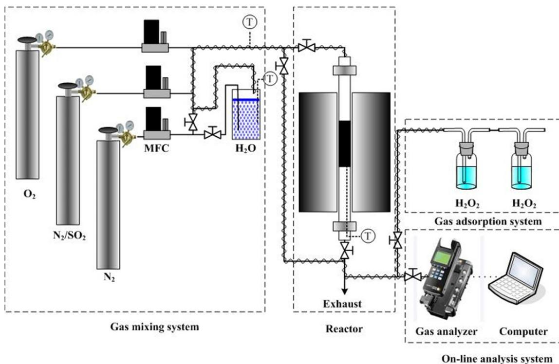
**Fig. 1.** Experimental installation for  $\text{SO}_2$  experiments (MFC, mass flow controller; T, temperature controller).
