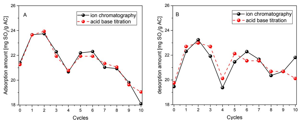
**Fig. 3.** SO<sub>2</sub> adsorption and desorption amounts for various cycles. Adsorption conditions: 1 vol.% SO<sub>2</sub>, 7 vol.% O<sub>2</sub>, 12 vol.% H<sub>2</sub>O, 120°C, 800 h<sup>-1</sup> for 1 h. Desorption conditions: 400°C in N<sub>2</sub> for 1 h, 800 h<sup>-1</sup>.
