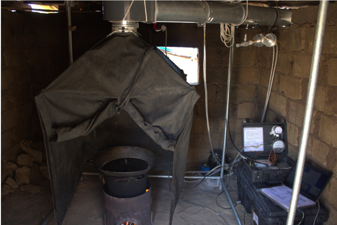
Figure S1- Portable Emission Monitoring System (PEMS), designed by the Aprovecho Research Centre.
