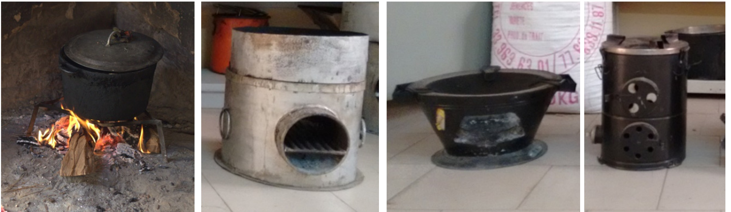
Figure S2- Cookstoves tested in the study. From left to right: three stones (traditional stove), Noflaye Jegg (rocket stove), Jambaar Bois (basic ceramic stove) and Prime Square (gasifier).
