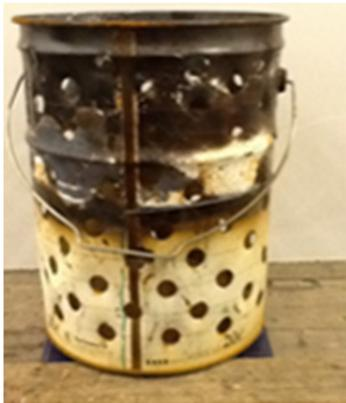
**Fig. 1.** Laboratory designed high ventilation stove.
