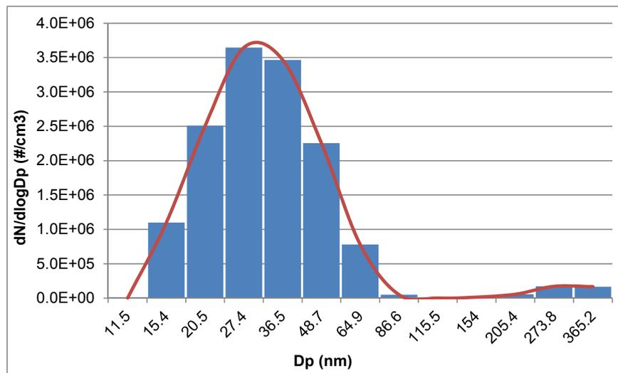
Fig. 8. Particle size distribution corresponding to the coking phase.
