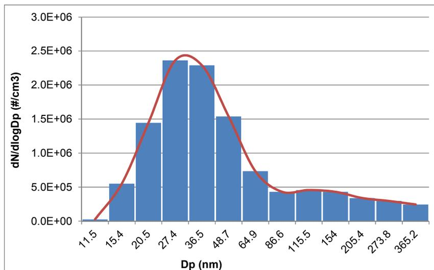
Fig. 10. Particle size distribution corresponding to the entire burn cycle.
