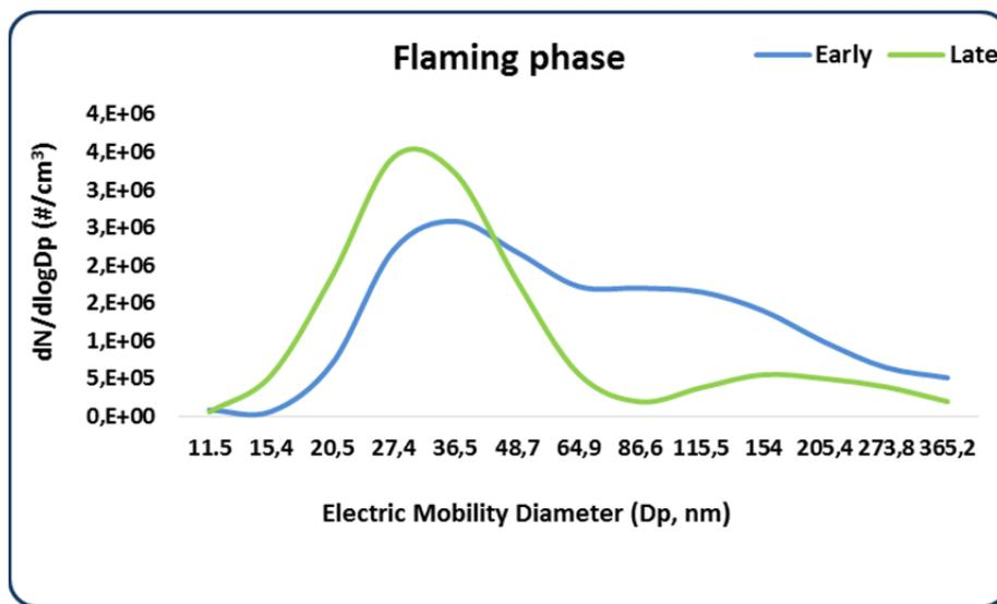
Fig. 7. Particle size distribution during early and late flaming.
