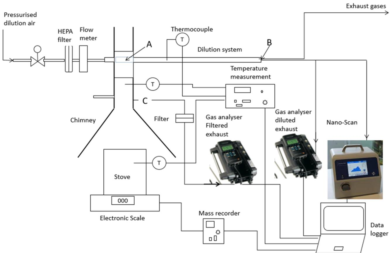
Fig. 2. Schematic diagram of the SeTAR Centre testing rig.
