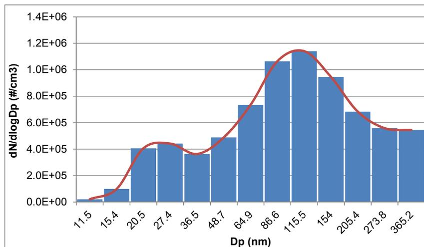
Fig. 4. Particle size distribution corresponding to the ignition phase.
