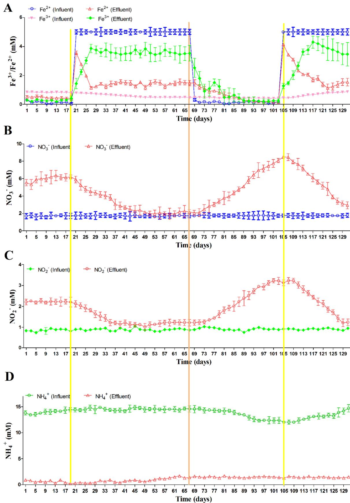
**Fig. 3.** Concentration of (A)  $\text{Fe}^{3+}$  and  $\text{Fe}^{2+}$ , (B)  $\text{NO}_3^-$ , (C)  $\text{NO}_2^-$  and (D)  $\text{NH}_4^+$ , in the UASB reactor. The yellow vertical solid lines represented the beginning of Fe(II) addition; the orange vertical solid lines represented the stop of Fe(II) addition.
