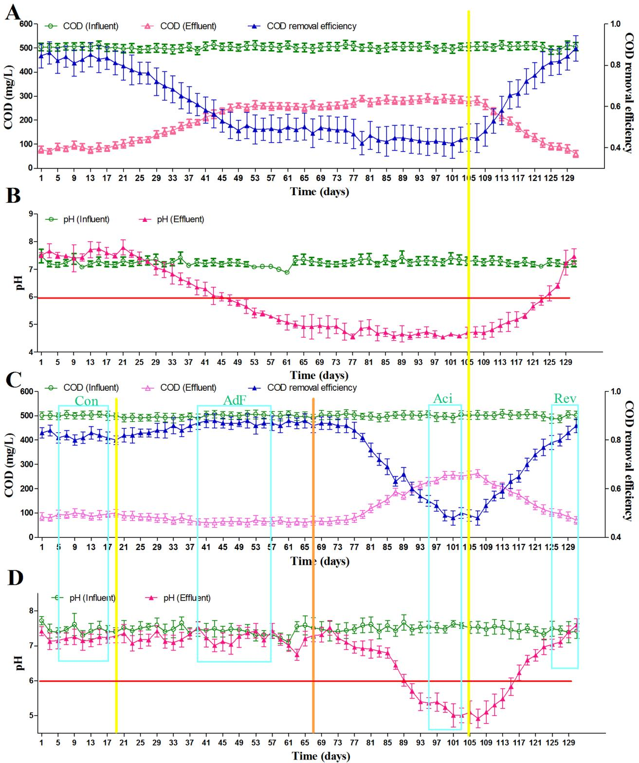
**Fig. 2.** Profiles of pH and COD removal efficiency with time in different UASB reactors. (A) and (B): control UASB reactor without the addition of Fe(II); (C) and (D): UASB reactor with Fe(II) addition; the yellow vertical solid lines represented the beginning of Fe(II) addition; the orange vertical solid lines represented the stop of Fe(II) addition; the box represented the sample for high-through sequencing.
