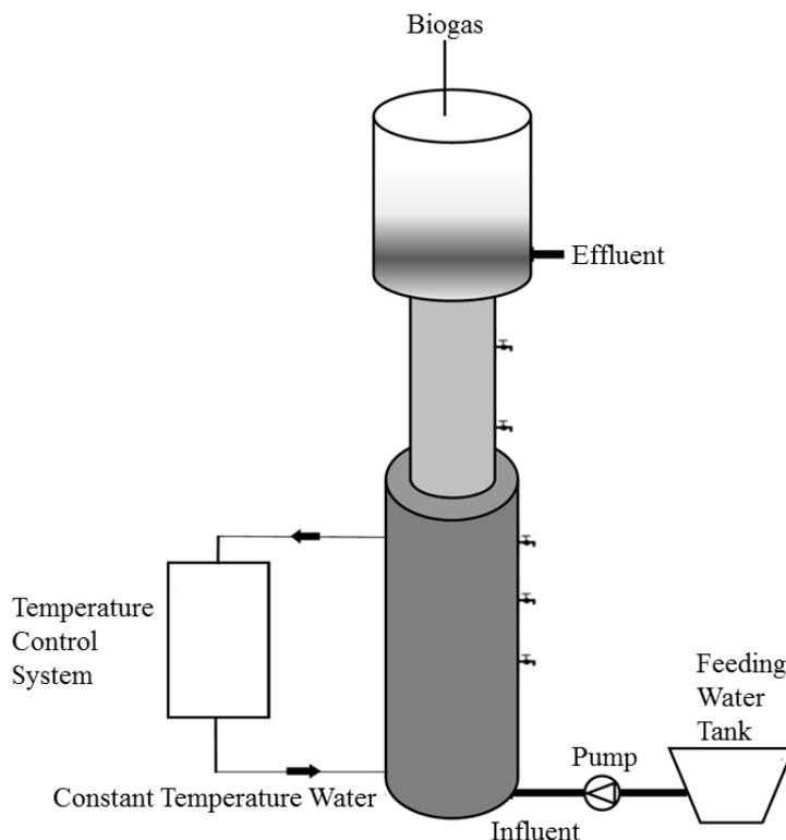
**Fig. 1.** The configuration of up-flow anaerobic sludge blanket.
