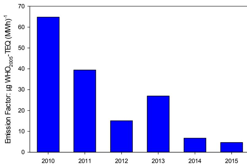
**Fig. 9.** The emission factor of total-PCDD/Fs -WHO<sub>2005</sub>-TEQ from the fly ash in the unit of electricity produced.
