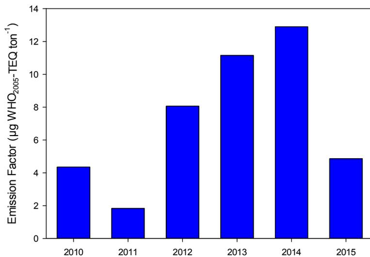
**Fig. 5.** The emission factor of total-PCDD/Fs-WHO-TEQ from the bottom ash in the unit weight of MSW treated.
