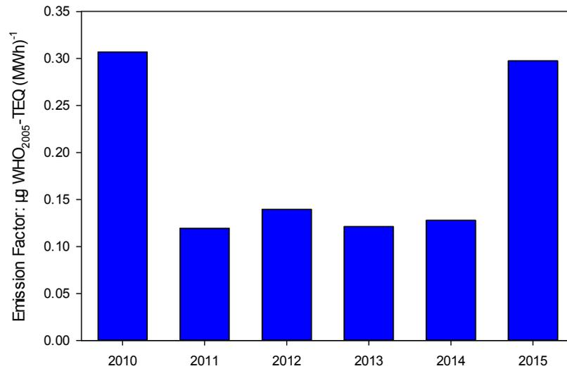
**Fig. 7.** The emission factor of total-PCDD/Fs -WHO<sub>2005</sub>-TEQ from the stack flue in the unit of electricity produced.
