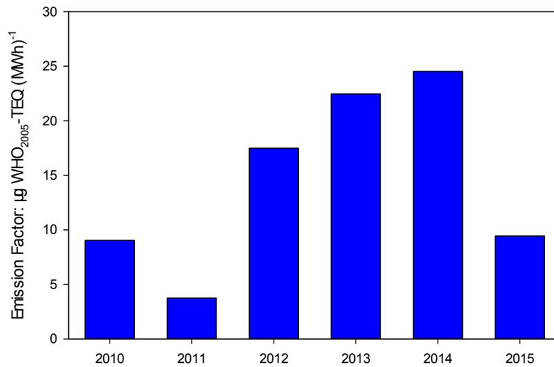
**Fig. 8.** The emission factor of total-PCDD/Fs -WHO<sub>2005</sub>-TEQ from the bottom ash in the unit of electricity produced.
