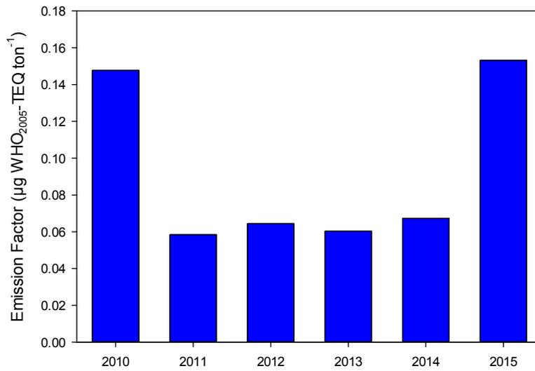
**Fig. 4.** The emission factor of total-PCDD/Fs-WHO-TEQ from the stack flue gas in the unit weight of MSW treated.
