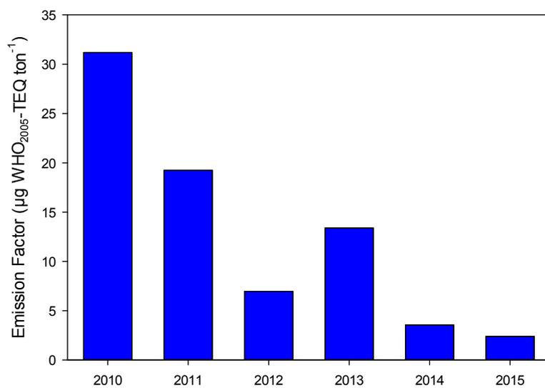
**Fig. 6.** The emission factor of total-PCDD/Fs-WHO-TEQ from the fly ash in the unit weight of MSW treated.
