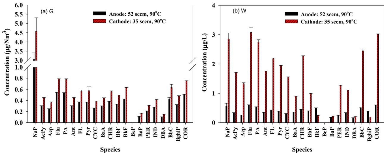
**Fig. 4.** Characteristic profiles of PAHs emitted at 90°C ((a) gas-phase (G) and (b) water-phase (W)) (anode/ cathode = 52/35 sccm) ( $n = 3$ ).
