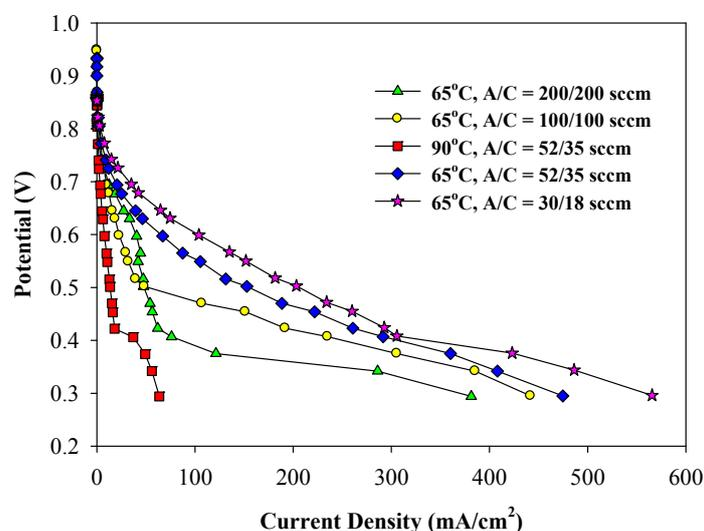
Fig. 8. Polarization (current-potential) curves under different operating conditions for the PEMFC.
