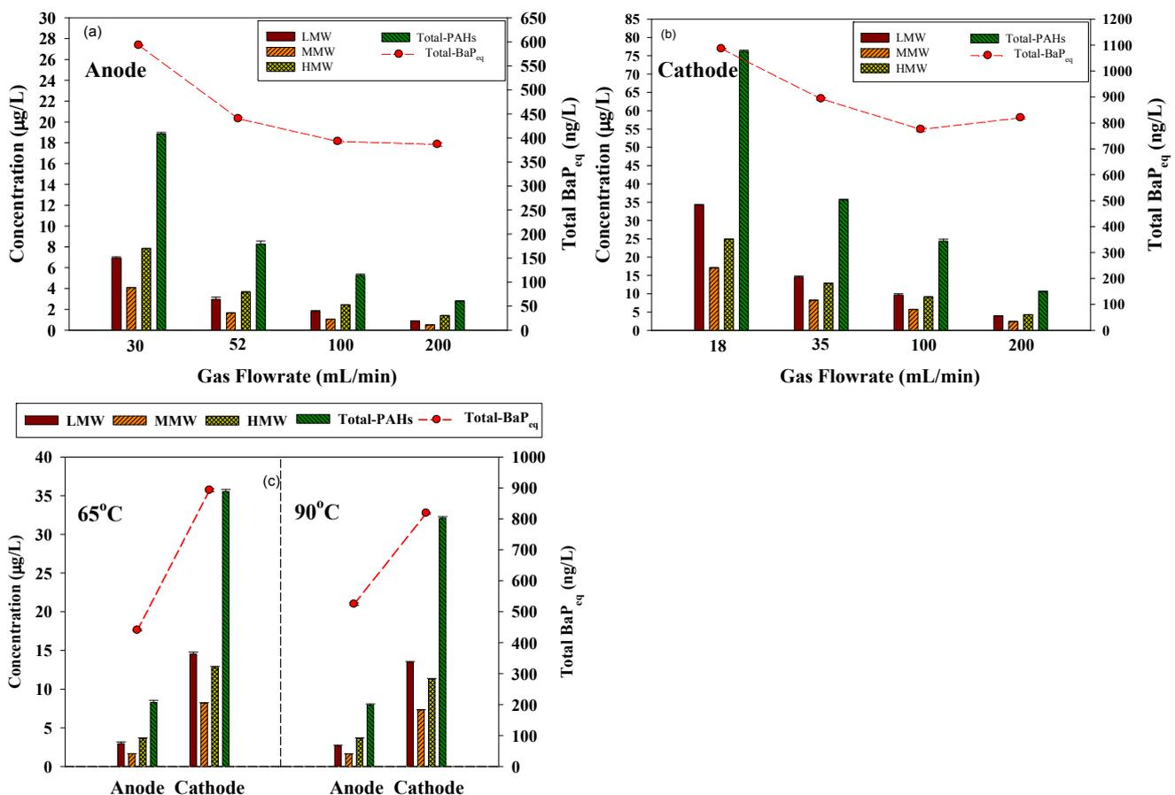
**Fig. 7.** Concentrations of water-phase LMW-, MMW-, HMW-, and Total-PAHs and Total- $\text{BaP}_{\text{eq}}$  at different flowrates ((a) anode and (b) cathode) and temperatures (c) ( $n = 3$ ).
