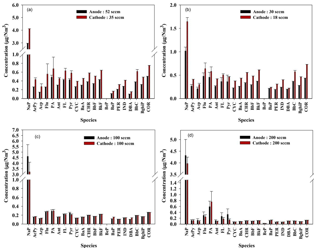
**Fig. 2.** Characteristic profiles of gas-phase PAHs emitted at different PEMFC anode/cathode flowrates (65°C): (a) 52/35, (b) 30/18, (c) 100/100, and (d) 200/200 sccm ( $n = 3$ ).
