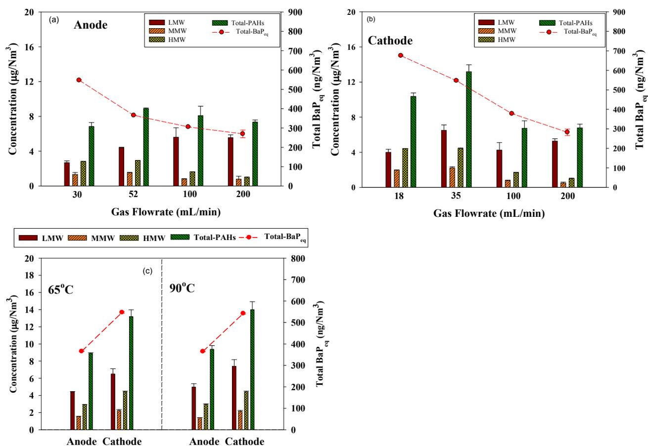
**Fig. 6.** Concentrations of gas-phase LMW-, MMW-, HMW-, and Total-PAHs and Total-BaP<sub>eq</sub> at different flowrates ((a) anode and (b) cathode) and temperatures (c) ( $n = 3$ ).
