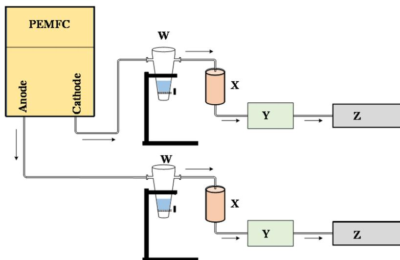
**Fig. 1.** The scheme of single PEMFC for PAH emission tests (W: water-phase PAHs collector, X: gas-phase PAHs collector (cartridge), Y: flow meter, and Z: pump).
