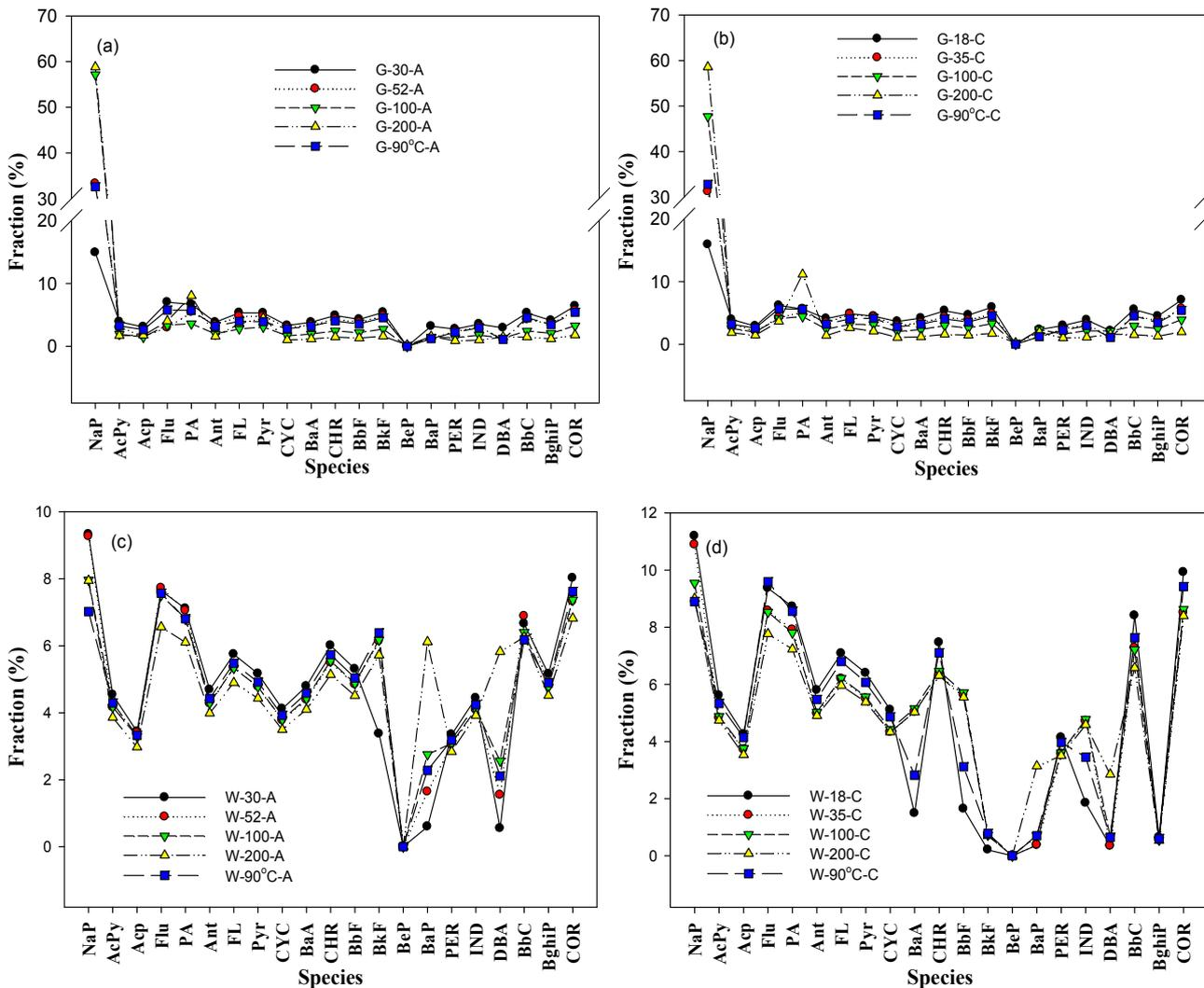
**Fig. 5.** Comparison of PAHs concentration fraction profiles (normalized to Total-PAHs concentration at different PEMFC anode/cathode flowrates (52/35, 30/18, 100/100, and 200/200 sccm) and temperature (65°C and 90°C) ( $n = 3$ )). (a) anode (A) gas-phase (G), (b) cathode (C) gas-phase, (c) anode water-phase (W), and (d) cathode water-phase.
