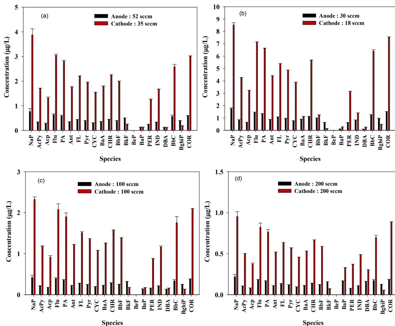
**Fig. 3.** Characteristic profiles of water-phase PAHs emitted at different PEMFC anode/cathode flowrates (65°C): (a) 52/35, (b) 30/18, (c) 100/100, and (d) 200/200 sccm ( $n = 3$ ).
