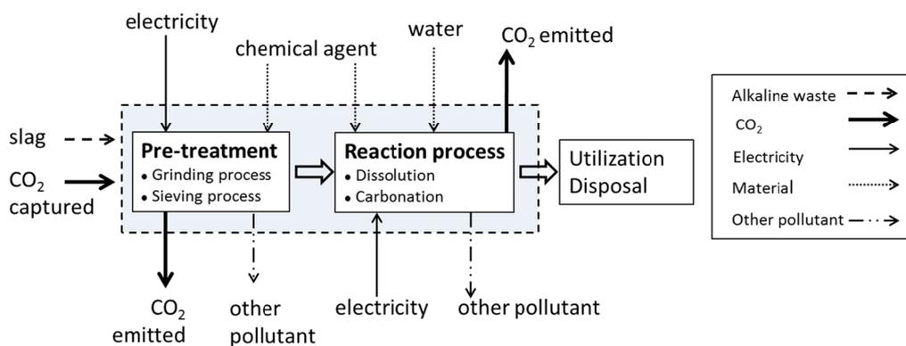
**Fig. 2.** System boundary of carbonation process defined for this study.
