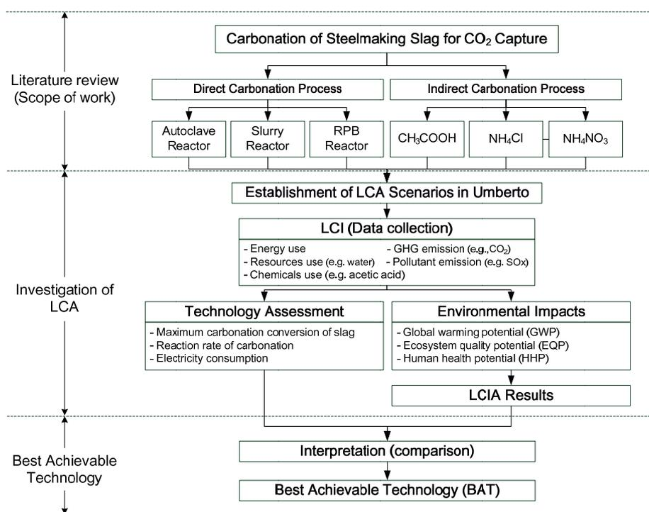
**Fig. 1.** Systematic comparison of carbonation processes for steelmaking slag by LCA.
