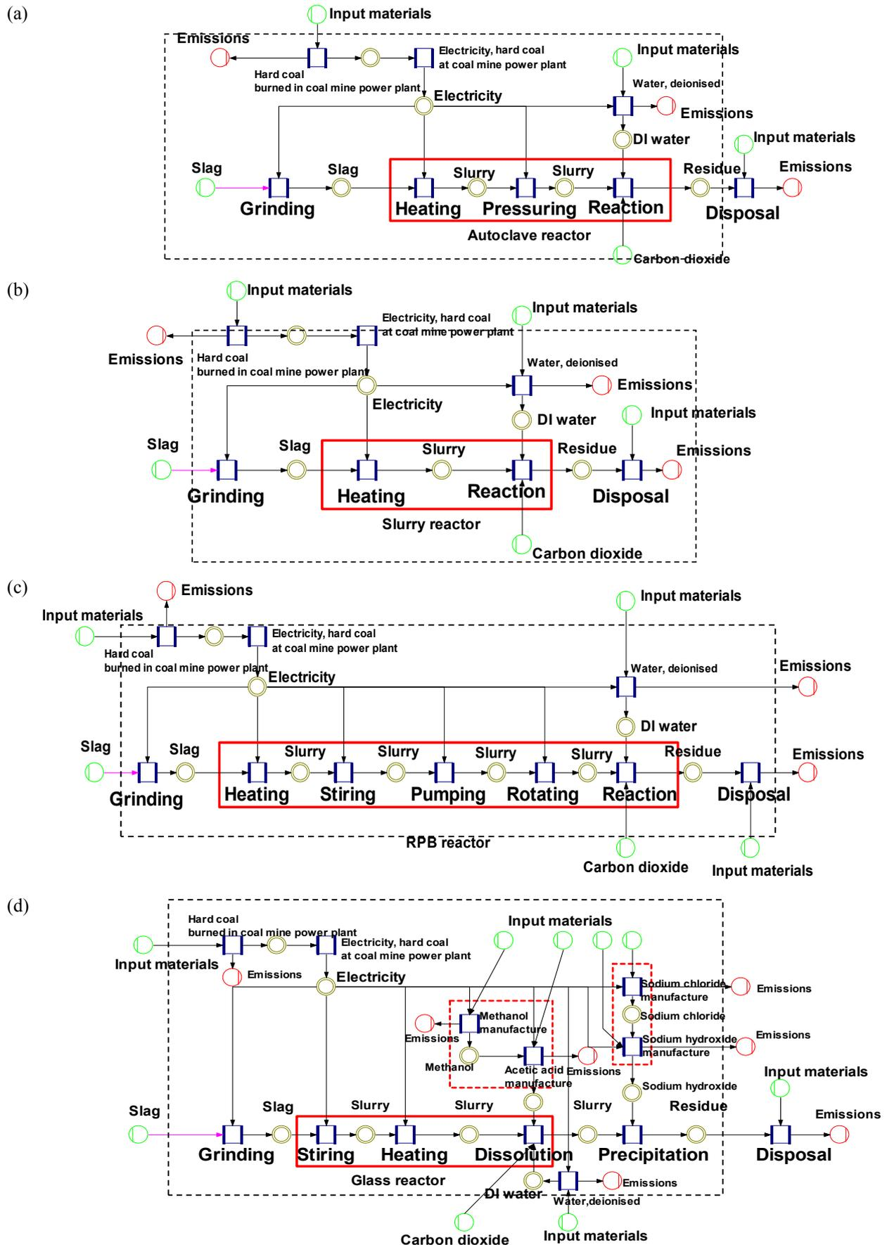
Fig. 3. Material and energy flow network of carbonation scenarios.
