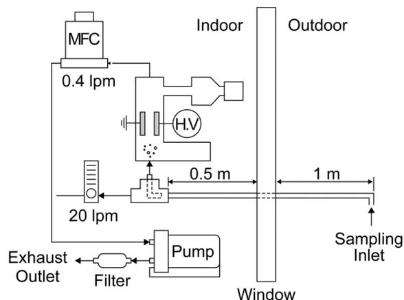
**Fig. 2.** Schematic of atmospheric particle sampling and measurement system.
