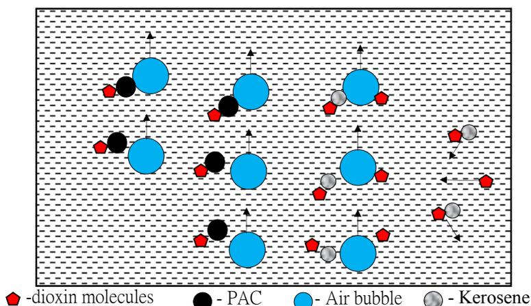
**Fig. 4.** Conceptual diagram of the dioxin removal by sorptive-flotation.
