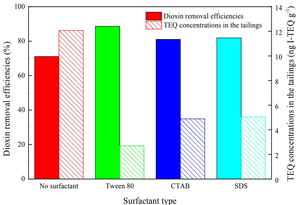
**Fig. 3.** Effect of surfactant type on dioxin removal efficiencies and TEQ concentrations in the tailings.
