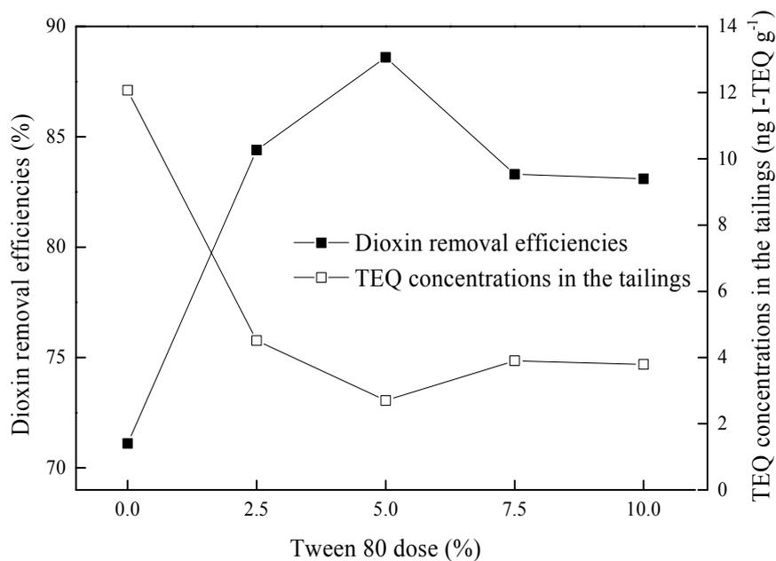
**Fig. 5.** Effect of Tween 80 dose on dioxin removal efficiencies and TEQ concentrations in the tailings.
