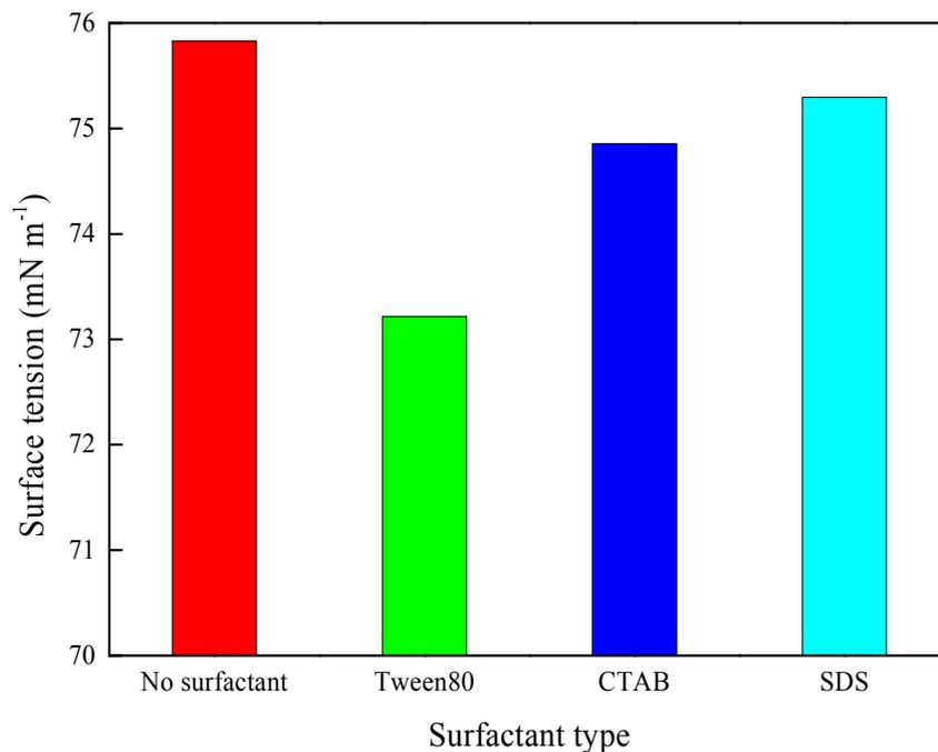
**Fig. 2.** Effect of surfactant type on surface tension of the slurry (5% (w/w) of dose).
