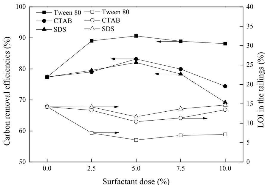
**Fig. 1.** Effect of surfactant type and dose on carbon removal efficiencies and LOI in the tailings.
