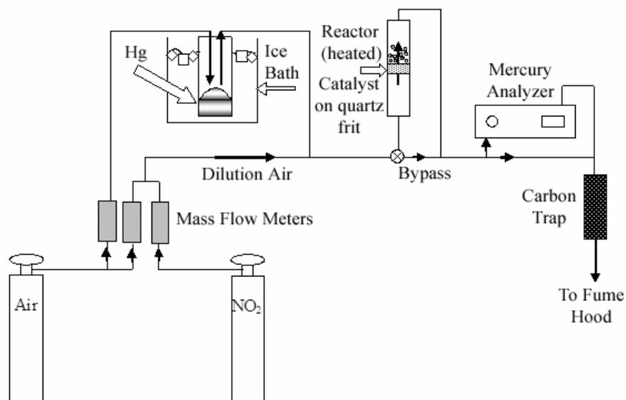
**Figure 3.** A schematic diagram of the experimental setup.
