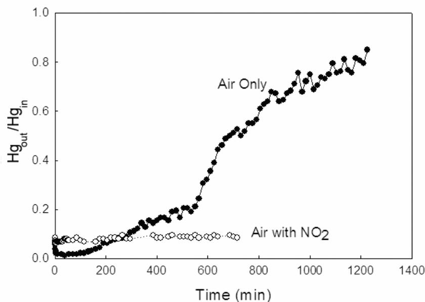
**Figure 5.** Representative results of saturations with 5 g of coated beads for air only and air with NO<sub>2</sub>.
