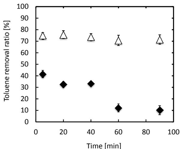
**Fig. 3.** Toluene removal for nonwoven ODC in the presence or absence of  $O_3$ . (◆): blank (no ozone), (△): ozone 38 ppm. Initial concentration of toluene: 10 ppm, gas flow rate:  $1.0 \text{ L min}^{-1}$ , RH: < 10 ppm.
