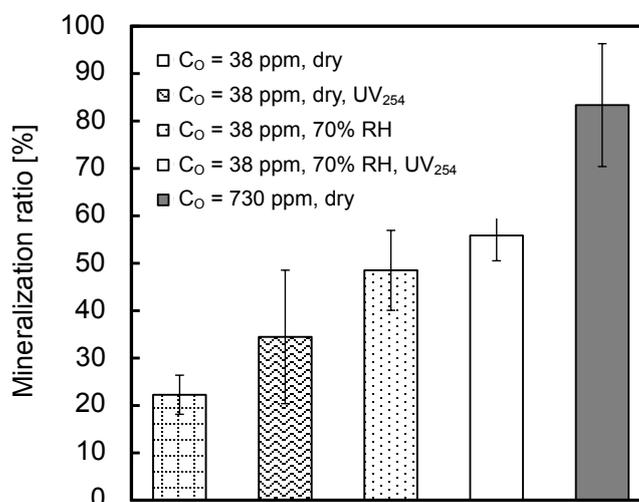
**Fig. 7.** Toluene mineralization ratio after 90 min under the same conditions as in Fig. 5. Initial concentration of toluene: 10 ppm, gas flow rate:  $1.0 \text{ L min}^{-1}$ , RH: < 10 ppm except for 70% RH ( $C_O$ : Initial ozone concentration).
