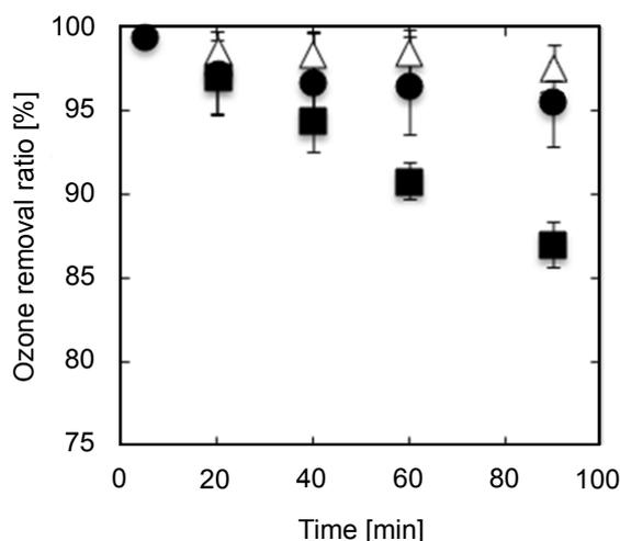
**Fig. 4.** Comparison of ozone removal ratio for nonwoven ODC under various conditions. (◆): ozone 38 ppm, (△): ozone 38 ppm with UV<sub>254</sub> irradiation, (■): ozone 38 ppm with 70% RH. Gas flow rate: 1.0 L min<sup>-1</sup>, RH: < 10 ppm except for 70% RH.
