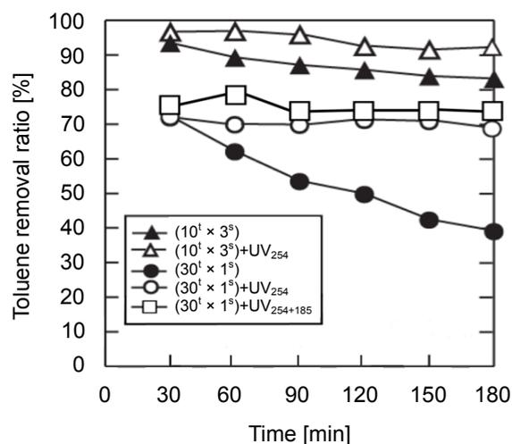
**Fig. 2.** Toluene removal ratio for honeycomb ODC for a single-step ( $30^t \times 1^s$ ) or three-step ( $10^t \times 3^s$ ) reactor with or without UV irradiation. Initial concentration of toluene: 40 ppm, initial concentration of ozone: 8 ppm, gas flow rate:  $5.0 \text{ L min}^{-1}$ , RH: < 10 ppm.
