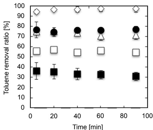
**Fig. 6.** Toluene removal ratios for nonwoven ODC under various conditions. (△): ozone 38 ppm, (●): ozone 38 ppm with UV<sub>254</sub> irradiation, (■): ozone 38 ppm with 70% RH, (□): ozone 38 ppm with 70% RH and UV<sub>254</sub> irradiation, (◇): ozone 730 ppm. Initial concentration of toluene: 10 ppm, gas flow rate: 1.0 L min<sup>-1</sup>, RH: < 10 ppm except for 70% RH.
