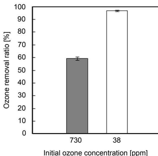
**Fig. 5.** Comparison of ozone removal ratio for nonwoven ODC without UV<sub>254</sub> irradiation after 90 min. Gas flow rate: 1.0 L min<sup>-1</sup>, RH: < 10 ppm.
