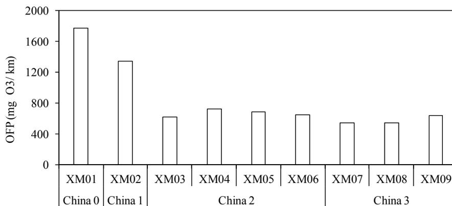
**Fig. 8.** Ozone-formation potential for all the tested vehicles.
