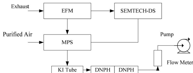
Fig. 1. PEMS for measuring carbonyl compounds in motor-vehicle exhaust.
