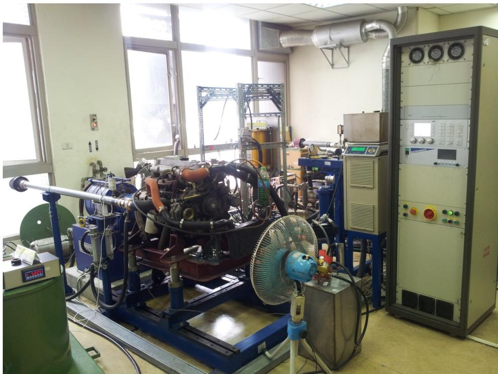
**Fig. 1.** Diesel engine and control system.
