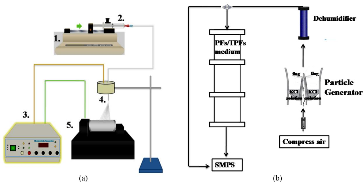
**Fig. 1.** (a) The experimental flowchart of TPFs preparation (1. The quantitative syringe, 2. cylinder, 3. high voltage supply, 4. needles, 5. Rotate the collector) (b) Filtration progress.
