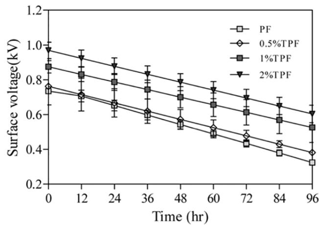
**Fig. 5.** Charge decay of the PFs and TPFs in every 12 hours (Temperature: 25°C; Humidity: 45%).
