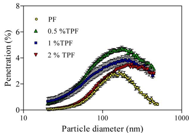
**Fig. 7.** Particle removal efficiency of TPFs by varies TiO<sub>2</sub> loading (basis weight: 1 g m<sup>-2</sup>; face velocity: 0.5 cm s<sup>-1</sup>).
