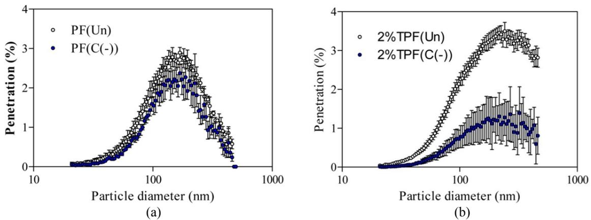
**Fig. 6.** Particle removal of TPFs under varies surface voltage with pure PFs and 2% TPFs ((Un) indicates the initial charged nanofibers and the (C(-)) indicates the charged nanofibers).
