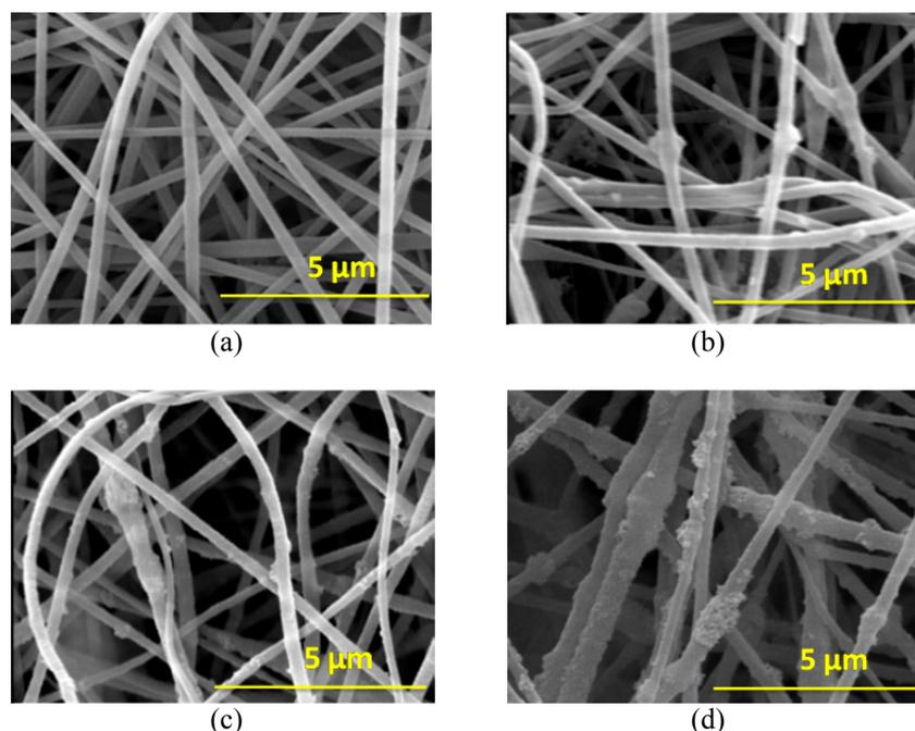
**Fig. 2.** SEM images of fibers with or without TiO<sub>2</sub> loading: (a) PFs, (b) 0.5%TPFs, (c) 1%TPFs, and (d) 2%TPFs.
