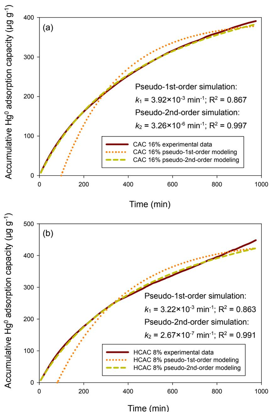
**Fig. 6.** Comparison of pseudo-first-order and pseudo-second-order kinetic simulations for (a)  $\text{N}_2$  condition and (b) simulated flue gas condition.
