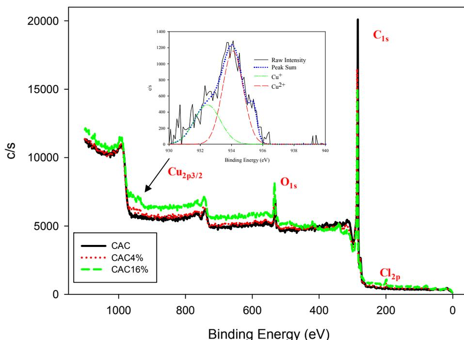
**Fig. 3.** XPS spectra of crude, 4% and 16% CuCl<sub>2</sub>-impregnated CAC samples and deconvoluted Cu<sub>2p3/2</sub> curves for CAC 16% sample.
