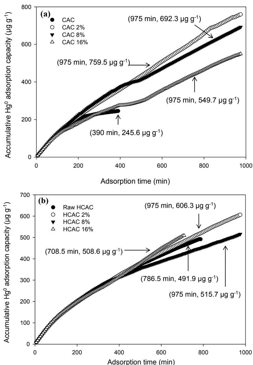
**Fig. 5.** Accumulative  $\text{Hg}^0$  adsorption capacity of (a) CAC and (b) HCAC under simulated flue gas condition.
