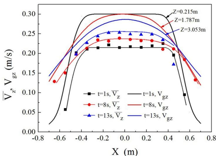
**Fig. 8.**  $\overline{V}_z$  of droplets in different regions and  $V_{gz}$  changes over time in Case 4.
