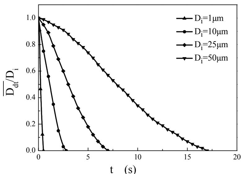
**Fig. 7.** The dimensionless diameter  $\overline{D}_{dt}/D_i$  change history of the droplets when ARH is 50%.
