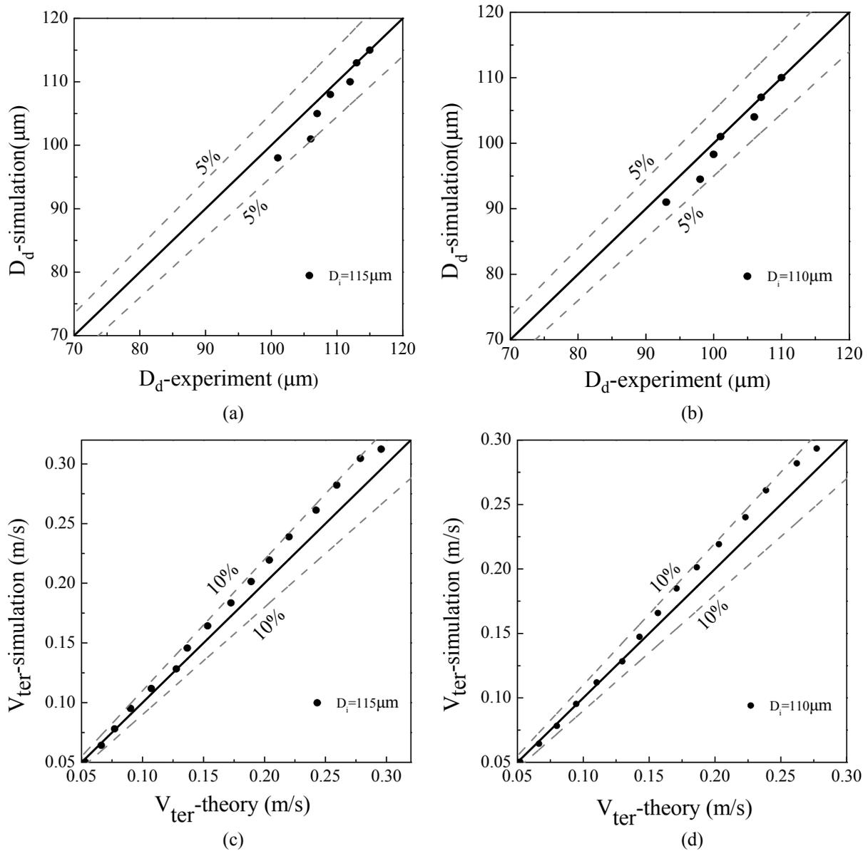
**Fig. 2.** Comparison of the experimental data and the simulation result (a) Comparison of  $D_d$  at the same drop height when  $D_i = 115 \mu\text{m}$ ; (b) Comparison of  $D_d$  at the same drop height when  $D_i = 110 \mu\text{m}$ ; (c) Comparison of  $v_{\text{ter}}$  at the same  $D_d$  when  $D_i = 115 \mu\text{m}$ ; (d) Comparison of  $v_{\text{ter}}$  at the same  $D_d$  when  $D_i = 110 \mu\text{m}$ .
