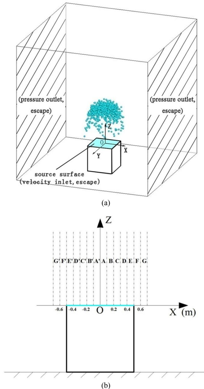
**Fig. 1.** Geometric schematic of droplets releasing from a tank in an industrial building (a) Geometric model; (b) The region schematic above the opening.
