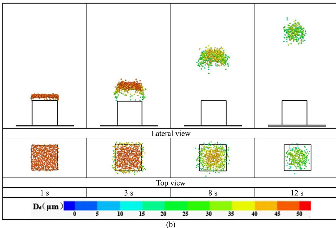
**Fig. 4.** Schematic diagram of the droplet diameter change history (a)  $D_i = 25 \mu\text{m}$  in Case 3; (b)  $D_i = 50 \mu\text{m}$  in Case 4.
