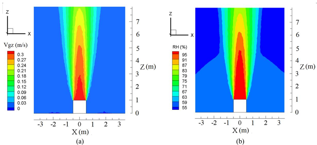
**Fig. 3.** The continuous phase parameter distribution when the ambient relative humidity is 50% (a) velocity component distribution along Z-axis; (b) relative humidity distribution.
