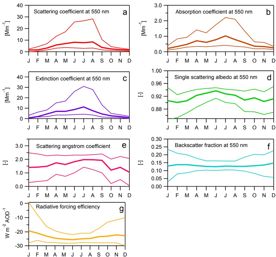
**Fig. 4.** Seasonal variation of dry optical aerosol properties at the Jungfraujoch from 1995–2007 (not corrected for scattering enhancement by water uptake), adapted from Andrews *et al.* (2011). The thick lines show the monthly median, and the thin lines the monthly 0.25 and 0.75 percentiles.
