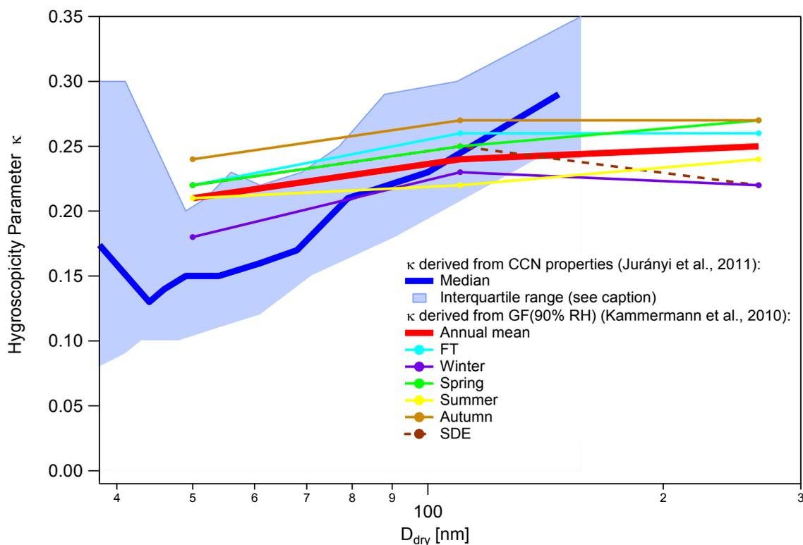
**Fig. 6.** Range of the hygroscopicity parameter  $\kappa$  found for the Jungfraujoch aerosol.  $\kappa$  derived from GF at RH = 90% (Kammermann *et al.*, 2010) are shown as annual mean values as well as separated by seasons and air mass types. The median and interquartile range (25<sup>th</sup> to 75<sup>th</sup> percentage) are shown for CCN-derived  $\kappa$  from Jurányi *et al.* (2011).
