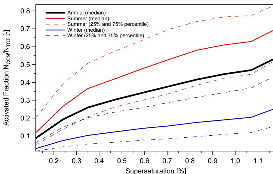
**Fig. 7.** Cloud condensation nuclei (CCN) climatology at the Jungfraujoch. Activated fraction calculated with CCN number concentrations from Jurányi *et al.* (2011) divided by number concentration of particles with diameter > 10 nm ( $N_{TOT}$ ).
