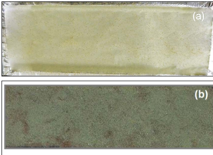
Figure S1. Image of the fungal surface on 3 rd day after incubation – Green colour indicates the formation of spores a) Aluminum foil and b) Cardboard.
