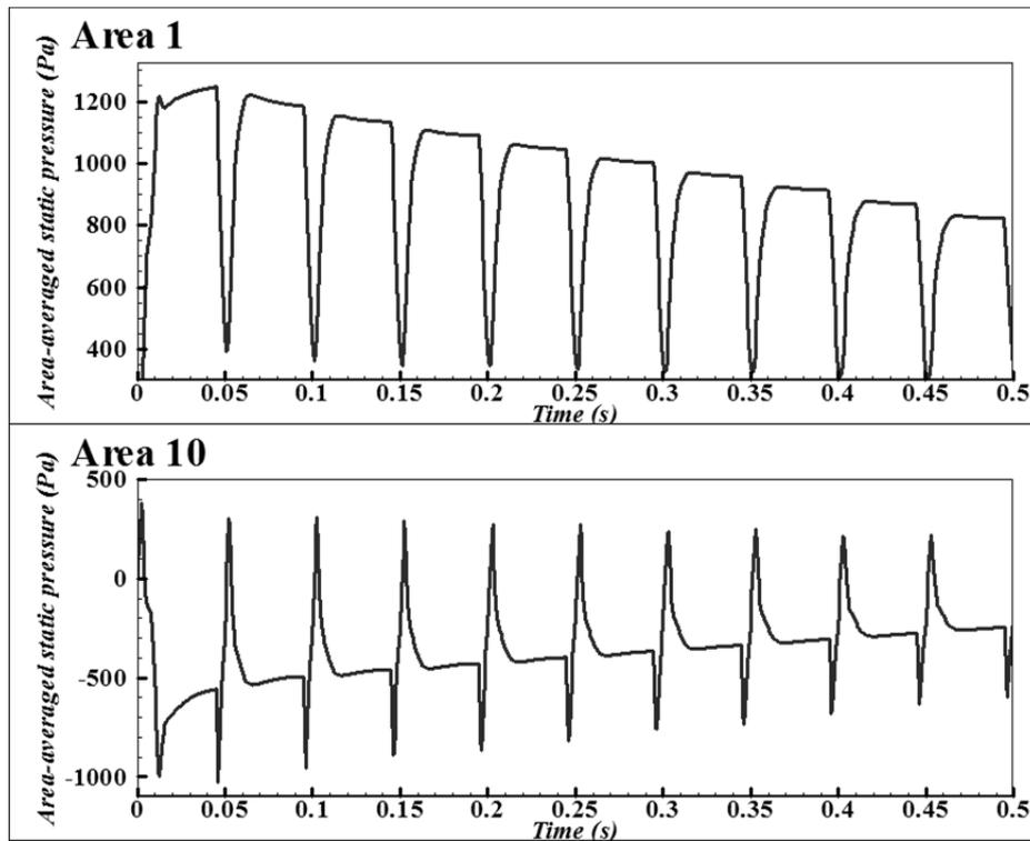
**Fig. 8.** Distribution of time-dependent area-averaged static pressure at the base and top regions of studied filter cartridges under the condition considering the decrease of gas tank pressure during a cleaning cycle ( $t = 0\text{--}0.5$  s).
