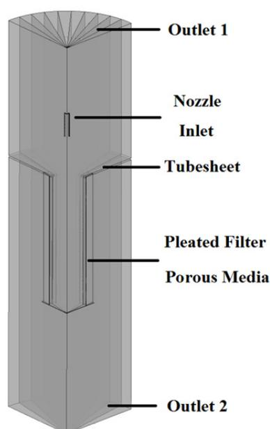
**Fig. 4.** Schematic diagram of a typical computational domain (10 copies, 1/4 circle).
