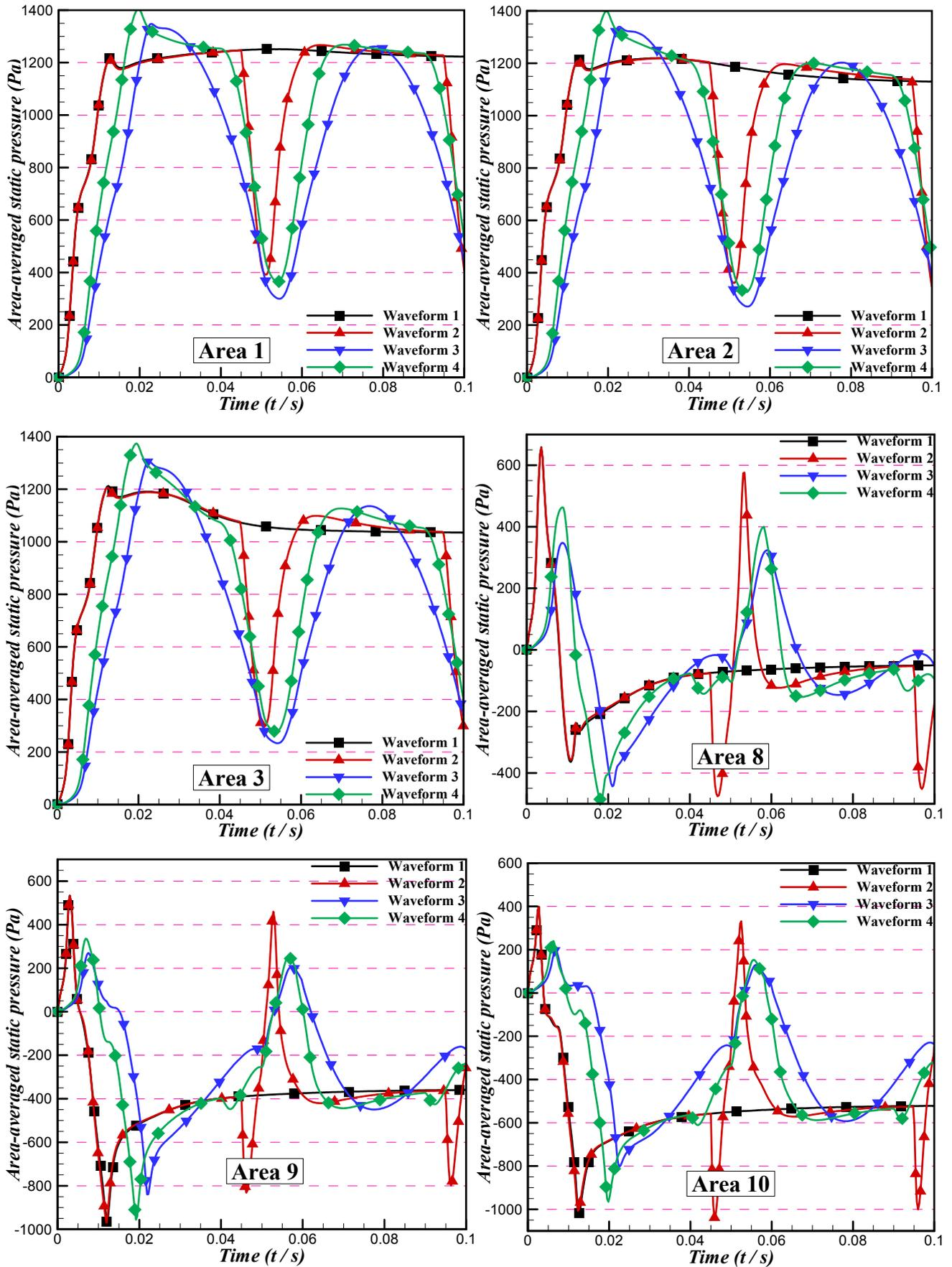
Fig. 6. Time-dependent area-averaged static pressure at selected sections of studied filter cartridges ( $t = 0\text{--}0.1$  s)
