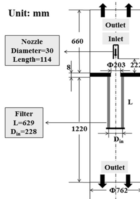
Fig. 2. Diagram of a studied filtration system with single filter cartridge in this study.
