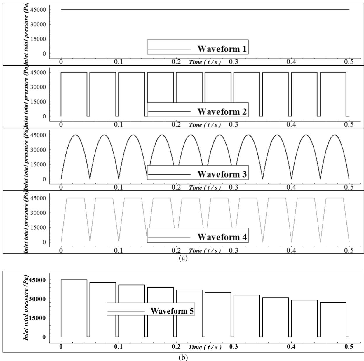
**Fig. 3.** Schematic diagram of studied reverse flow pulsing schemes (a) with constant peak inlet pressure; (b) with the consideration of peak inlet pressure reduction due to the depletion of gas tank during a cleaning cycle.
