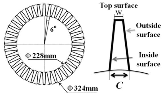
Fig. 1. Schematic diagram of studied filter cartridges with convergent trapezoidal pleats.
