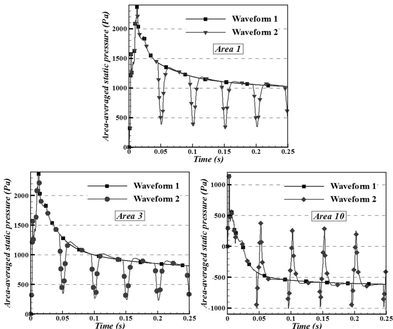
**Fig. 10.** Comparison of area-averaged static pressure difference as a function of time when applying the pulsing schemes of Waveform #1 and #2 and with the consideration of dust cake removal ( $t = 0\text{--}0.25$  s)
