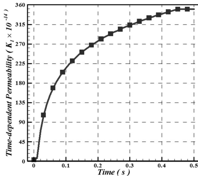
**Fig. 9.** Assumed transient permeability of media undergoing the dust cake removal in a cleaning cycle pulse
