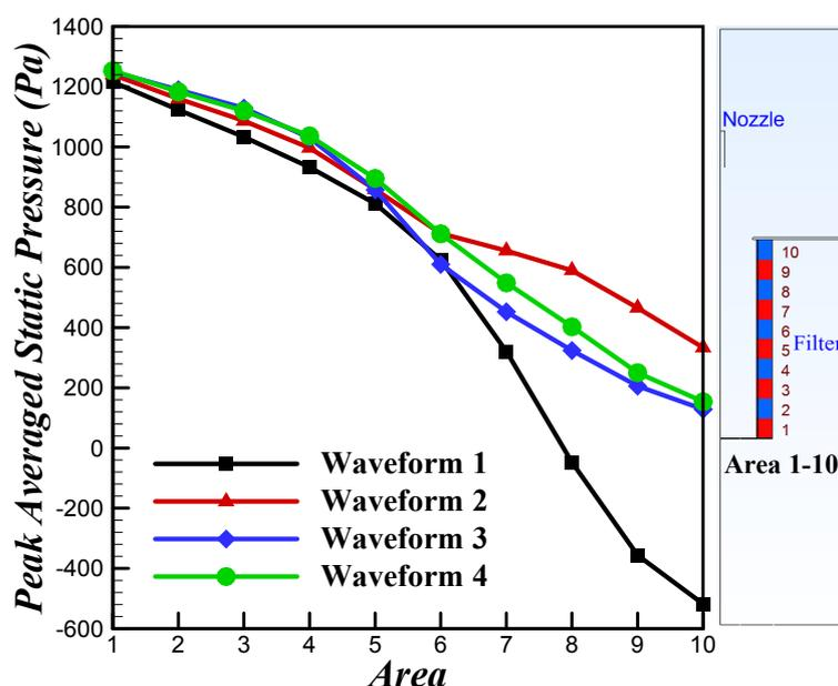
**Fig. 5.** Distribution of average peak pulse pressure at various sections of studied filter cartridges ( $t = 0.2\text{--}0.3$  s). Note that the base section of studied cartridge was labeled as Area 1 and the top section as Area 10.
