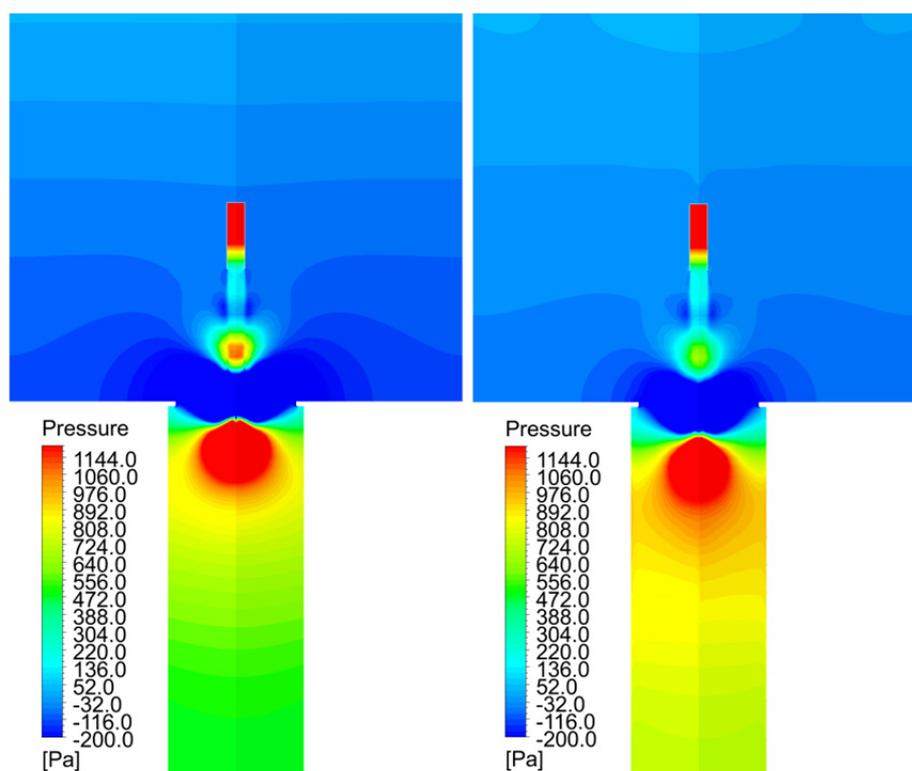
**Fig. 7.** Comparison of transient static-pressure distribution at two selected time instances in the case with the pulsing scheme of Waveform 2: (a) the 1<sup>st</sup> pulse jet,  $t = 0.003$  s; (b) the 4<sup>th</sup> pulse jet,  $t = 0.153$  s.
