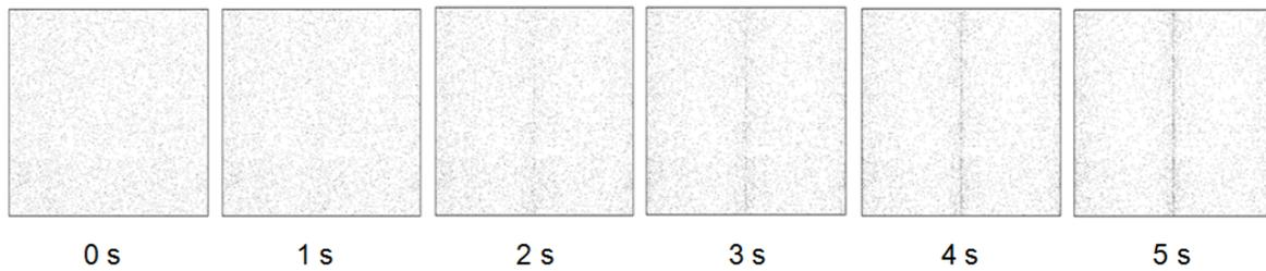
**Fig. 3.** Evolution of particle spatial distribution with time.  $L = 155$  dB,  $f = 5000$  Hz.
