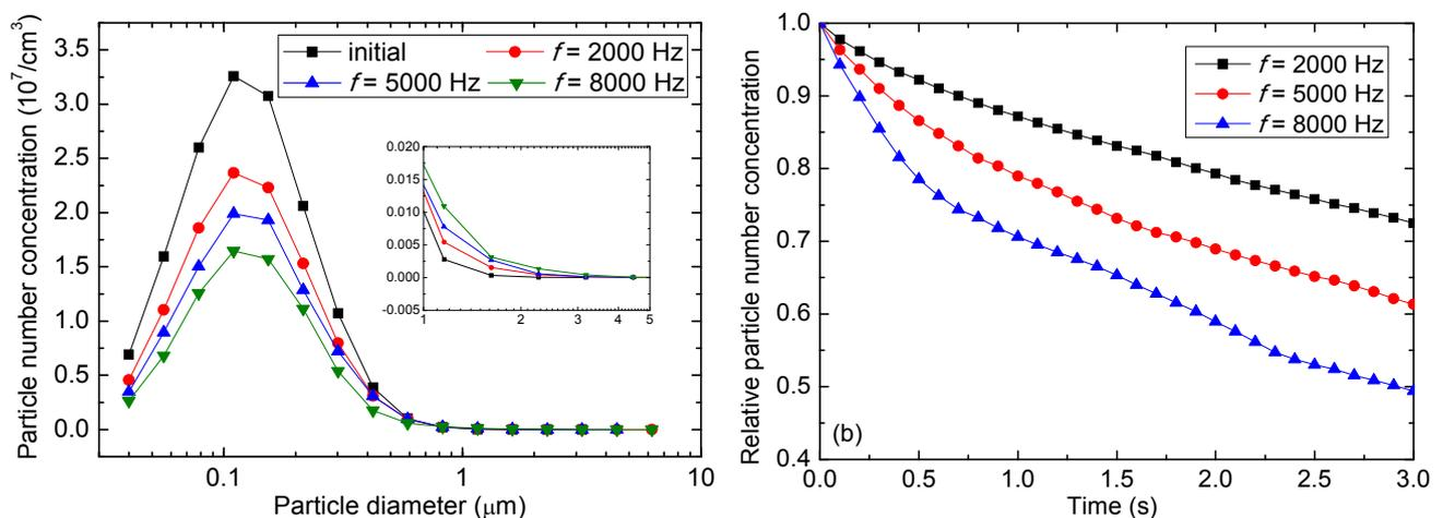
**Fig. 5.** Effect of acoustic frequency on acoustic agglomeration.  $L = 155$  dB,  $t = 3$  s. (a) Particle size distribution before and after acoustic agglomeration. (b) Evolution of total particle number concentration with time.
