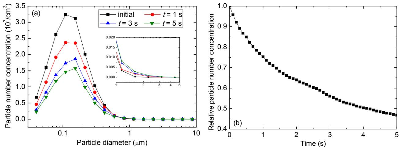
**Fig. 4.** Evolution of particle size and concentration with time.  $L = 155$  dB,  $f = 5000$  Hz. (a) Evolution of particle size distribution with time. (b) Evolution of total particle number concentration with time.
