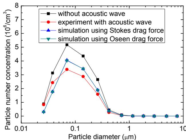
**Fig. 1.** Comparison with experiment of Zhao (2007).  $L = 158.5$  dB,  $f = 1000$  Hz,  $t = 3.2$  s.
