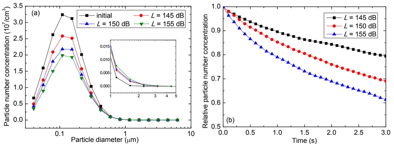
**Fig. 6.** Effect of acoustic intensity on acoustic agglomeration.  $f = 5000$  Hz,  $t = 3$  s. (a) Particle size distribution before and after acoustic agglomeration. (b) Evolution of total particle number concentration with time.
