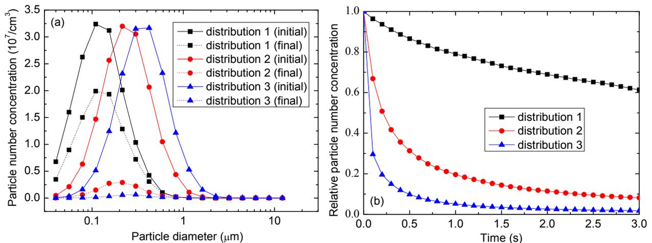
**Fig. 7.** Effect of particle size distribution on acoustic agglomeration.  $L = 155$  dB,  $f = 5000$  Hz,  $t = 3$  s. (a) Particle size distribution before and after acoustic agglomeration. (b) Evolution of total particle number concentration with time.
