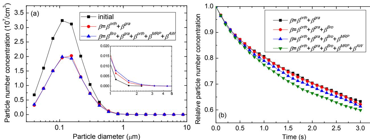
**Fig. 2.** Comparison of the effects of agglomeration mechanisms.  $L = 155$  dB,  $f = 5000$  Hz,  $t = 3$  s. (a) Particle size distribution before and after acoustic agglomeration. (b) Evolution of total particle number concentration with time
