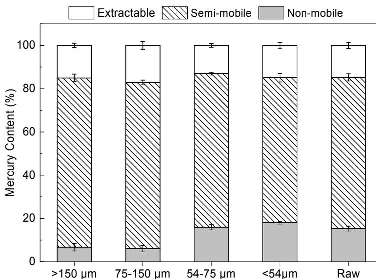
**Fig. 4.** Mercury species and concentrations with the error bar (standard deviation) in raw/sorted FA samples.
