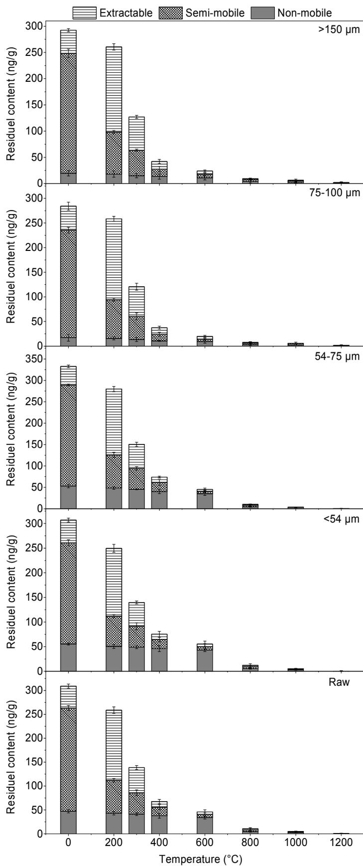
**Fig. 6.** Species distribution of mercury with the error bar (standard deviation) in raw/sorted FA samples during thermal treatment.
