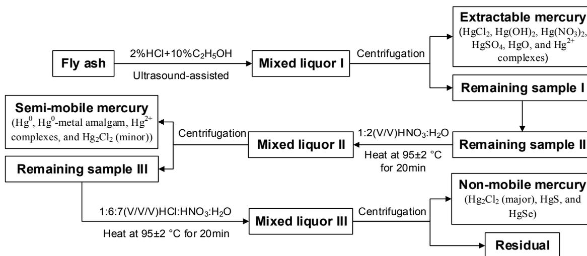
**Fig. 1.** Sequential extraction procedure and mercury fractions (extractable, semi-mobile and non-mobile) corresponding with individual species.
