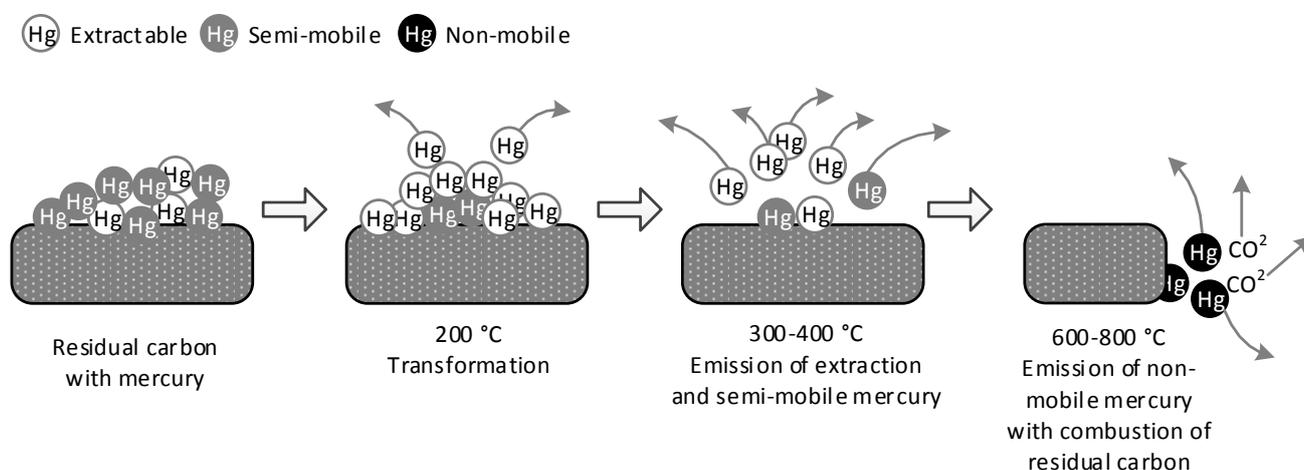
Fig. 7. Mechanism of desorption process of mercury on the residual carbon in FA.
