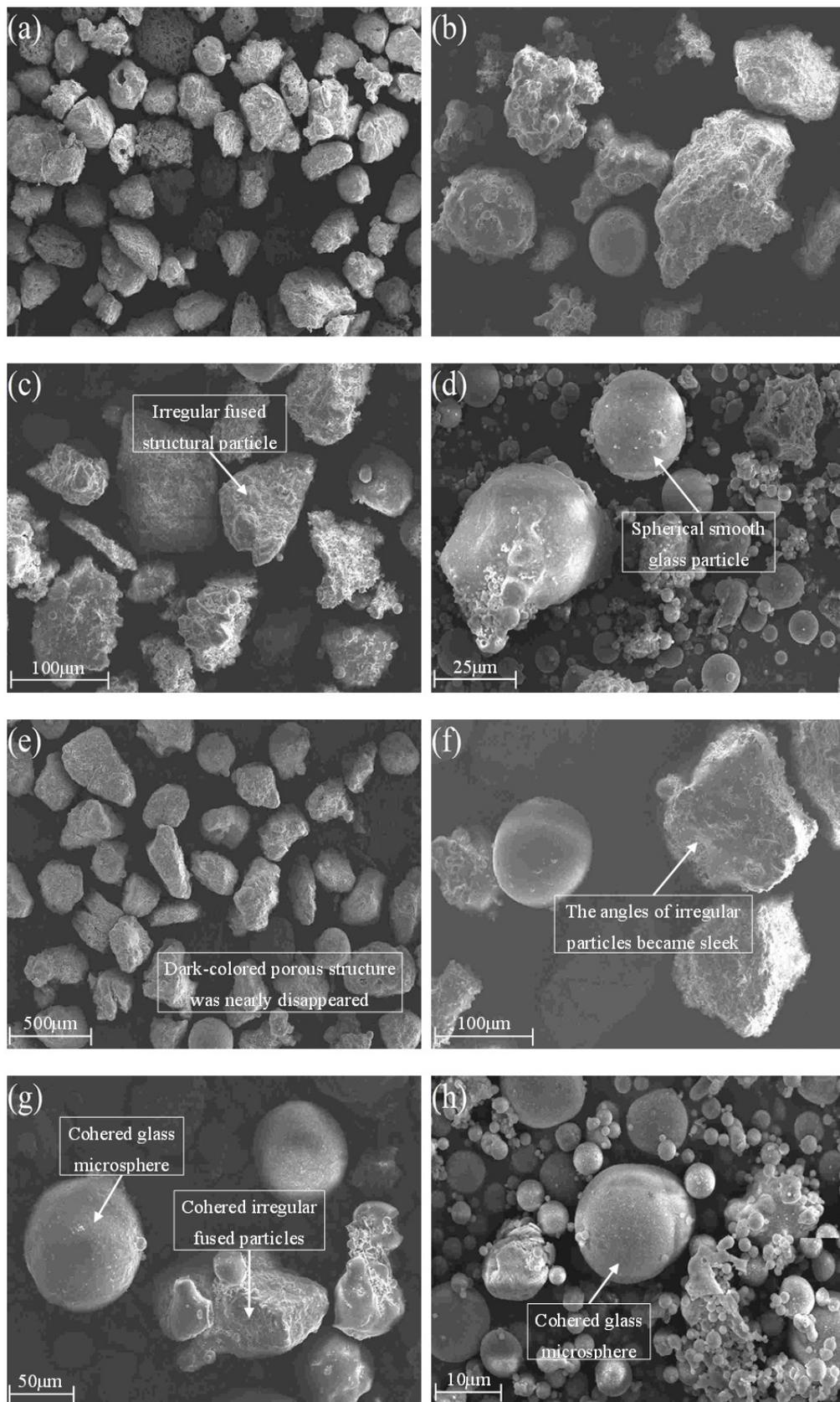
**Fig. 3.** Superficial morphology of the sorted FA samples without thermal treatment (a–d) and heated at 800°C (e–h). (a) > 150 μm size grade (× 50); (b) 75–150 μm size grade (× 200); (c) 54–75 μm size grade (× 300); (d) < 54 μm size grade (× 1000). (e) > 150 μm size grade (× 50); (f) 75–150 μm size grade (× 300); (g) 54–75 μm size grade (× 400); (h) < 54 μm size grade (× 2000).
