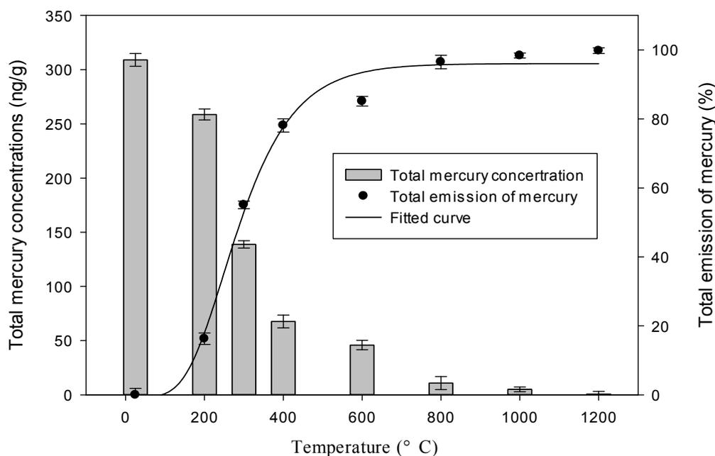
**Fig. 5.** Total mercury concentrations and total emission of mercury with the error bar (standard deviation) in raw FA sample during thermal treatment.
