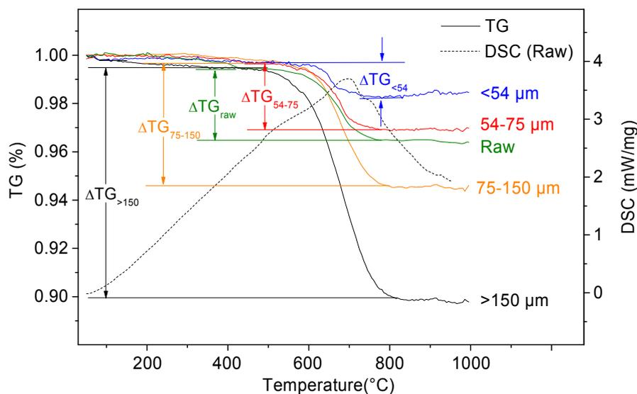
Fig. 2. TG-DSC curve and  $\Delta\text{TG}$  of the raw and sorted FA samples.
