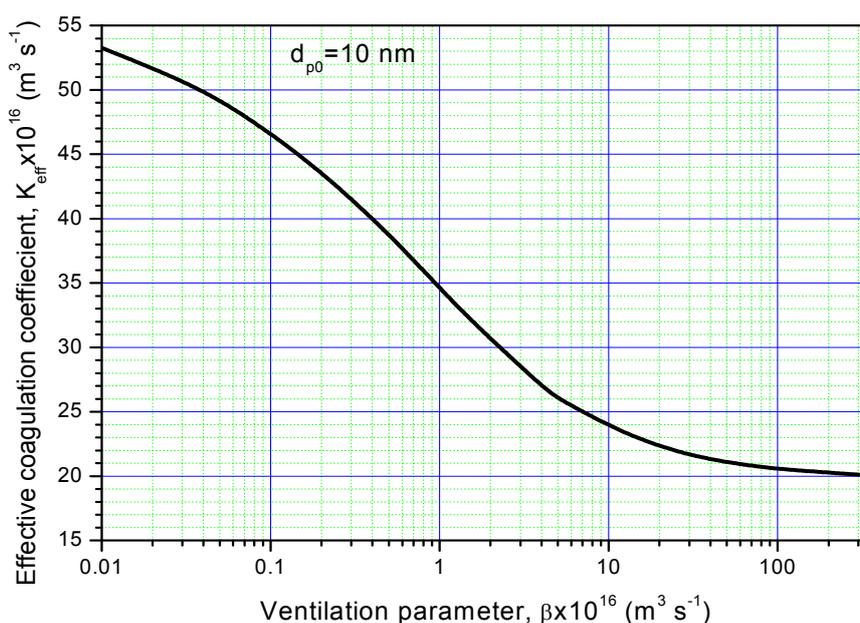
**Fig. 2.** Effective coagulation kernel ( $K_{eff}$ ) computed for an initial particle diameter ( $d_{p0}$ ) of 10 nm using Eqs. (4)–(6).
