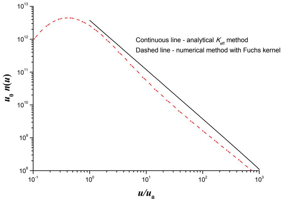
**Fig. 3.** Steady-state number size distributions for a typical aerosol system ( $S = 10^{11} \text{ m}^{-3} \text{ s}^{-1}$ ) for (i) constant kernel ( $K_{eff}$ ) solution (Eq. (3)) with  $d_{p0} = 10 \text{ nm}$ , and (ii) numerical solution using Fuchs kernel (CMD = 10 nm; GSD – 1.3).
