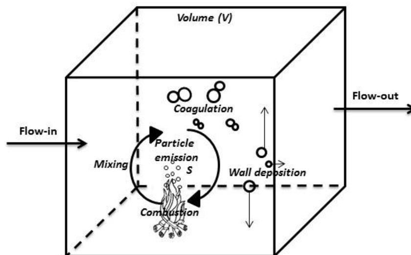
Fig. 1. Schematic diagram - aerosol microphysical processes in the study volume.
