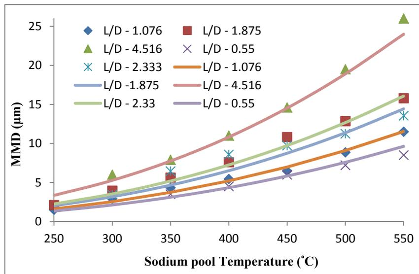
**Fig. 7.** Variation of MMD (Expt. and Theo.) with sodium pool temperature for various L/D ratio.
