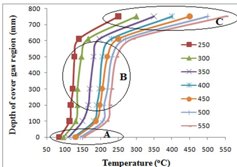
Fig. 4. The variation of temperature in cover gas region with cover gas height for various pool temperatures for TP-3.
