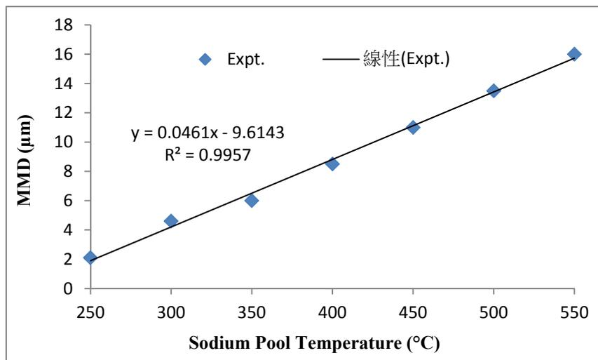
Fig. 5. MMD of sodium aerosol in the middle region of the cover gas of TP-3 for various pool temperatures.
