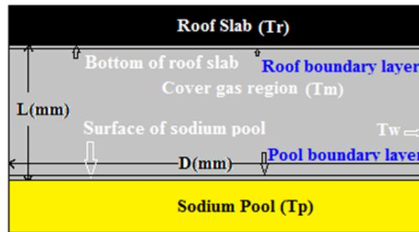
**Fig. 1.** Schematic diagramme of cover gas region, sodium pool and roof top.
