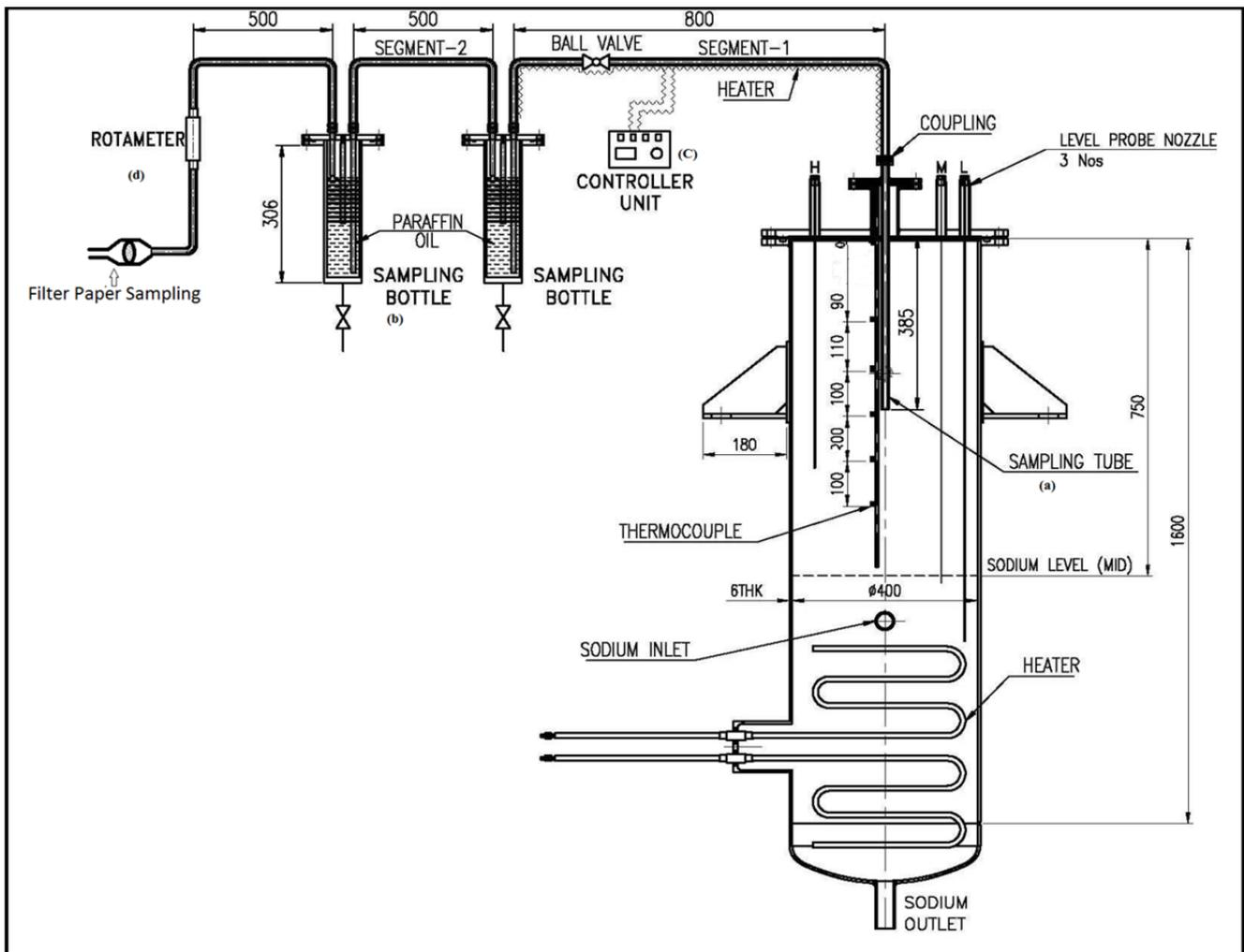
Fig. 2. A schematic diagram of sodium aerosol sampling system installed in TP-3 of SILVERINA loop.
