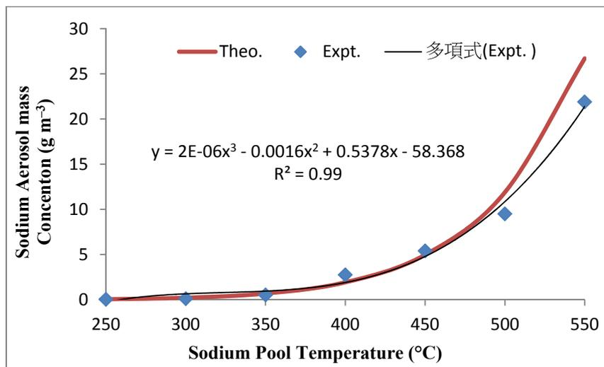
Fig. 6. Sodium aerosol mass concentration (simulated and expt.) in the middle region of cover gas of TP-3 for various pool temperatures.
