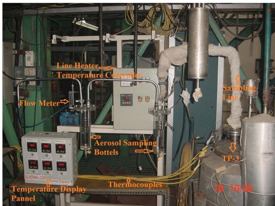
Fig. 3. A photograph of the aerosol sampling system along with temperature measurement system.
