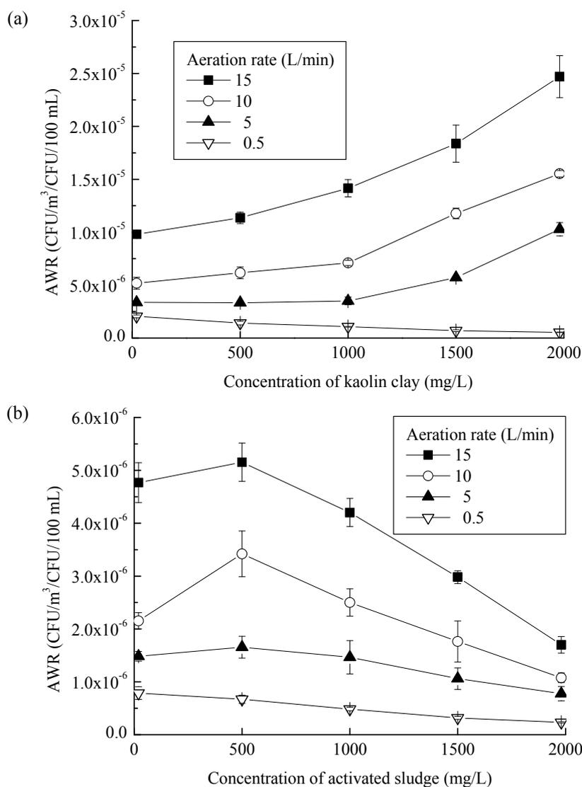
**Fig. 2.** Air/water ratios (AWR) when (a) kaolin clay and (b) activated sludge serve as the suspended solid. Each error bar represents one standard deviation on mean of at least three tests.
