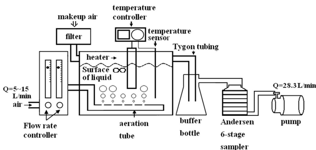
**Fig. 1.** Schematic drawing of the experimental and measurement systems. Cells of *E. coli* and test sludge were introduced into the aeration tester before each test.
