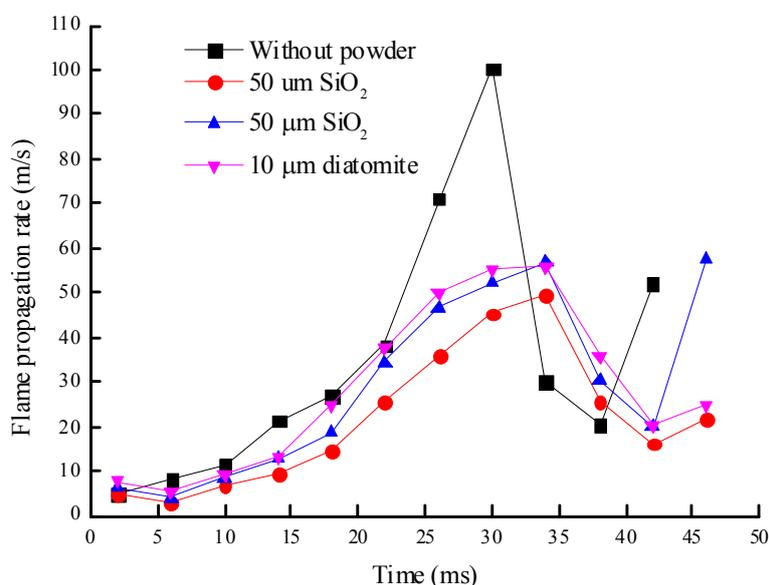
**Fig. 4.** Influence of  $11.28 \text{ mg L}^{-1}$  added amount of powder aerosol on flame propagation rate of gas explosion.
