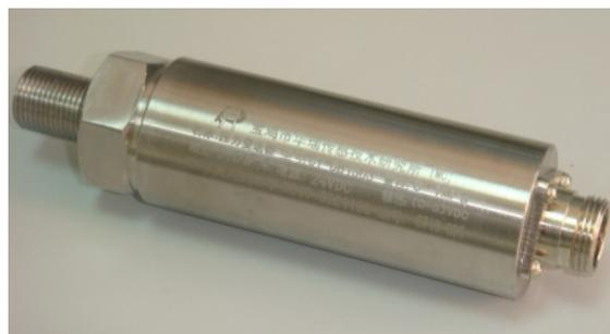
(b) The CY-DB1303 pressure sensor of experimental system (Range: 0–1 MPa, Response time: 1 ms, Accuracy: 0.3% F.S)
