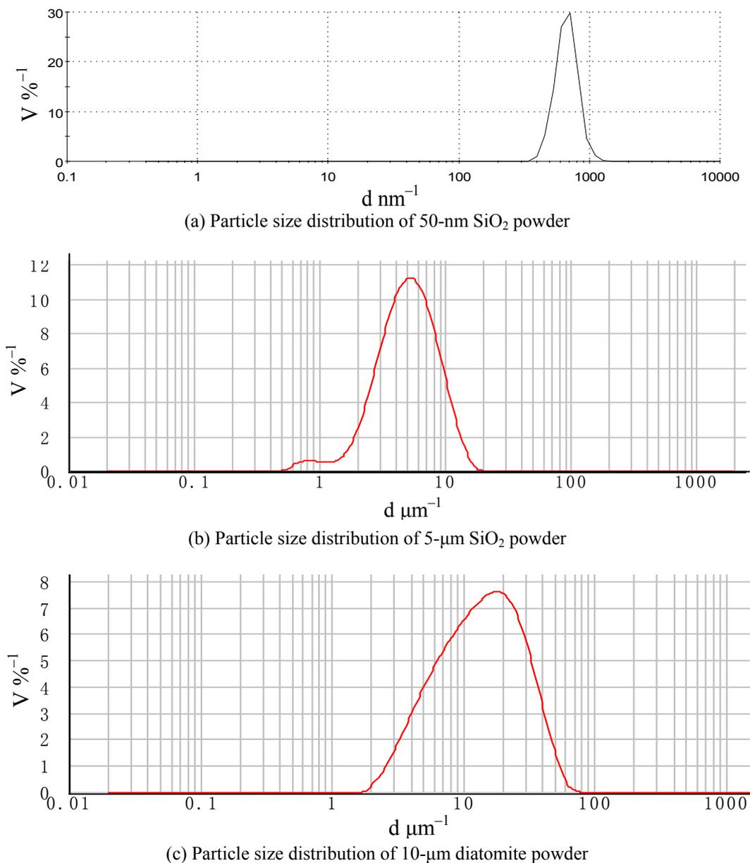
**Fig. 1.** Particle size distribution of SiO<sub>2</sub> powder aerosol and powder aerosol.
