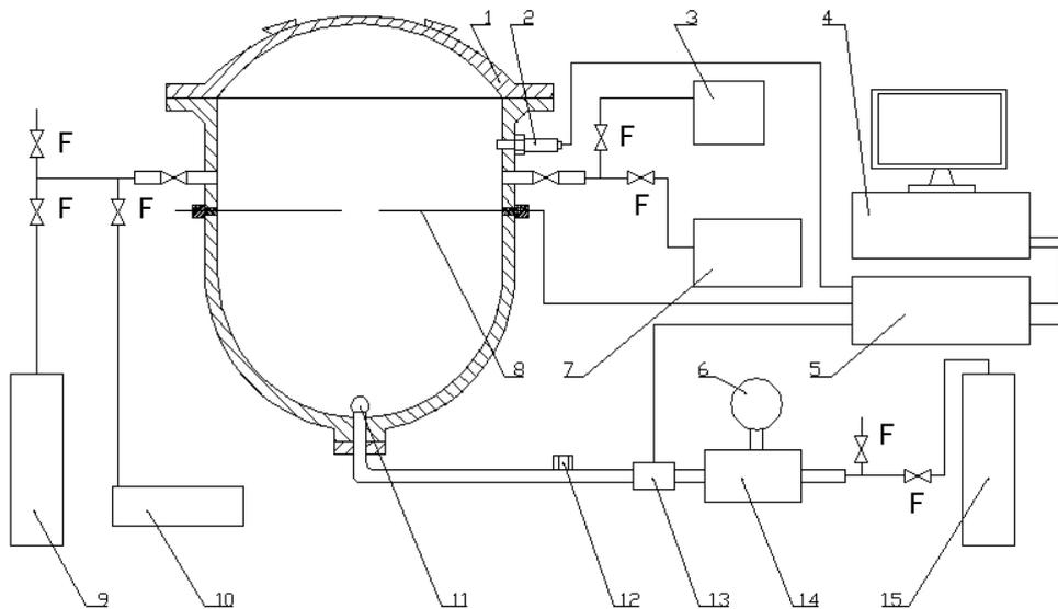
(a) 1-Explosion reactor; 2-Pressure sensor; 3-Digital pressure gauge; 4-Computer; 5-Controller; 6-Pressure gauge; 7-Vacuum pump; 8-Ignition source; 9-Methane cylinder; 10-Air compressor; 11-Powder aerosol injector; 12-Powder aerosol cylinder; 13-Solenoid valve; 14-High pressure air tank; 15-Compressed air cylinder
