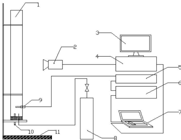
1-Quartz tube; 2-High-speed camera; 3-Displayer; 4-Data acquisition unit; 5-Igniter; 6-Controller; 7-Computer; 8-Gas cylinder; 9-Spark plug; 10-Suppressant spray entrance; 11-Fixed support
