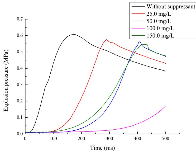
**Fig. 5.** Effect of nano-scale SiO<sub>2</sub> powder aerosol on 7% gas explosion pressure.
