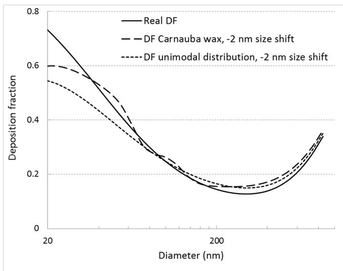
**Figure S6.** Illustrates the error caused by a negative diameter size shift of 2 nm of the exhaled particles. The solid line corresponds to the true DF, dashed line to the resulting measured DF in the case of a size shift in the carnauba wax particle size distribution, and the dotted line corresponds to the measured DF in the case of a size shift of a fictive distribution with a geometrical mean diameter of 100 nm (geometrical standard deviation 1.7).
