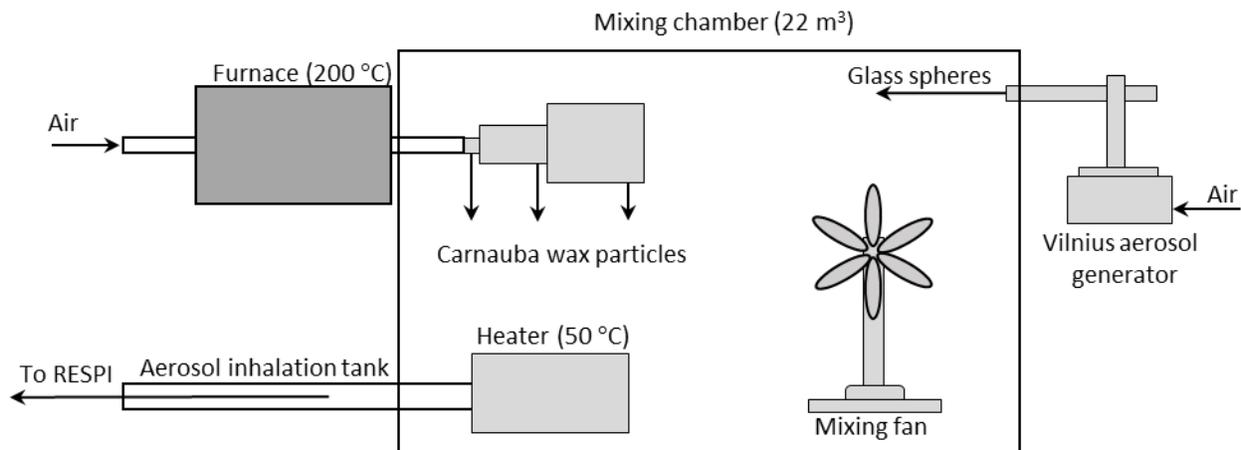
**Figure S4.** Schematic picture of the aerosol generation.
