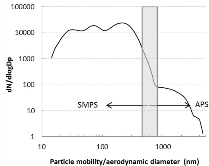
**Figure S5.** The graph shows a typical size distribution of the aerosol used in the study. The grey area shows the cut-point between the size region of the SMPS and APS.
