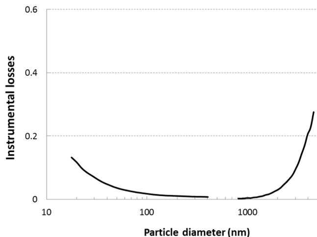
Figure S2. Instrumental particle losses at 6 L/min.
