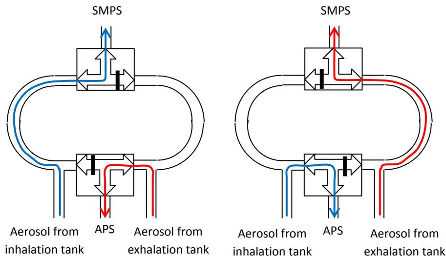
**Figure S1.** Schematic picture of the air flows through the 3-way valves in the RESPI<sub>2</sub>.
