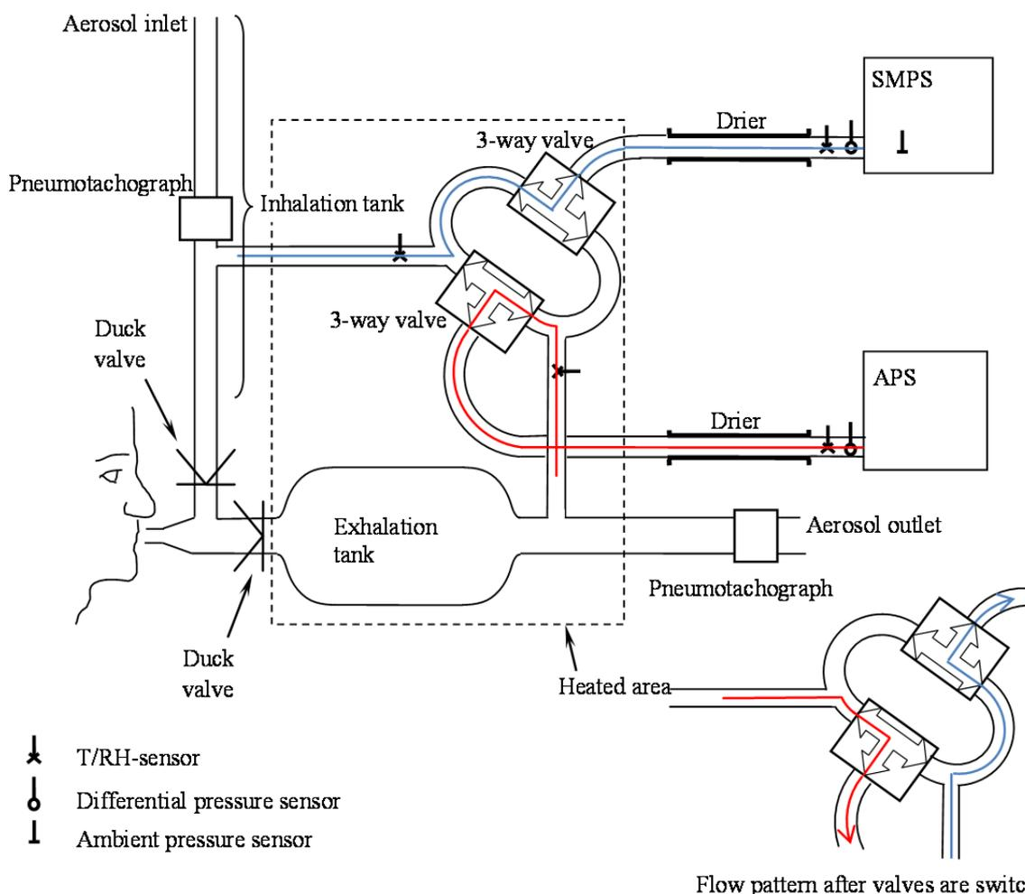
**Fig. 1.** A schematic picture of the RESPI<sub>2</sub> set-up. Arrows indicate the flows, where the red arrow represents the APS flow and the blue arrow the SMPS flow. The flows after switching the valves are shown in the lower right corner of the main figure.
