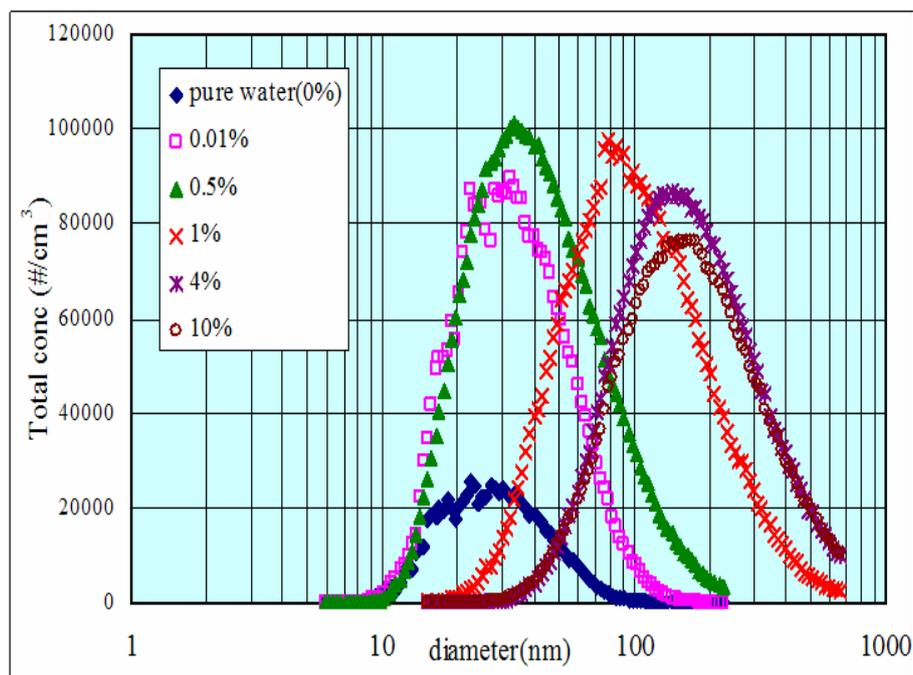
**Fig. 2.** Size distribution of polydisperse particles produced from NaCl<sub>(aq)</sub>.
