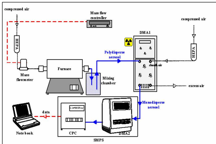
**Fig. 1B.** Generation system of oleic acid nanodroplets.
