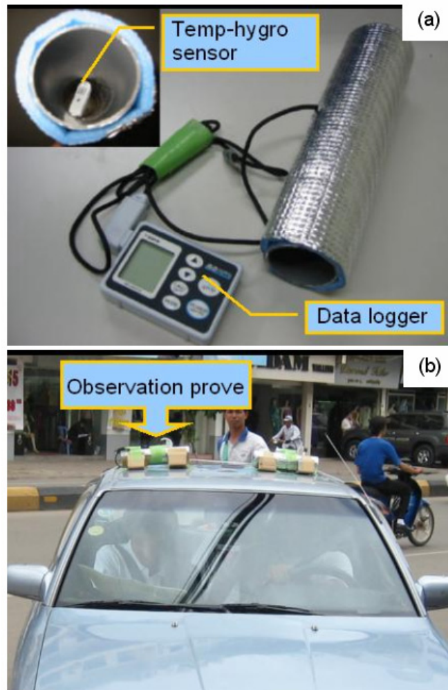
Fig. 2. (a) Observation probe (a temp-hygro sensor with data logger), (b) observation probes installed on the roof top of a car.
