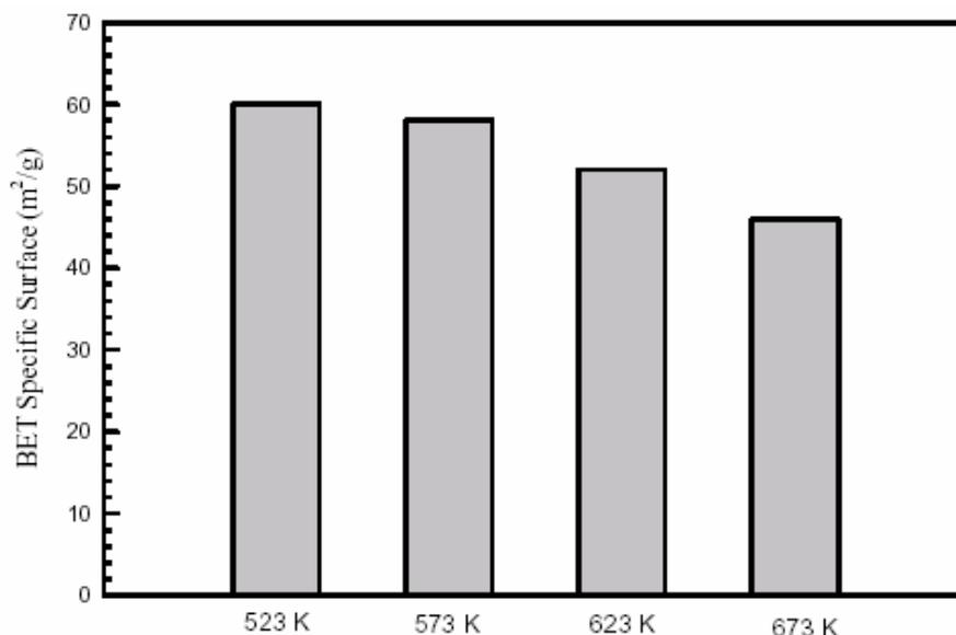
**Fig. 3.** Effect of reaction temperature with changes of specific surface area on the bimetallic CuO/CeO<sub>2</sub> nanoparticle catalyst for the conversion of NH<sub>3</sub>. Test conditions: 800 ppm NH<sub>3</sub> in He, O<sub>2</sub> = 4%, RH = 18%, GHSV = 92000 mL/h-g.
