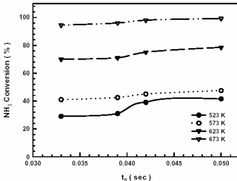
**Fig. 2.** Effect of empty bed residence time (EBRT) on the bimetallic CuO/CeO<sub>2</sub> nanoparticle catalyst for the conversion of NH<sub>3</sub> as function of temperature. Test conditions: 800 ppm NH<sub>3</sub> in He, O<sub>2</sub> = 4%, GHSV = 92000 mL/h-g.
