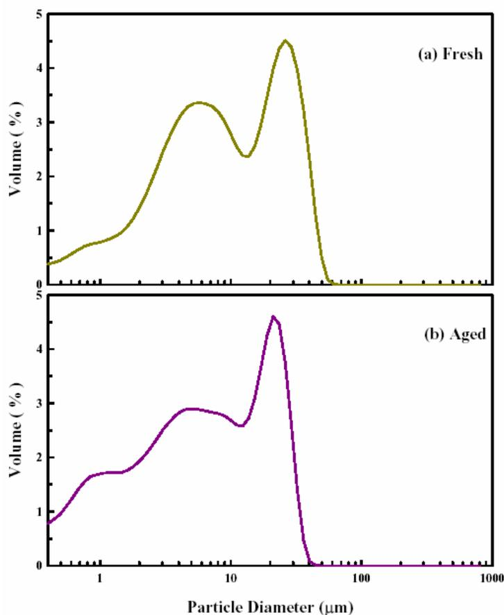
**Fig. 6.** Changes in particle sizes distribution of the bimetallic CuO/CeO<sub>2</sub> nanoparticle catalyst. (a) fresh, (b) after activity test. Test conditions: 800 ppm NH<sub>3</sub> in He, O<sub>2</sub> = 4%, GHSV = 92000 mL/h-g.
