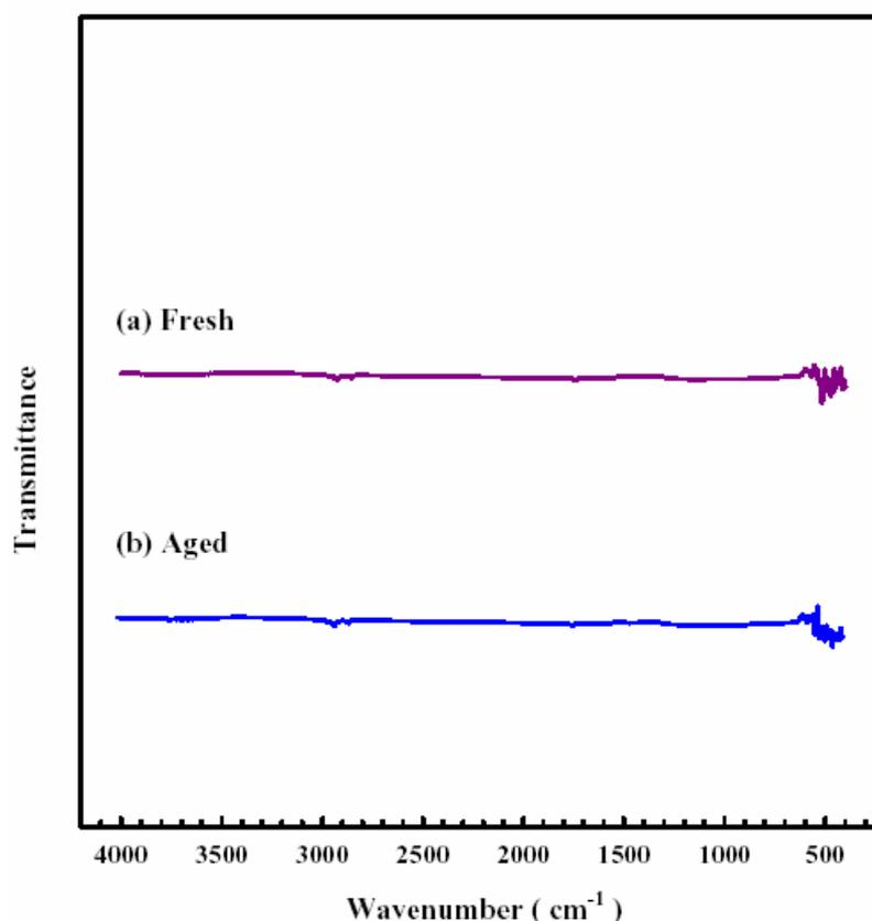
**Fig. 5.** ATR-FTIR pattern of the bimetallic CuO/CeO<sub>2</sub> nanoparticle catalyst. (a) fresh, (b) after activity test. Test conditions: 800 ppm NH<sub>3</sub> in He, O<sub>2</sub> = 4%, GHSV = 92000 mL/h-g.
