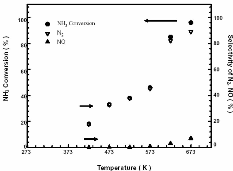
**Fig. 4.** Relationship of the ammonia conversion, N<sub>2</sub> yield, and NO yield at various temperatures over the bimetallic CuO/CeO<sub>2</sub> nanoparticle catalyst. Test conditions: 800 ppm NH<sub>3</sub> in He, O<sub>2</sub> = 4%, RH = 12%, Temp = 423-673K, GHSV = 92000 mL/h-g.
