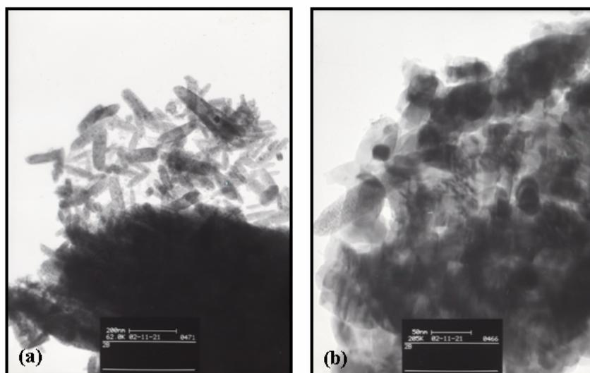
**Fig. 7.** TEM photograph of (a) fresh and (b) after activity test bimetallic CuO/CeO<sub>2</sub> nanoparticle catalyst. Test conditions: 800 ppm NH<sub>3</sub> in He, O<sub>2</sub> = 4%, GHSV = 92000 mL/h-g.
