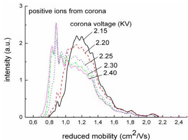
**Fig. 7.** Mobility spectra of positive air ions as a function of the corona voltage.
