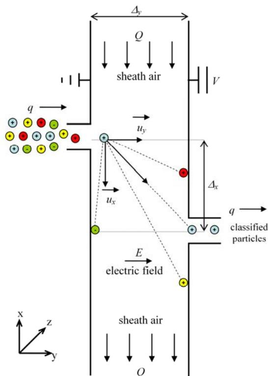
Fig. 1. Sketch of a parallel-plate DMA.
