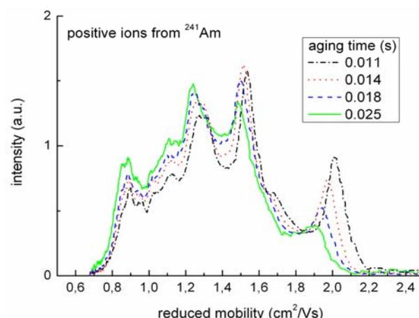
Fig. 4. Evolution of the mobility distribution of positive air ions generated by  $^{241}\text{Am}$  during the early stages of aging.
