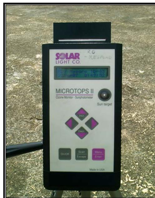
**Fig. 1.** Tripod mounted MICROTOPS II under action.
